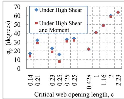
Figure 5:  $\phi_p$  values of the first plastic hinge
