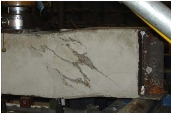
Figure 7. USFB No.1 at Failure point.
