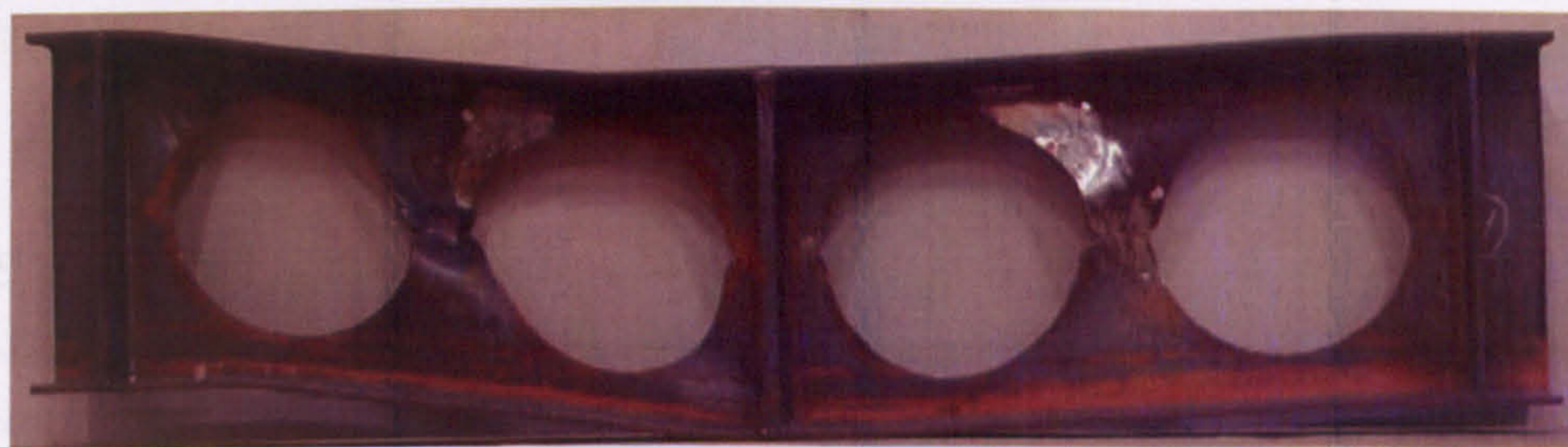
Figure 5.60(a): Web-post buckling shape of the Specimen A-2
