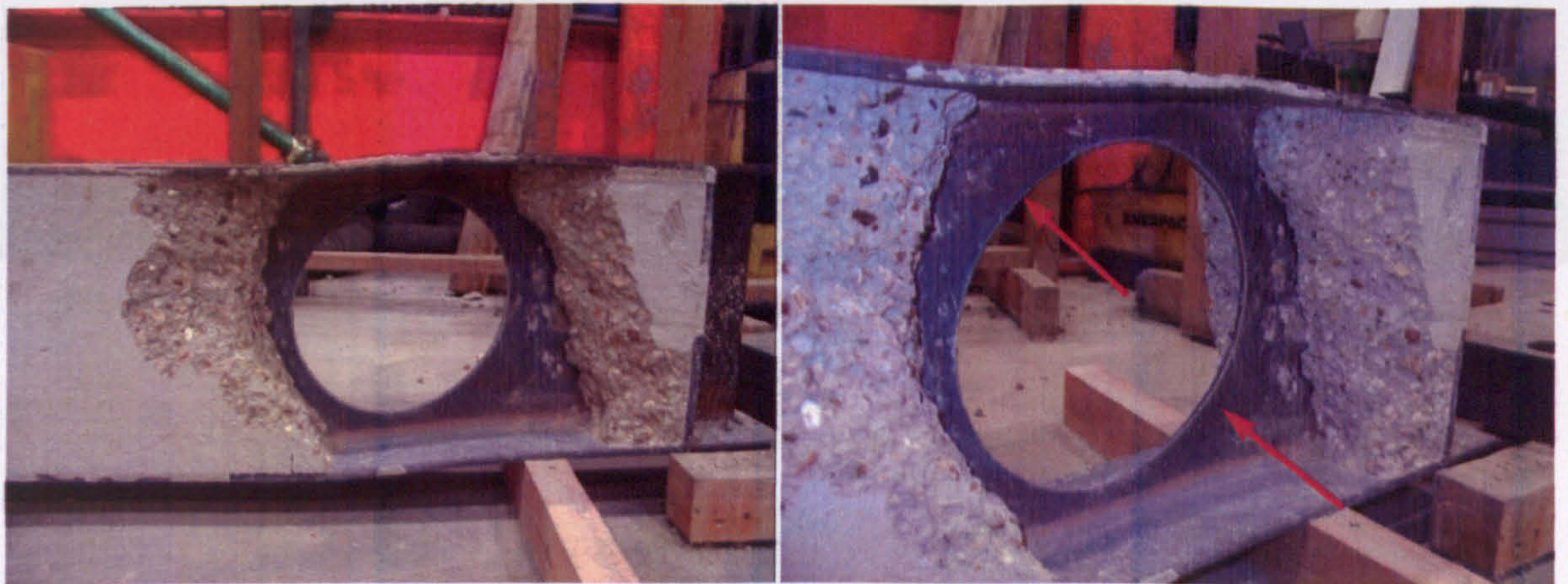
Figure 6.16: USFB No.2 after concrete is removed
