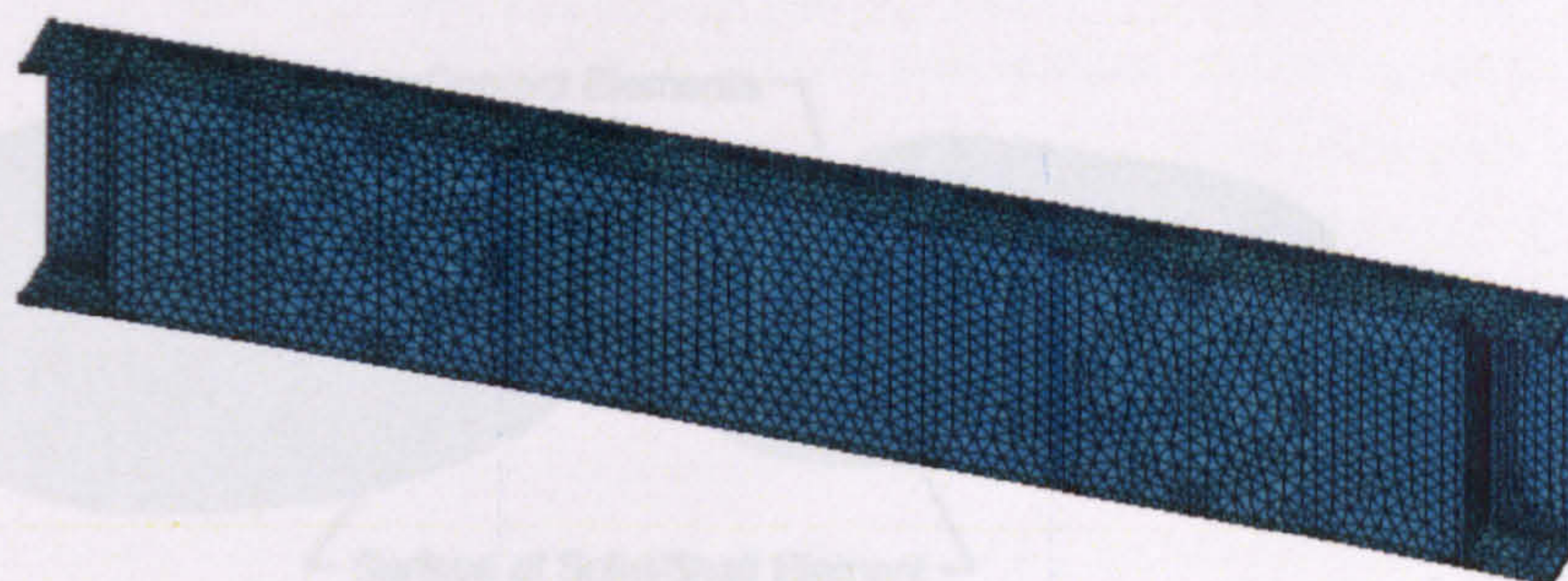
Figure 6.19: Symmetric FE model of the USRB
