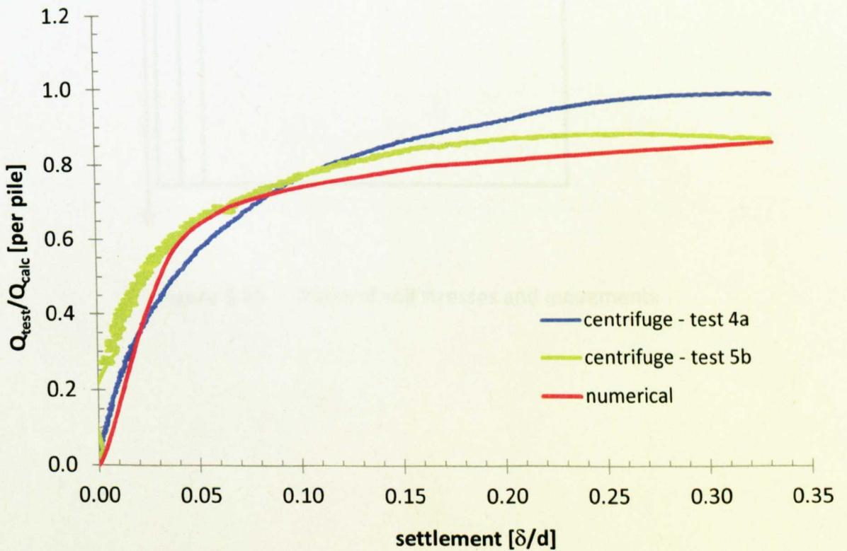
Figure 8.14  $Q_{test}/Q_{calc}$  vs settlement comparison: GS25\_2.00
