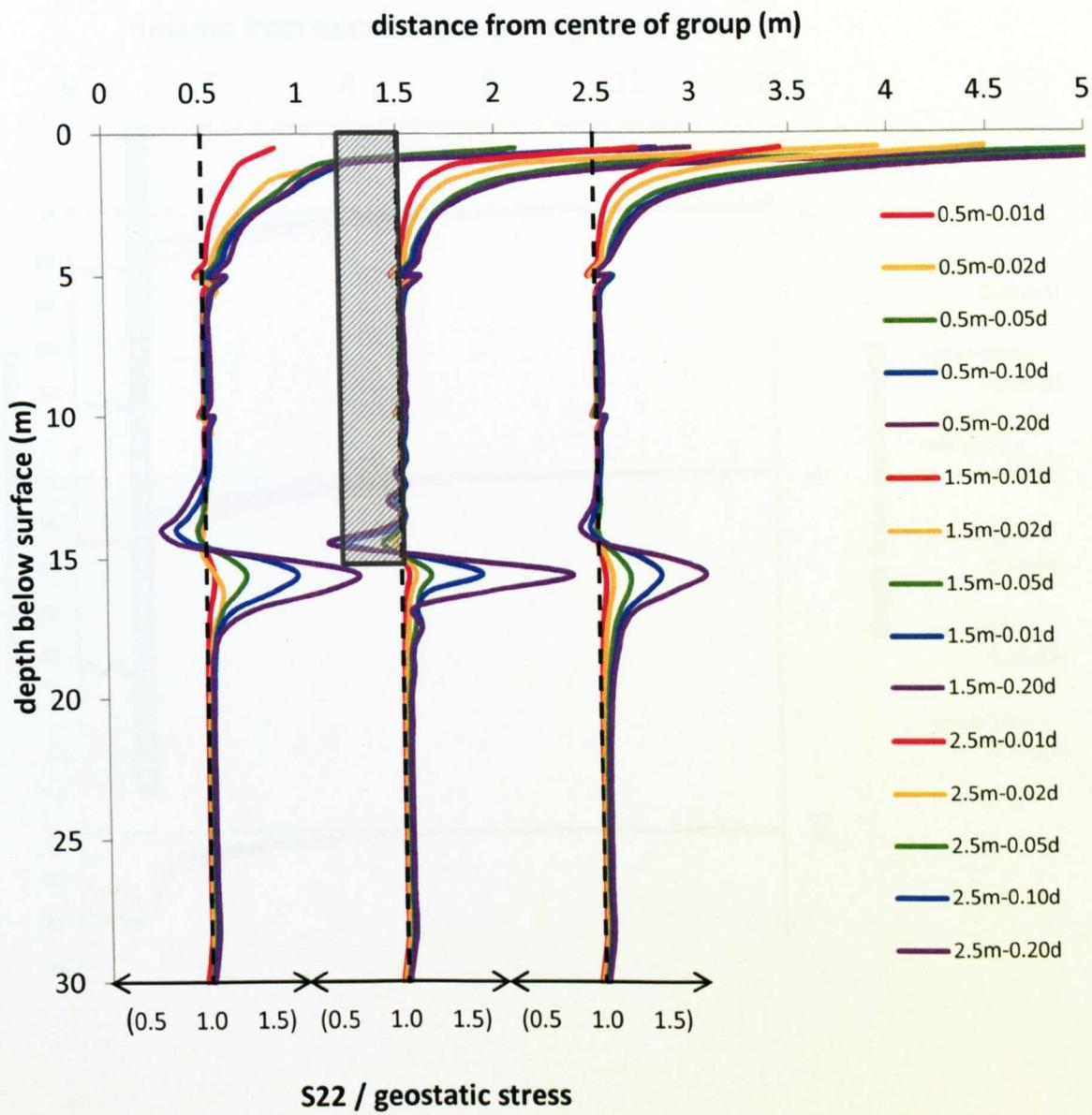
Figure 8.21 Horizontal stress change with settlement ( $s_{pB}$ )
