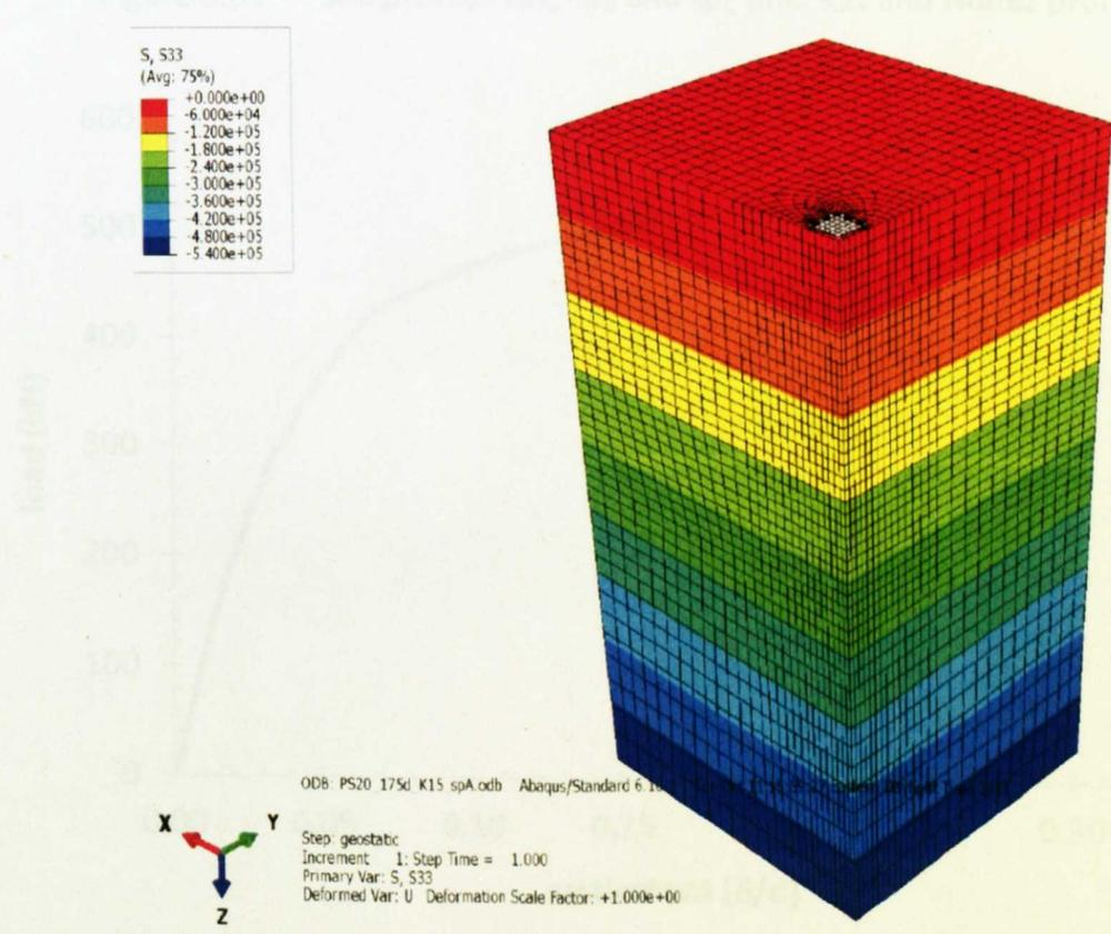
Figure 7.02 Geostatic stress distribution
