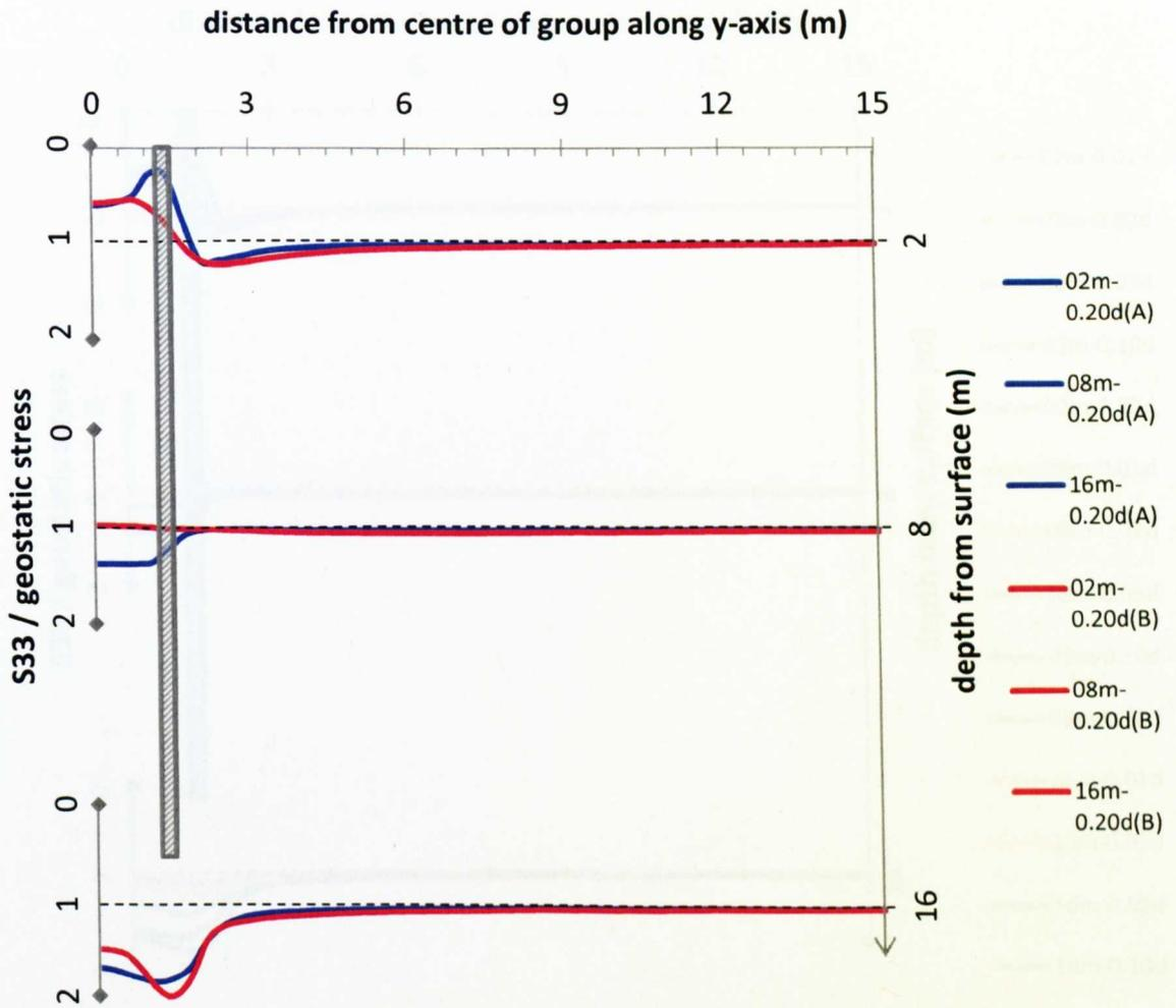
Figure 8.17 Vertical stress change with saturation (sp)
