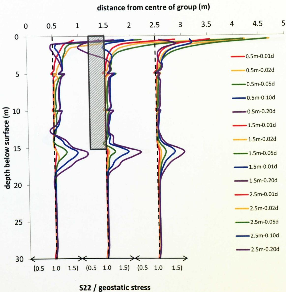
Figure 8.20 Horizontal stress change with settlement ( $sp_A$ )
