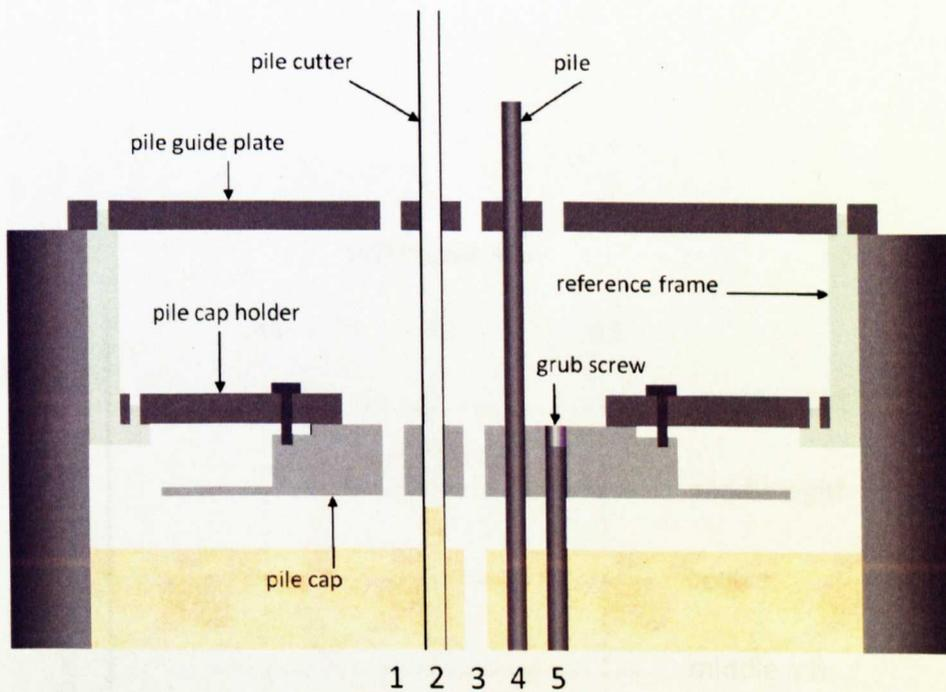
1. Apparatus in place pre pile installation
