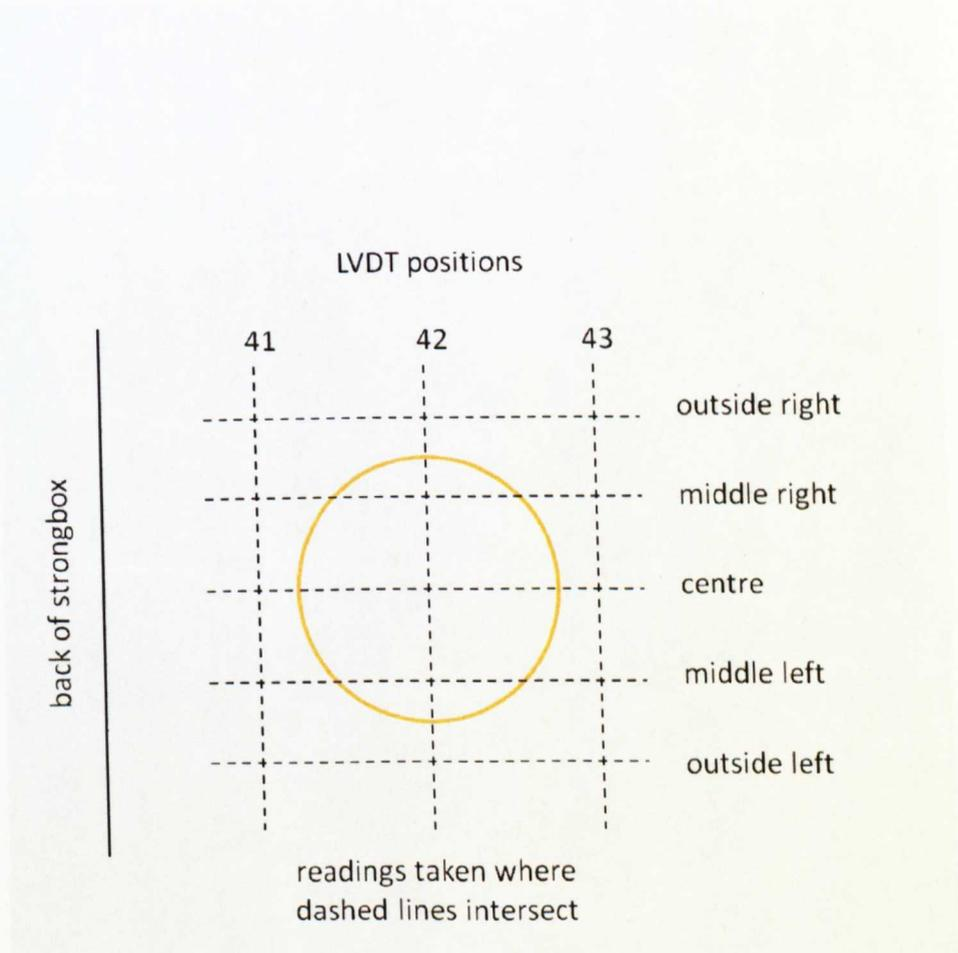
Figure 5.13 Central soil settlement data recording points
