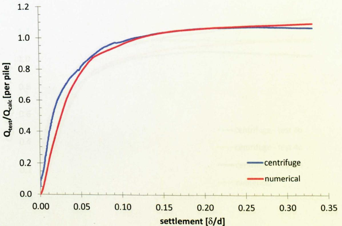
Figure 8.06  $Q_{test}/Q_{calc}$  vs settlement comparison: PC14\_1.75
