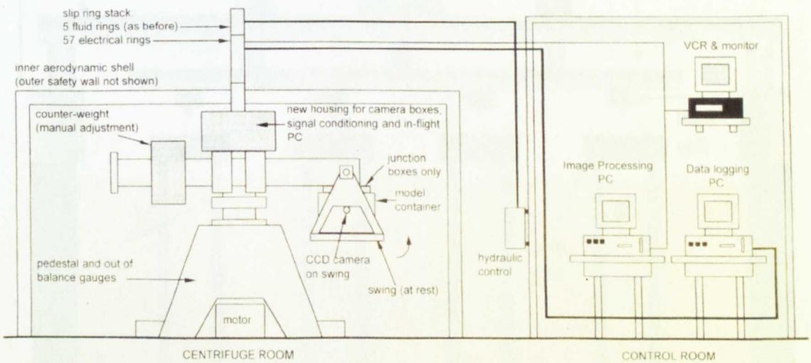
Figure 4.05 Schematic diagram of the centrifuge (Grant, 1998)
