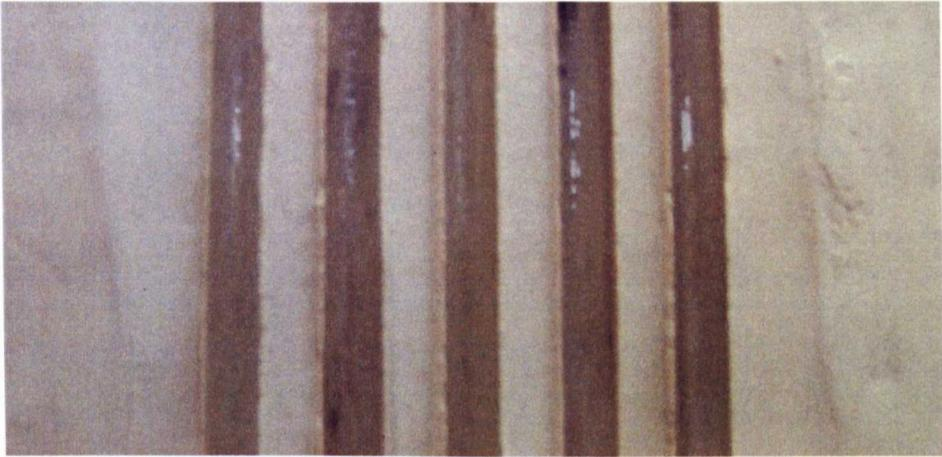
Figure 5.22 Silicone oil on clay bore (test 1c)
