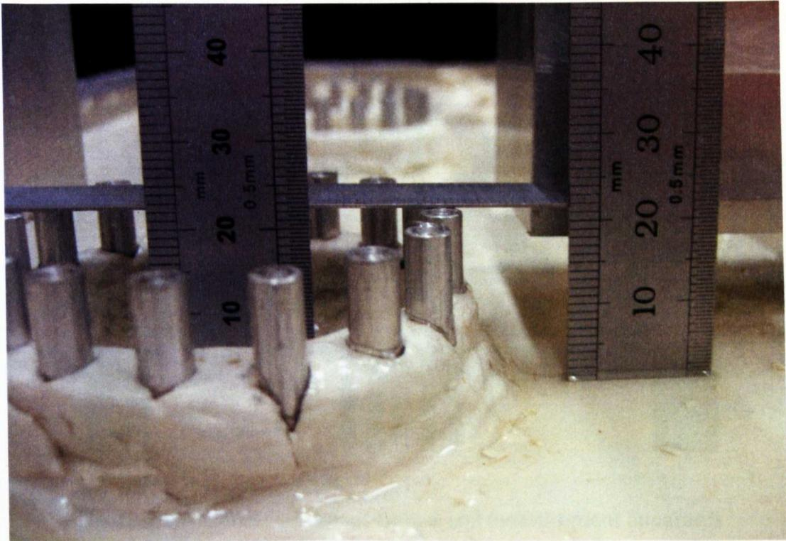
Figure 6.18a Early measurement of 'block effect' failure (test 2b)
