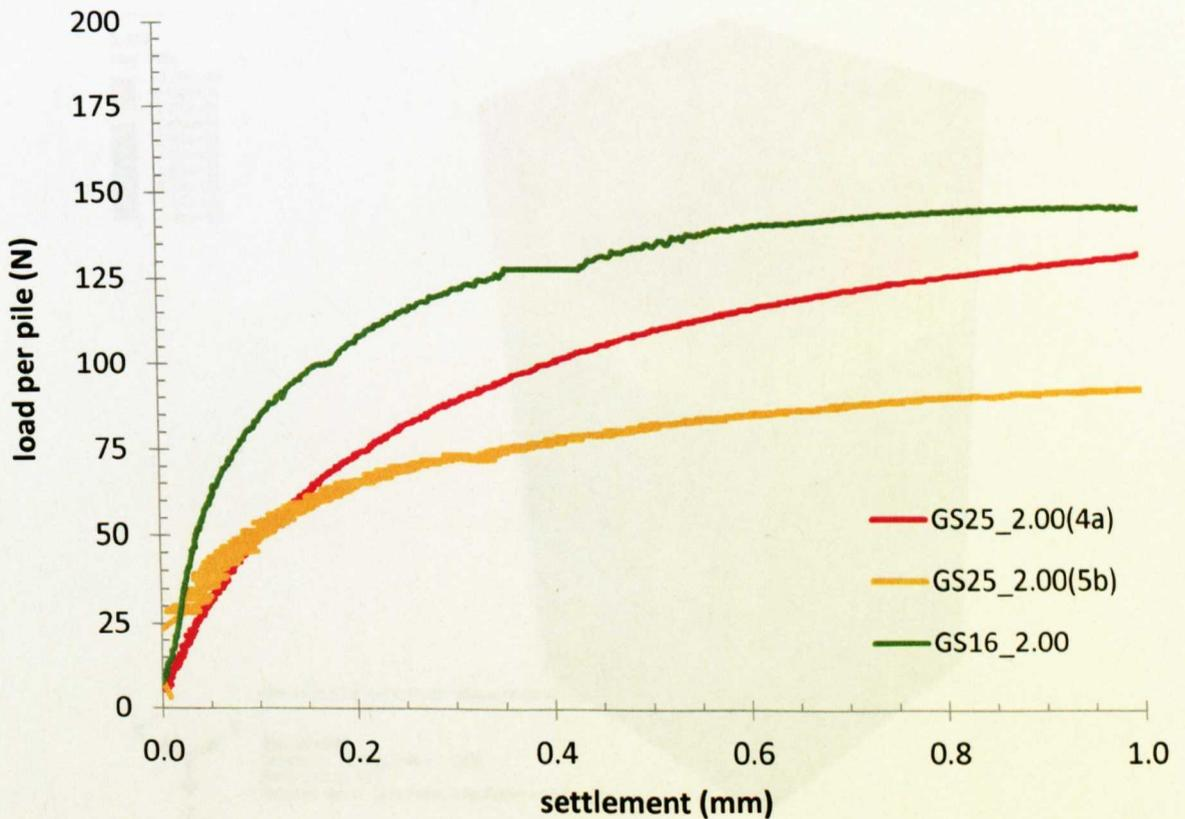
Figure 6.35 Load vs settlement (0 – 1 mm): grid groups
