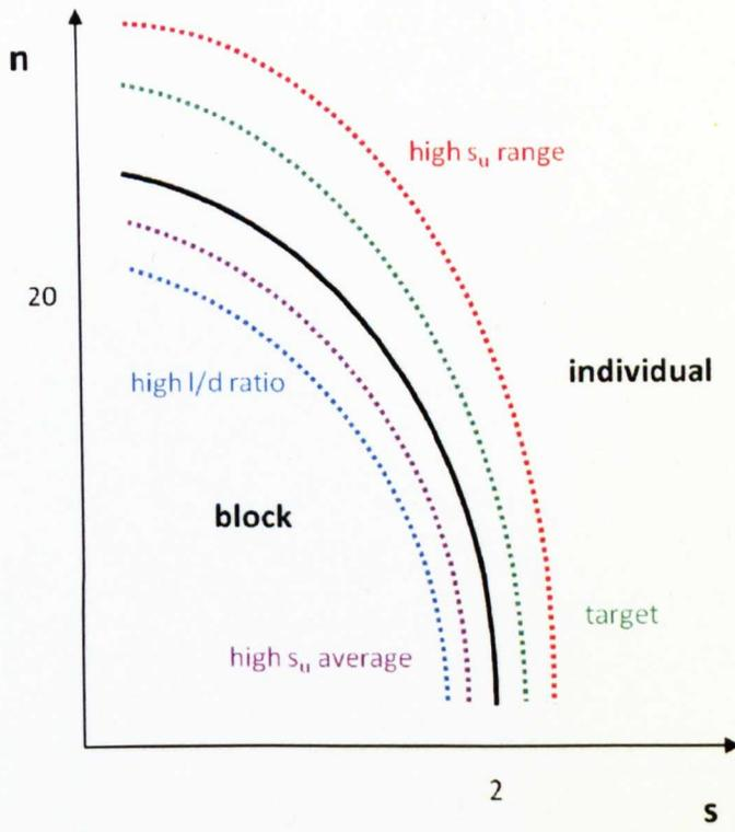
Figure 10.01 General trend showing influences on failure mechanism
