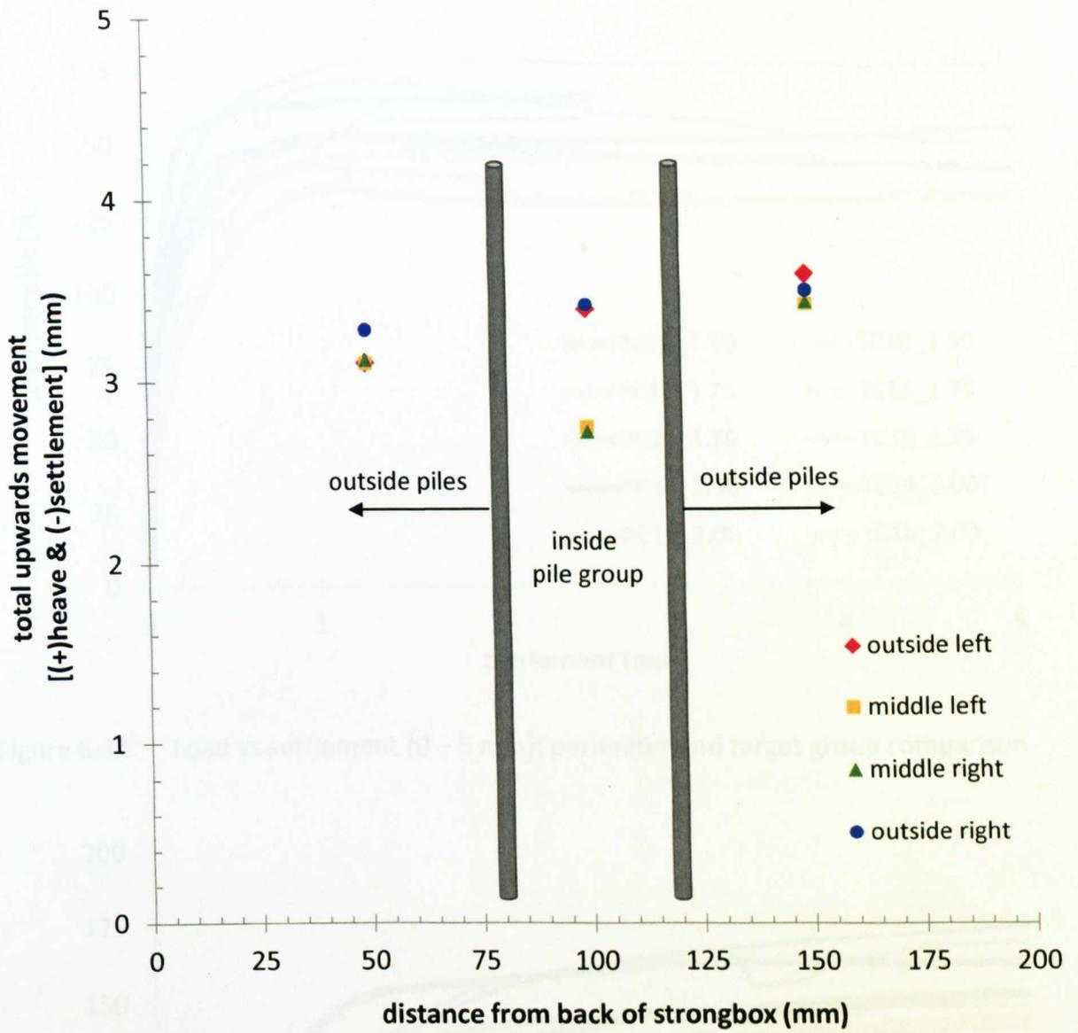
Figure 6.31 Central soil settlement measurements of TC14\_2.00
