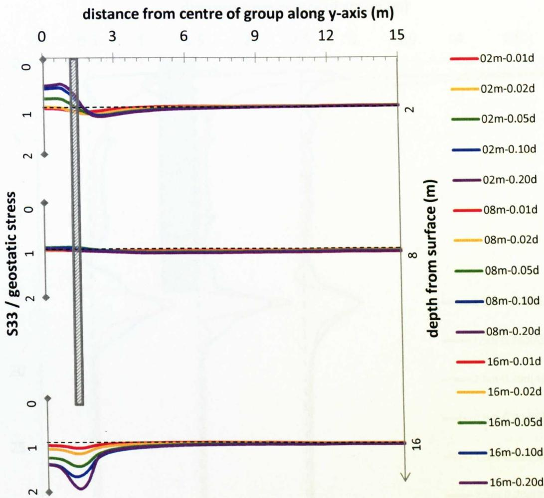
Figure 8.18 Vertical stress change with settlement ( $sp_B$ )
