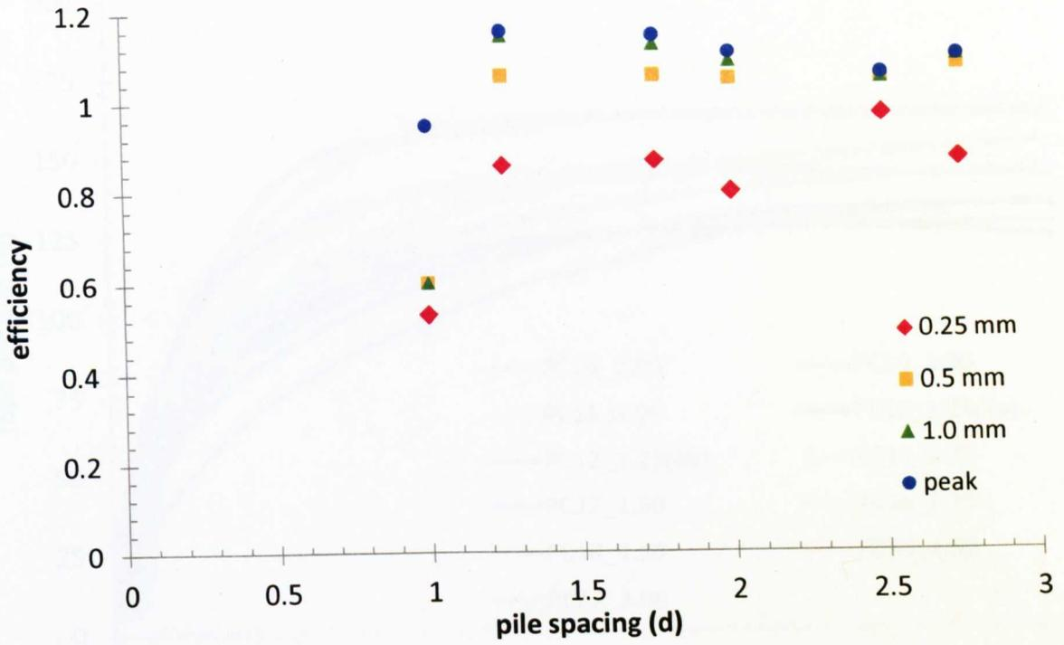
Figure 6.10 Efficiency vs pile spacing: linear groups
