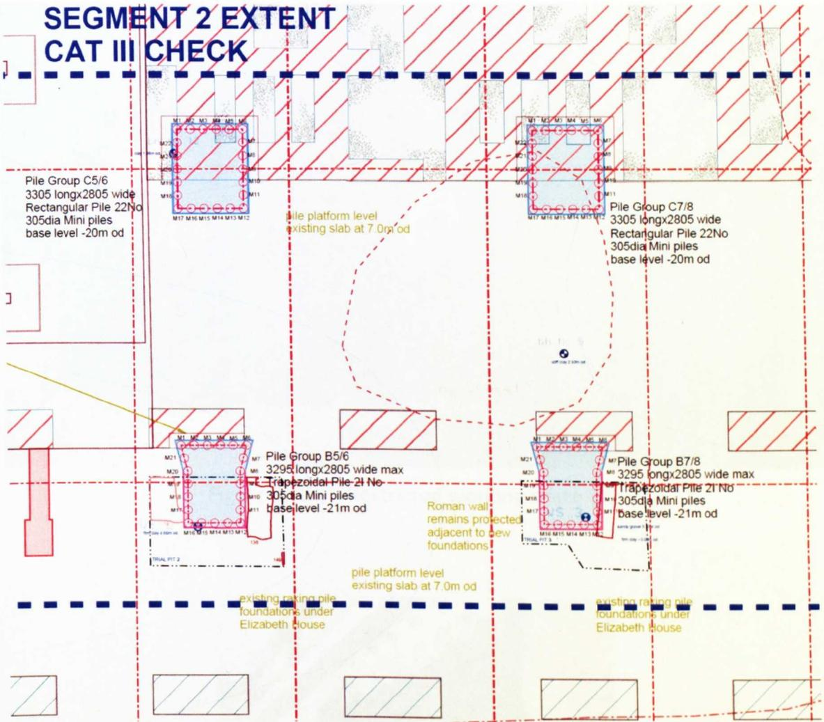
Figure 3.01b Perimeter group pile layout drawing (east)
