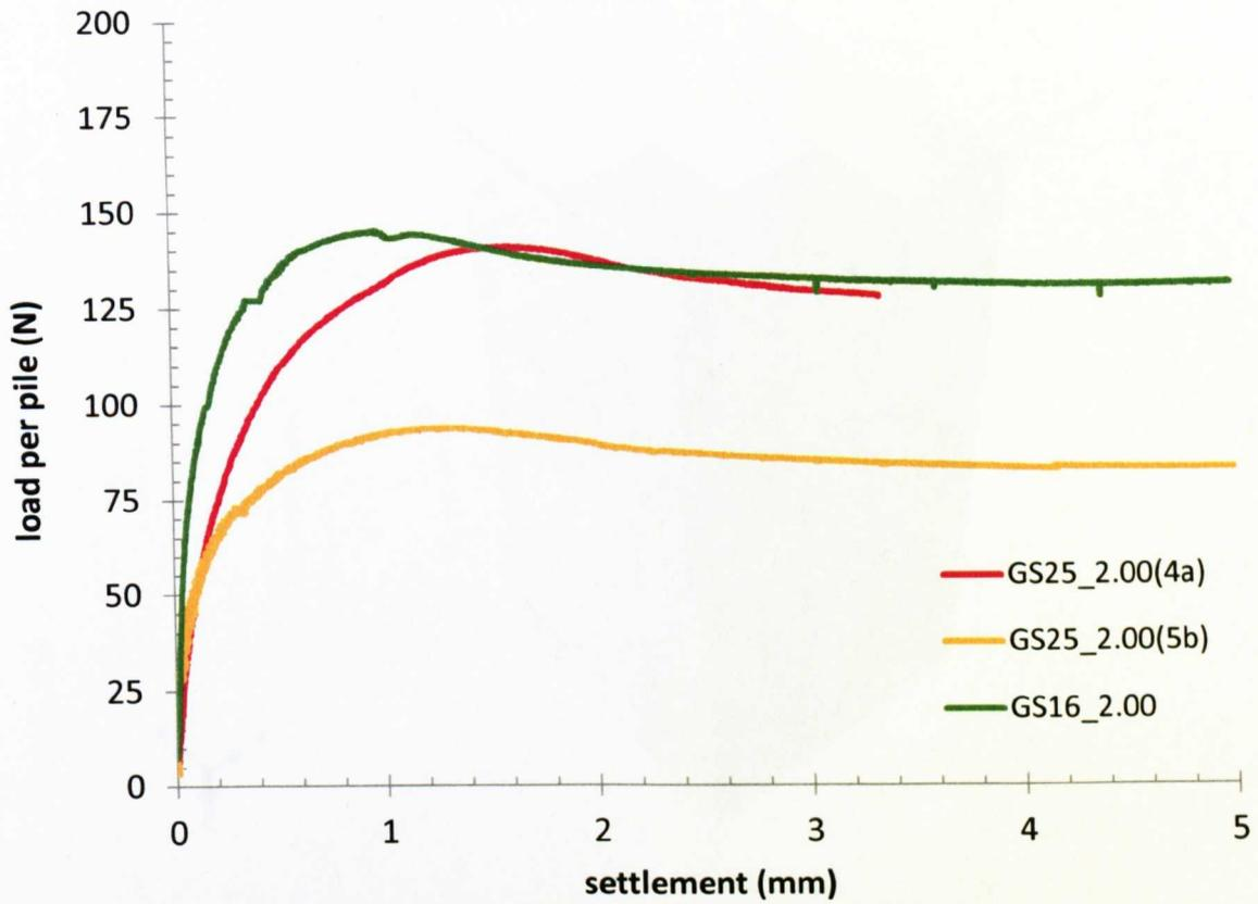
Figure 6.34 Load vs settlement (0 – 5 mm): grid groups
