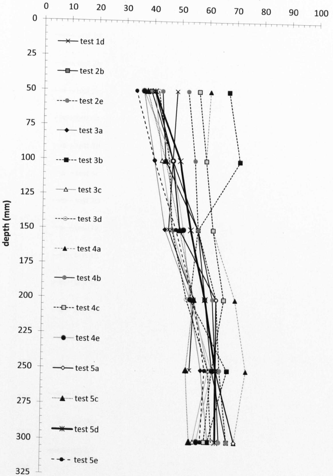
Figure 6.01 Undrained shear strength profile from hand vane tests
