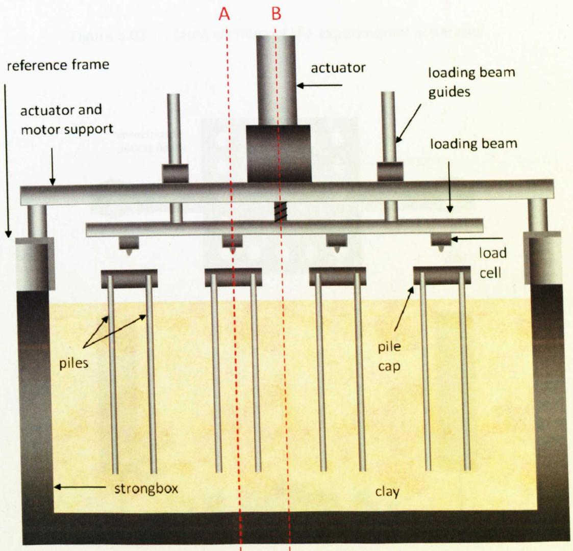
Figure 5.02 Long section of the experimental apparatus
