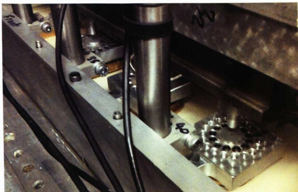
Figure 5.18 Loading beam and load cell in place above loading point and pile cap
