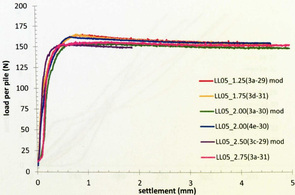
Figure 6.07 Load vs settlement (0 – 5 mm): linear groups
