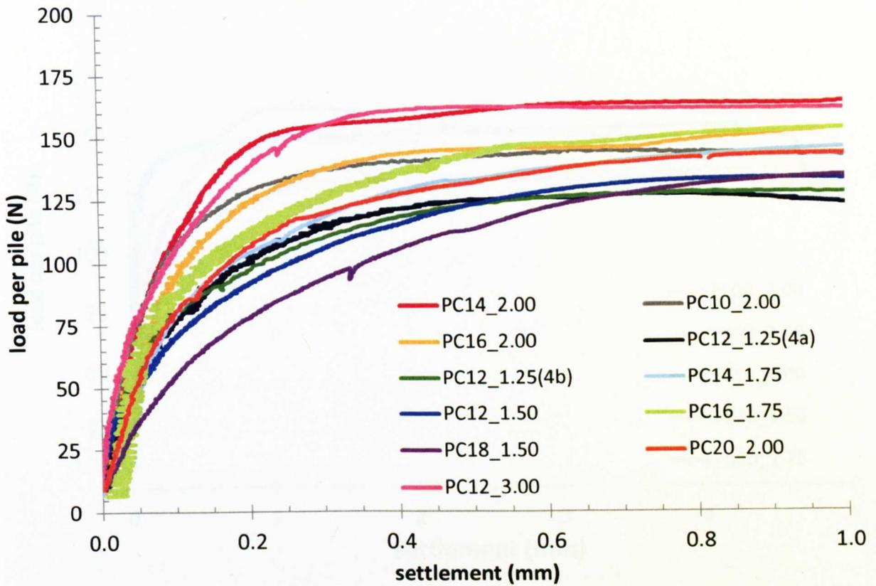
Figure 6.12 Load vs settlement (0 – 1 mm): perimeter groups (circular)
