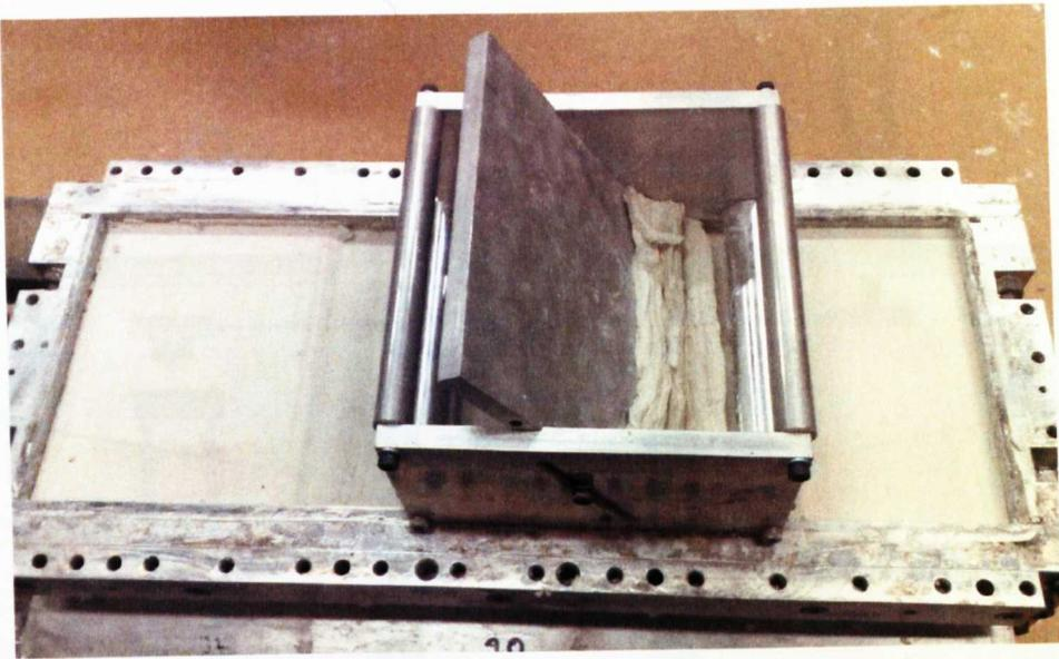
Figure 5.01 Cutting the clay surface to the correct height
