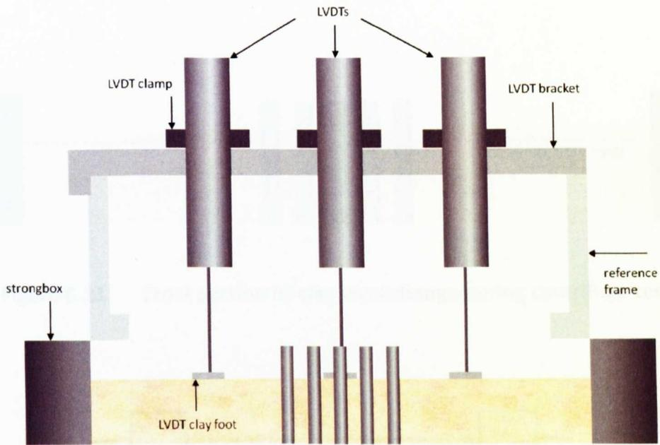
Figure 6.19 Cross section of central soil measurement apparatus
