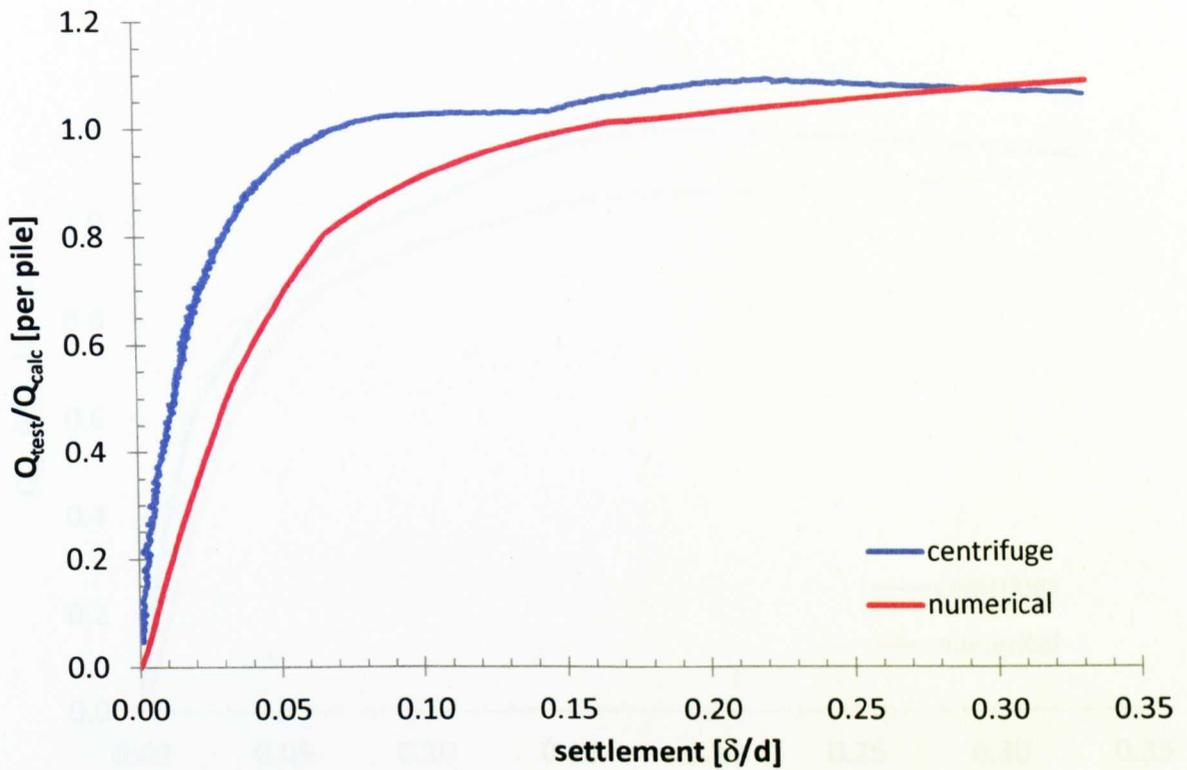
Figure 8.05  $Q_{test}/Q_{calc}$  vs settlement comparison: PS16\_2.00 (numerical) and PC16\_2.00 (centrifuge)
