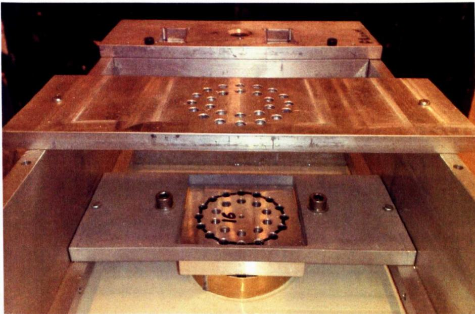
Figure 5.10 Pile installation set-up (test 3b)
