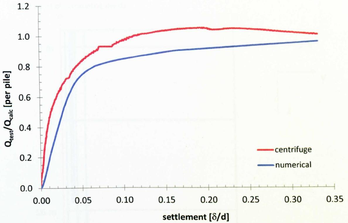
Figure 8.13  $Q_{test}/Q_{calc}$  vs settlement comparison: GS16\_2.00
