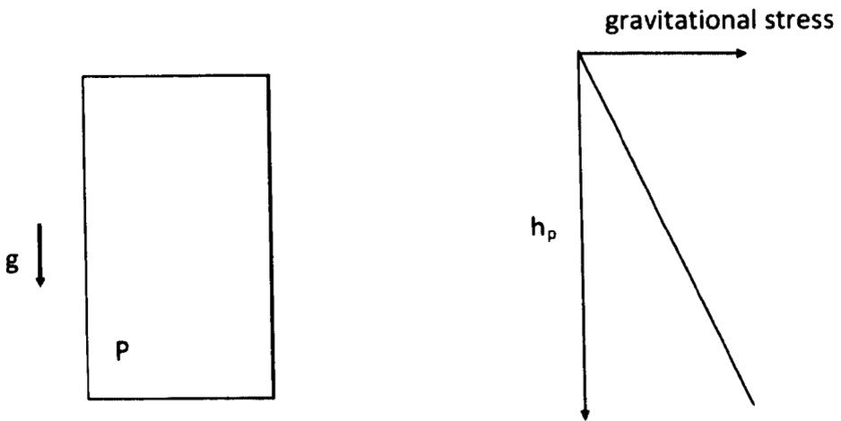
Figure 4.01b Gravitational stress in the prototype (after Taylor, 1995)
