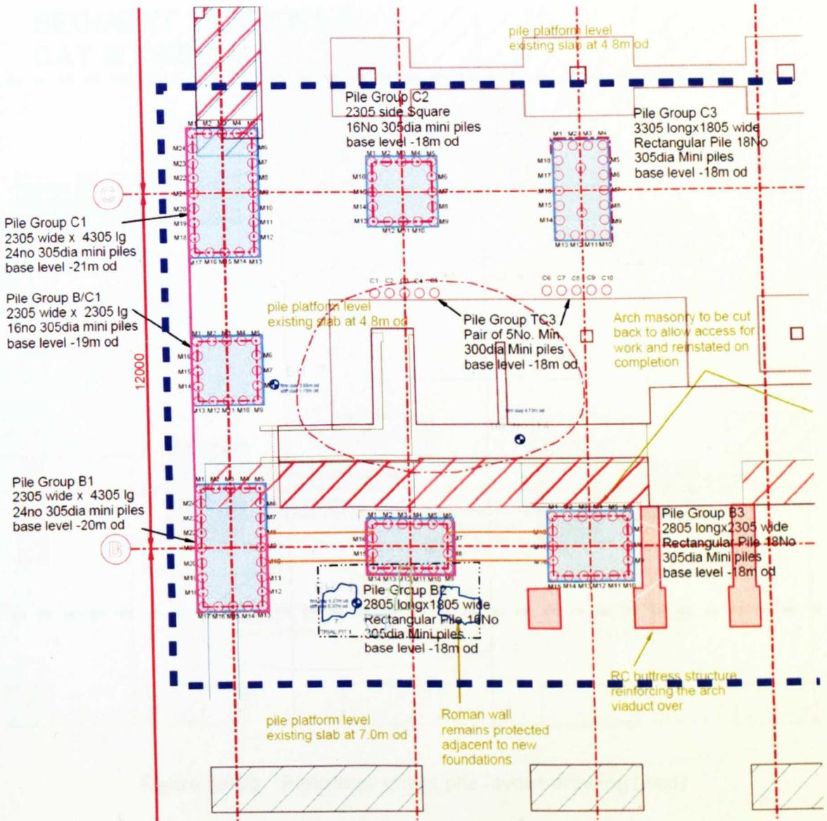
Figure 3.01a Perimeter group pile layout drawing (west)
