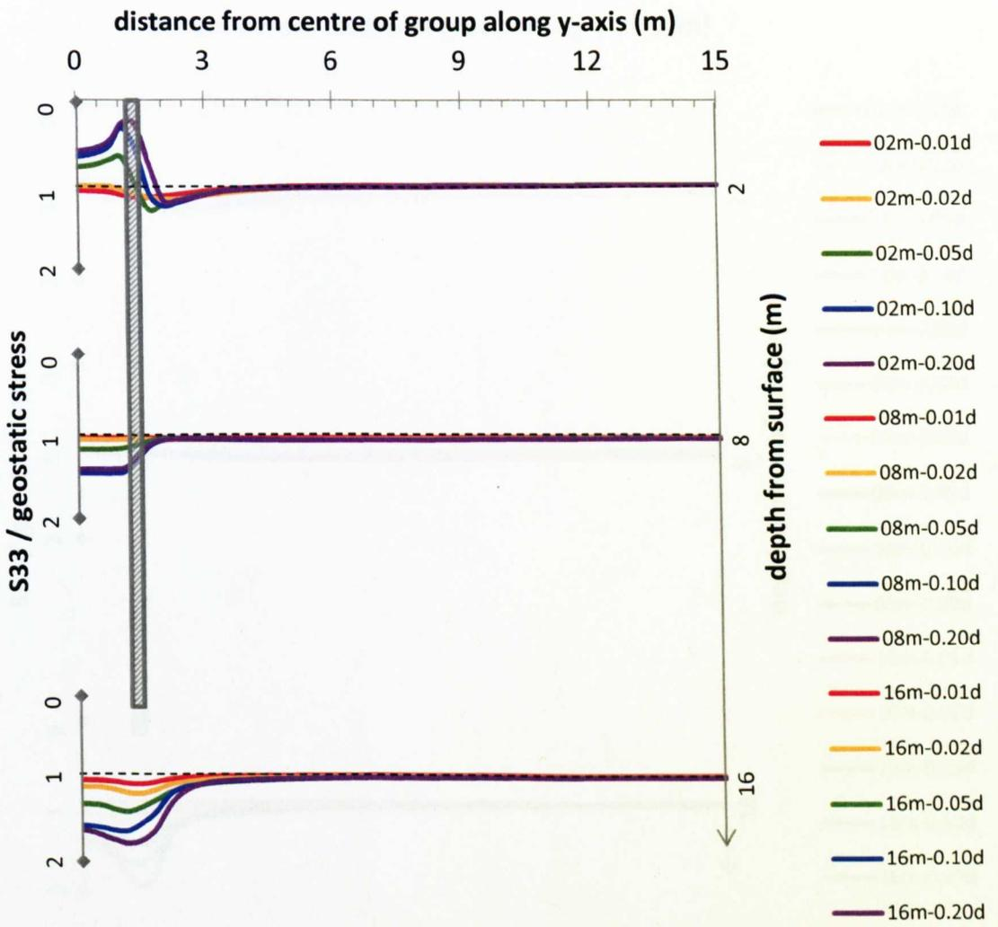
Figure 8.17 Vertical stress change with settlement ( $s_{pA}$ )
