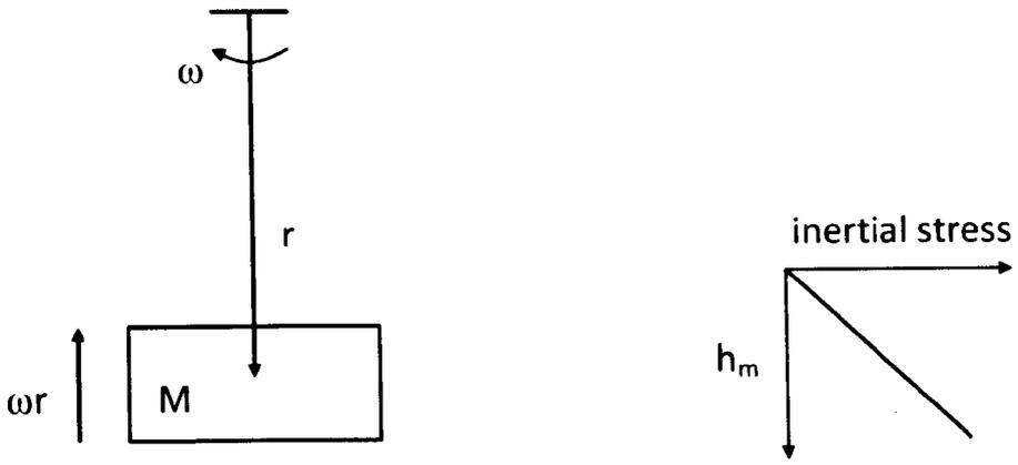
Figure 4.01a Inertial stress in the model (after Taylor, 1995)
