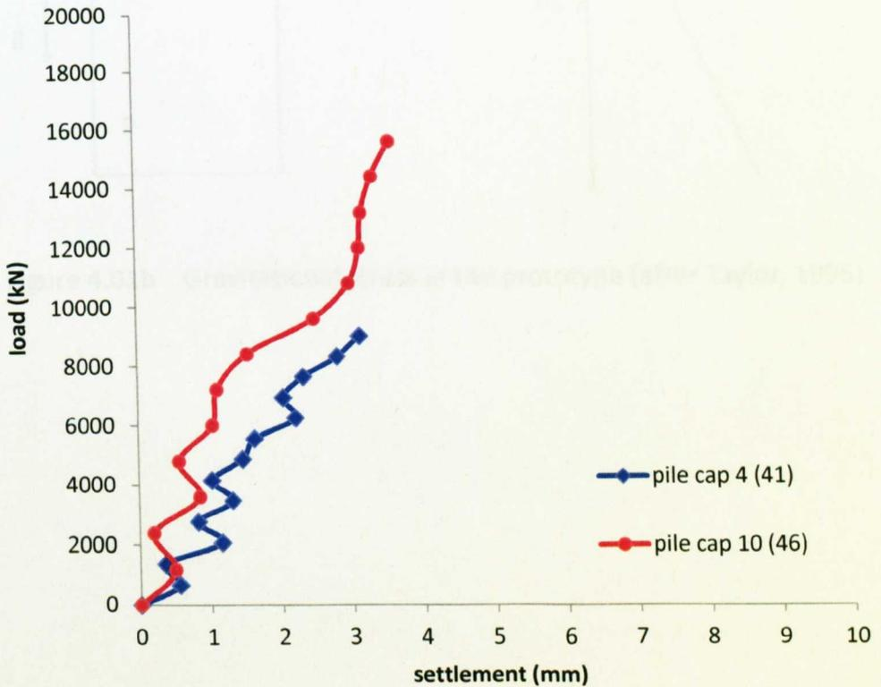
Figure 3.12 Load vs settlement: perimeter group monitoring
