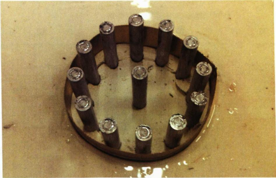
Figure 5.24 Oil prevention techniques: brass ring (test 4e)
