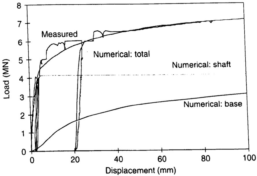
Figure 2.02 Components of capacity:  $Q_s$  and  $Q_b$  (Fleming et al, 2009)
