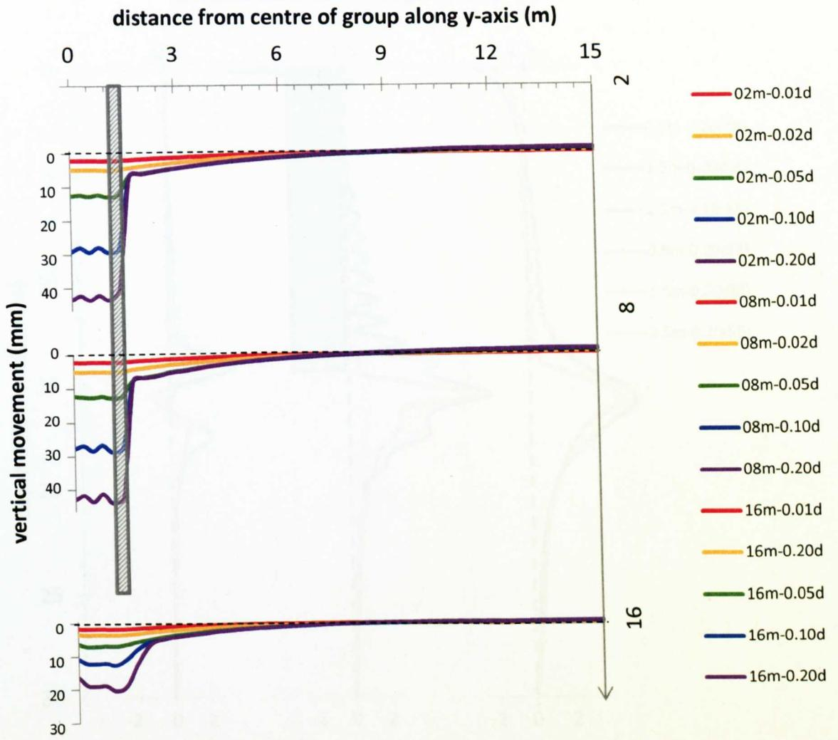
Figure 8.23 Vertical soil movement change with settlement ( $sp_A$ )
