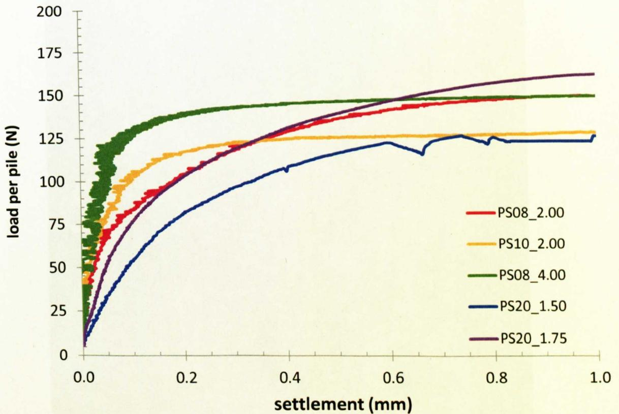
Figure 6.15 Load vs settlement (0 – 1 mm): perimeter groups (square)
