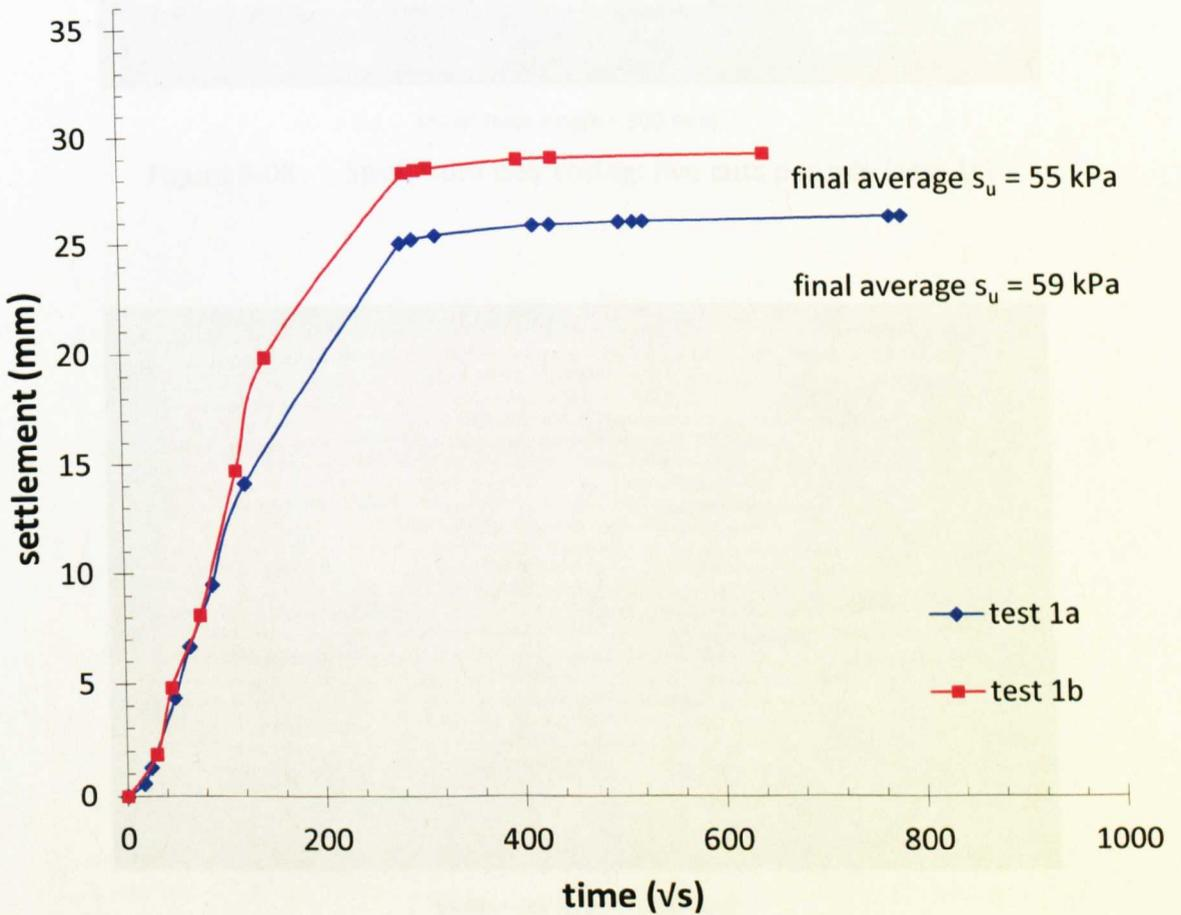
Figure 5.06 Consolidation to 500 kPa: settlement vs time
