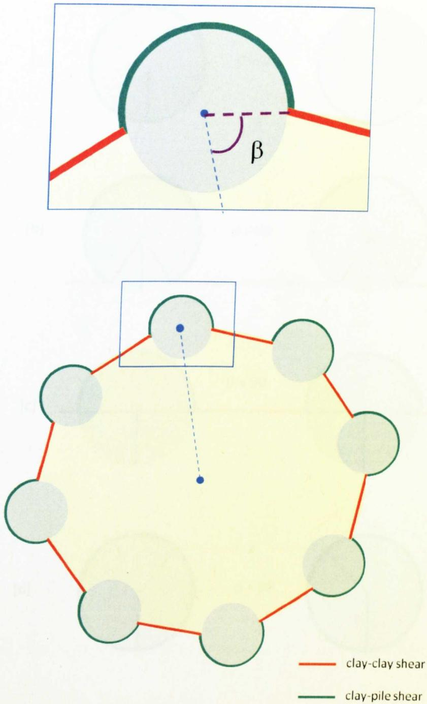
Figure 6.23 Distinction between clay-clay shear and clay-pile shear; and definition of  $\beta$
