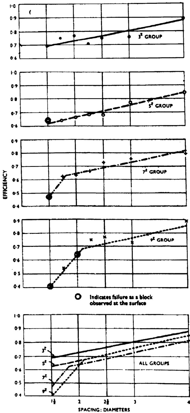
Figure 2.04 Spacing vs efficiency: grid groups with  $l/d = 24$  (Whitaker, 1957)
