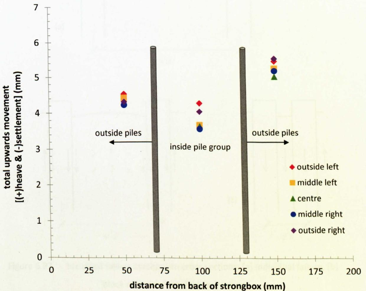
Figure 6.20 Central soil settlement measurements of PC20\_2.00
