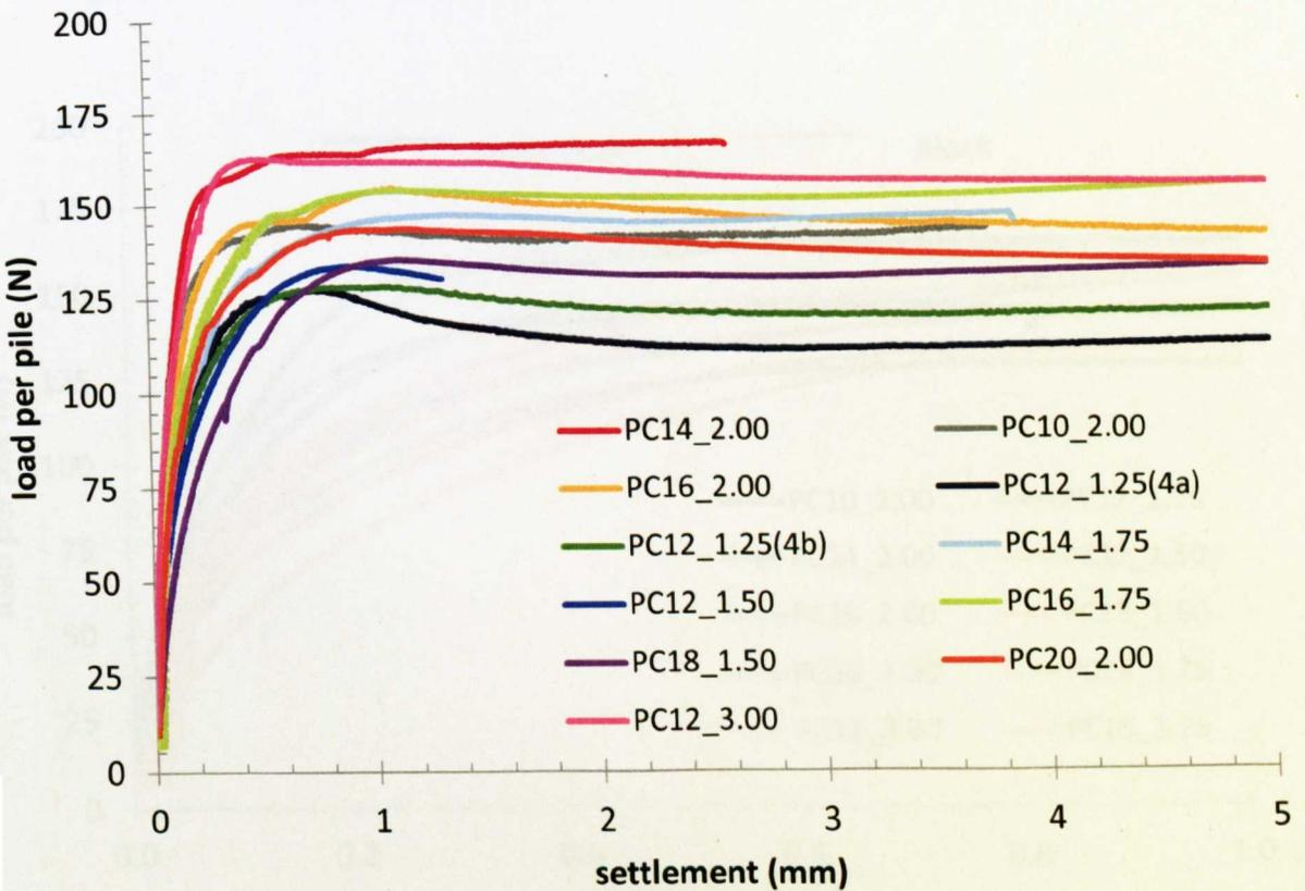
Figure 6.11 Load vs settlement (0 - 5 mm): perimeter groups (circular)
