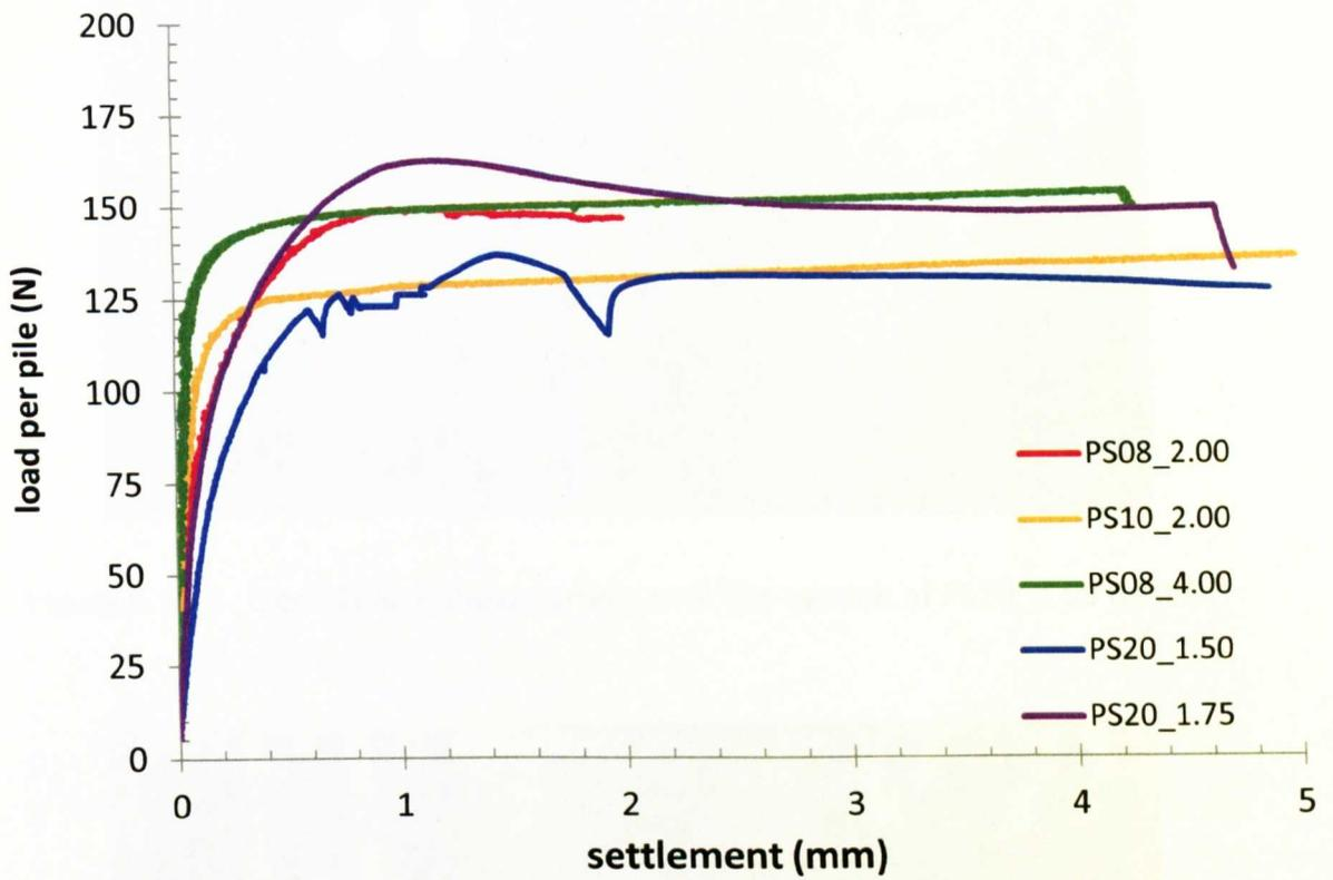
Figure 6.14 Load vs settlement (0 – 5 mm): perimeter groups (square)
