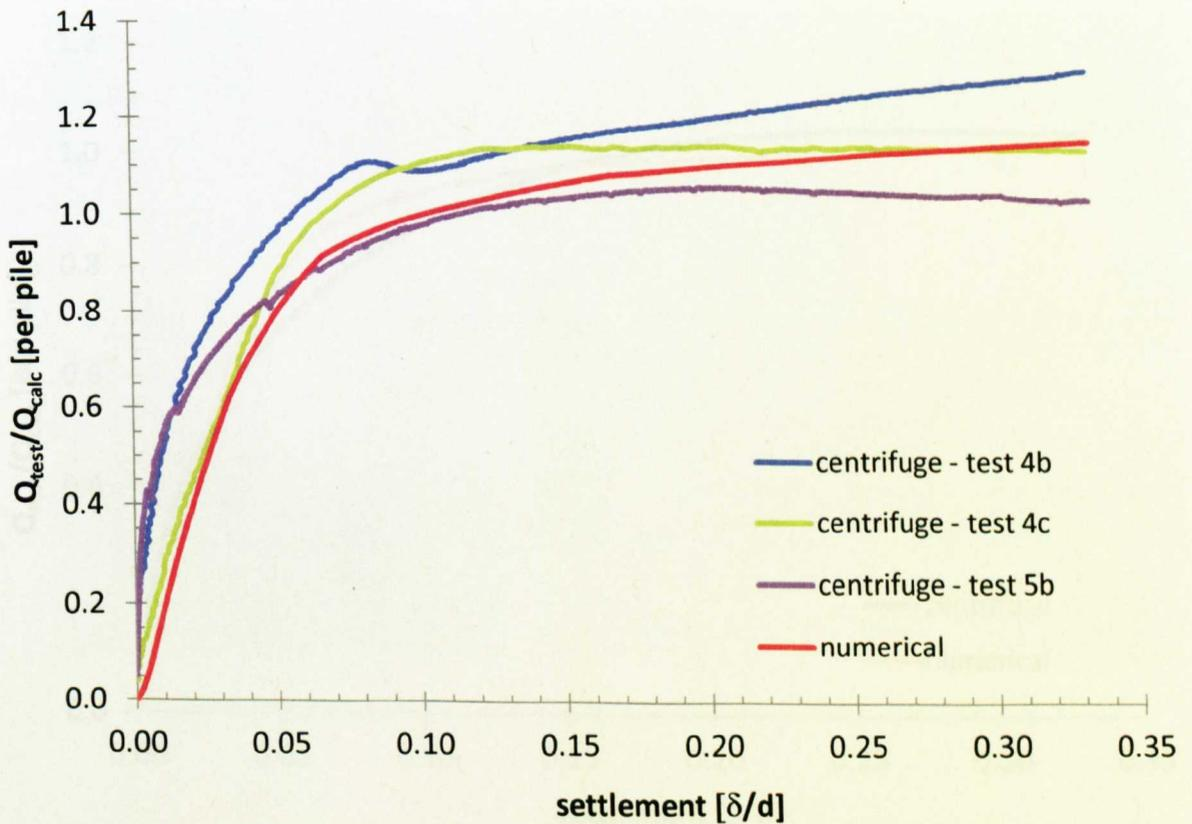
Figure 8.08  $Q_{test}/Q_{calc}$  vs settlement comparison: TS16\_2.00
