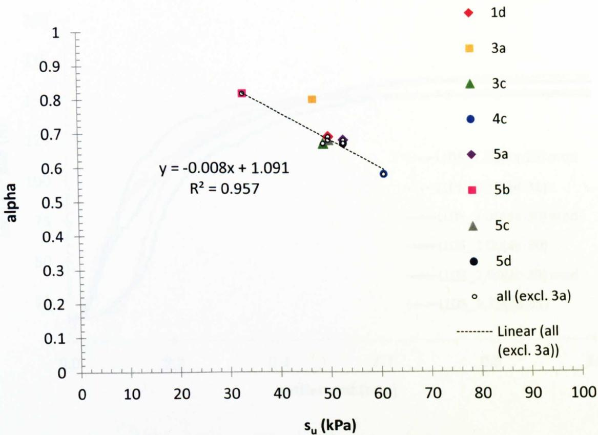
Figure 6.06  $\alpha$  vs  $s_u$ : from hand vane tests and back calculations
