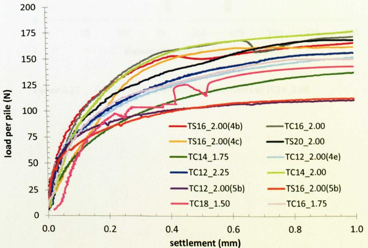
Figure 6.30 Load vs settlement (0 – 1 mm): target groups
