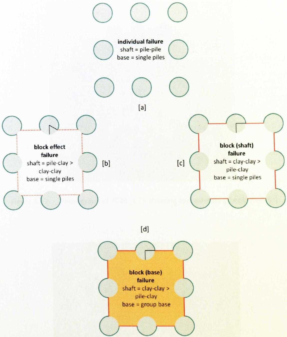
Figure 6.26 Change in  $Q_s$  and  $Q_b$  and the contribution to total capacity: [a] individual failure, [b] 'block effect' failure, [c] and [d] block failure
