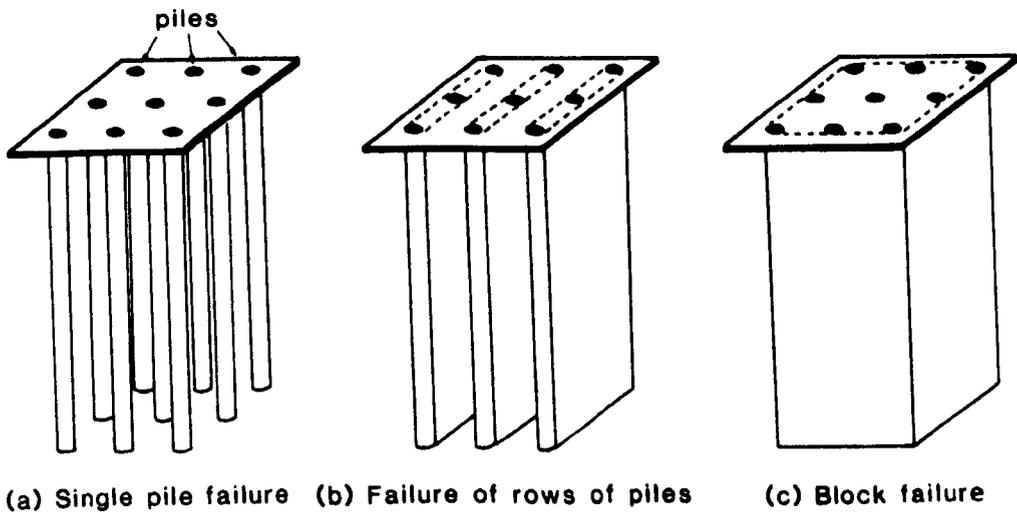
Figure 2.03 Idealised group failure planes (Fleming et al, 2009)
