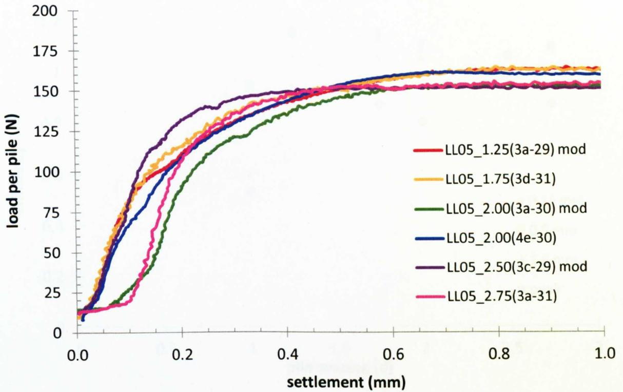
Figure 6.08 Load vs settlement (0 – 1 mm): linear groups
