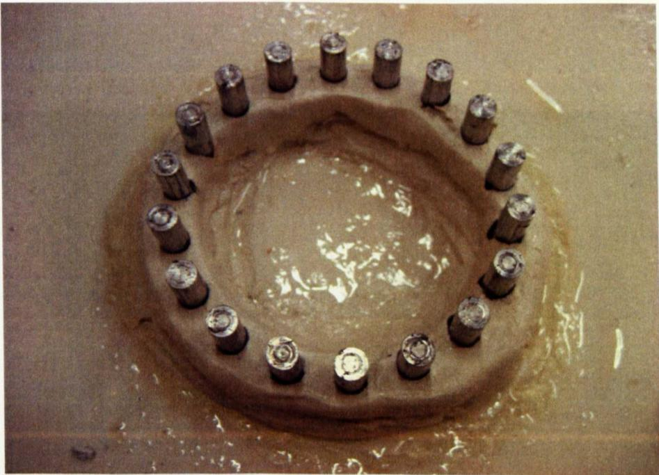
Figure 5.23 Oil prevention techniques: clay bund (test 2b)
