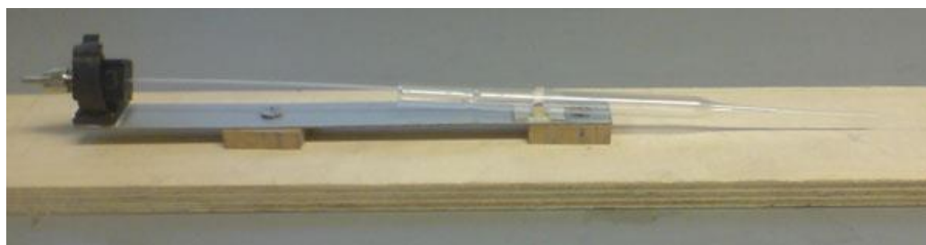
Fig.5.5b Picture of the probe used to gather experimental data. The SMA connector is on the left and will connect to the fibre bundle. The glass capillary tube is on the right with the fibre probe inserted deep inside.
