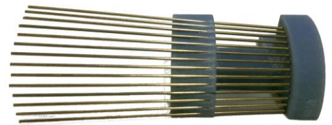
Figure 6. Guide produced by high-resolution 3D printer for precise installation of brass rods.
