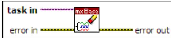
Figure 9.15: Diagram of DAQmx Base Clear Task VI.
