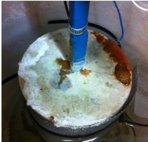
Figure 5.7. Photo of corroding cylinder.
