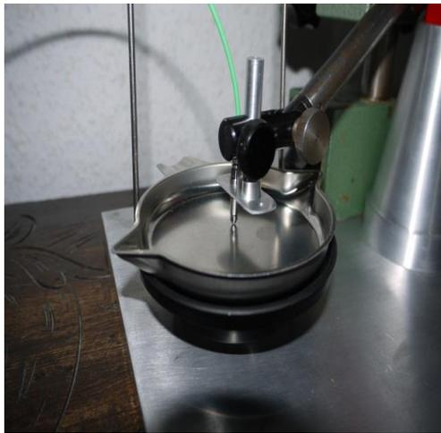
Figure 5.10 Calibration of the low force sensor.
