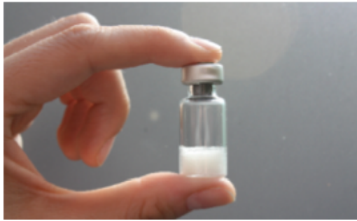
Glass vial containing the ARSOLux biosensor
