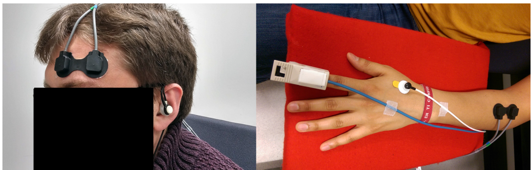
FIGURE 11.2: Photograph of the measurement set-up showing the forehead NIRS sensor and the ear canal PPG sensor on the left, and the finger PPG probe on the index finger, NIRS sensor on the forearm and LDF sensor on the back of the hand on the right.
