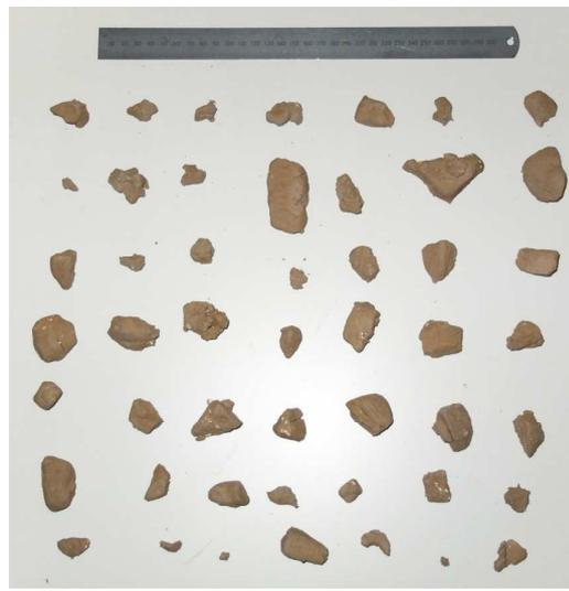
London Clay post 10 minute mixing test (dried and sized)
