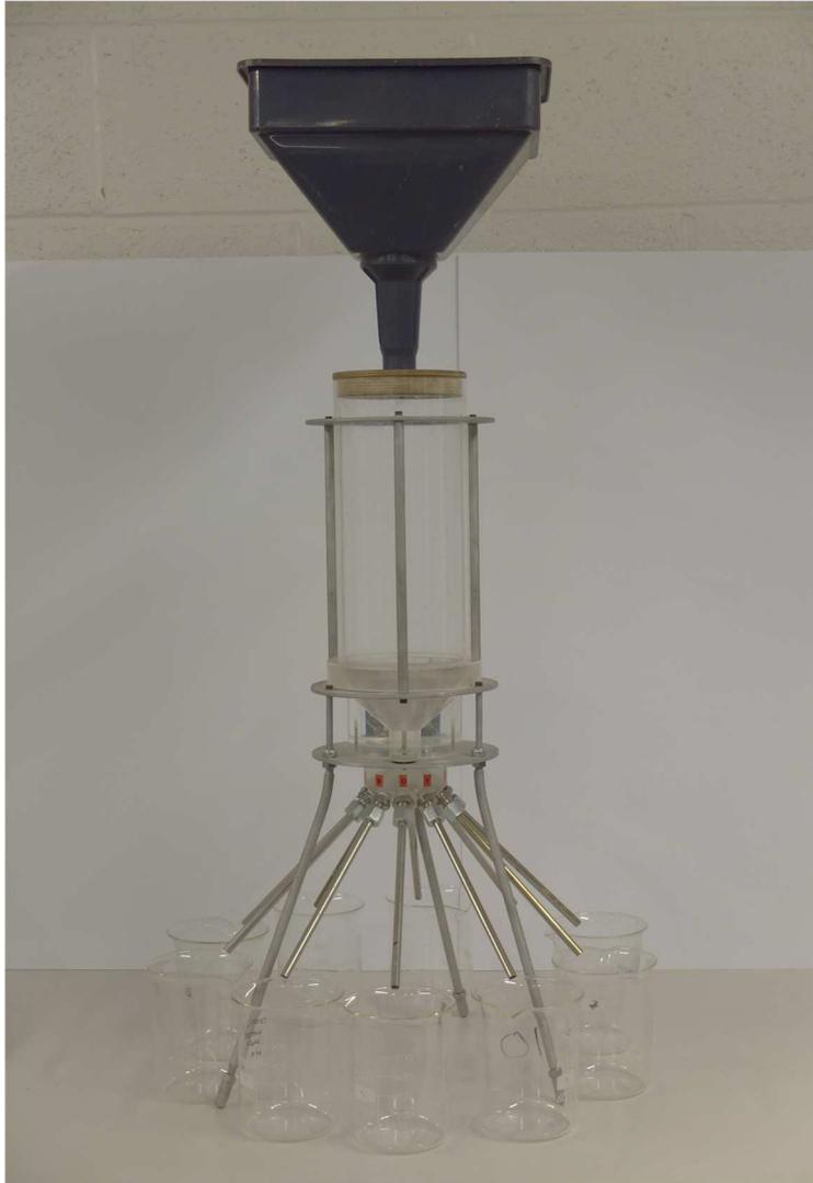
**Figure 4.9 10 way cone splitter and beaker set-up**
