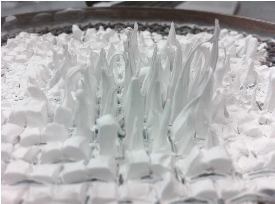
**Figure 5.2 Extrusion of Speswhite Kaolin through 4.75 mm sieve**
