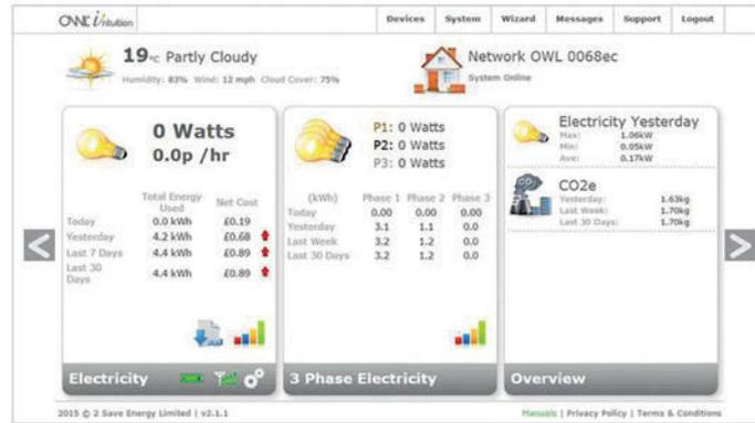
Figure 5: Power meter for monitoring the energy consumption.
