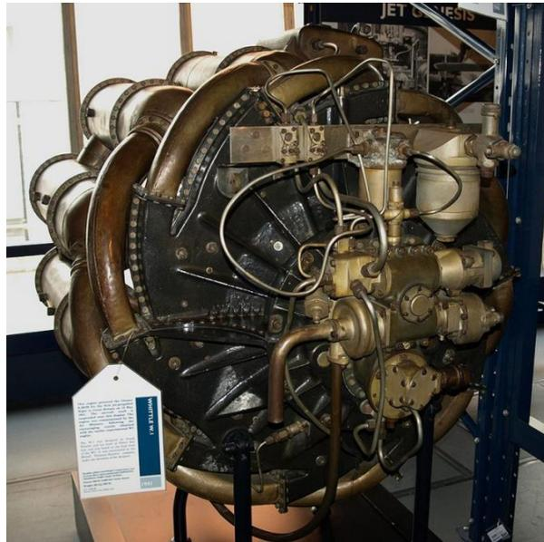
Figure 1.1: Power Jets W.1, Type: Turbojet [2].
