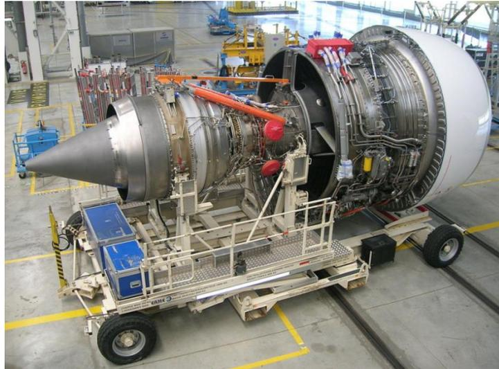
Figure 1.3: Rolls-Royce Trent 900 engines, Type: Turbofan [4].
