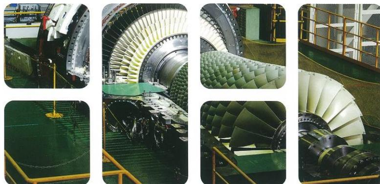
Figure 1.2: J-series gas turbine developed by Mitsubishi Heavy Industries, Ltd [3].
