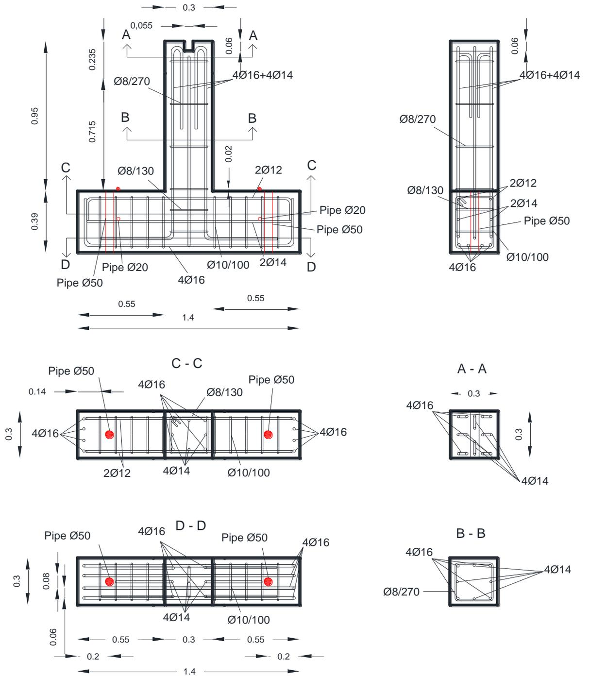
Figure C-3: As-built design drawings of FSC specimens.
