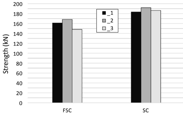
Figure 7-9 : Comparison of the maximum horizontal strength, for FSC and SC specimens.
