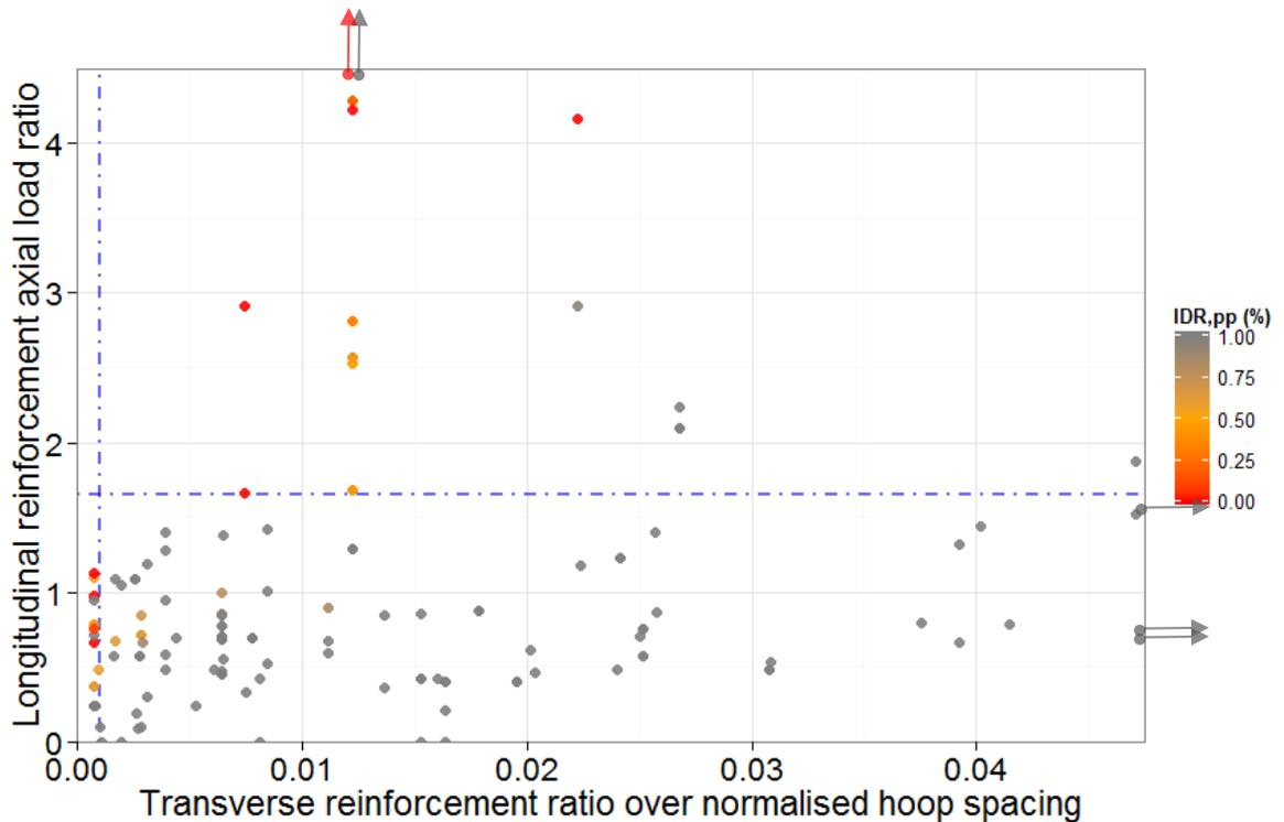
Figure 5-4: Values of  $IDR_{pp}$  depicted against longitudinal reinforcement axial load ratio and transverse reinforcement ratio over normalised hoop spacing. Values greater than 1% are in grey colour. Some points are shown with arrows, indicating accurately one of their coordinates and that the other one is higher than the maximum of the range of the respective axis.
