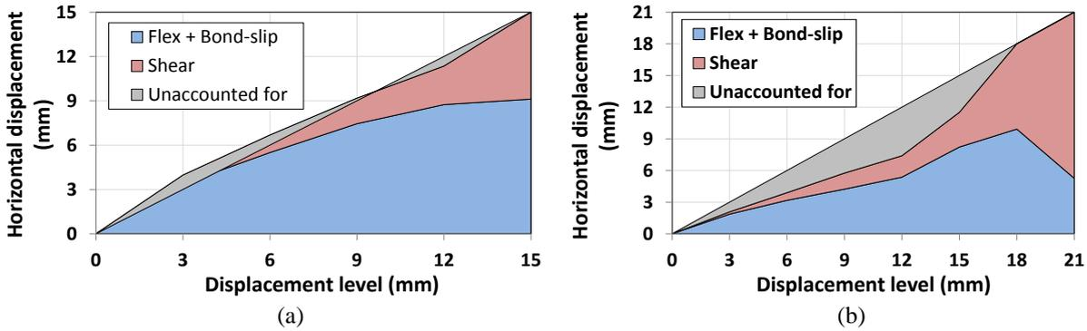
Figure 7-18: Lateral displacement decomposition for (a) FSC\_3, and (b) SC\_3, including the 'unaccounted for' component.
