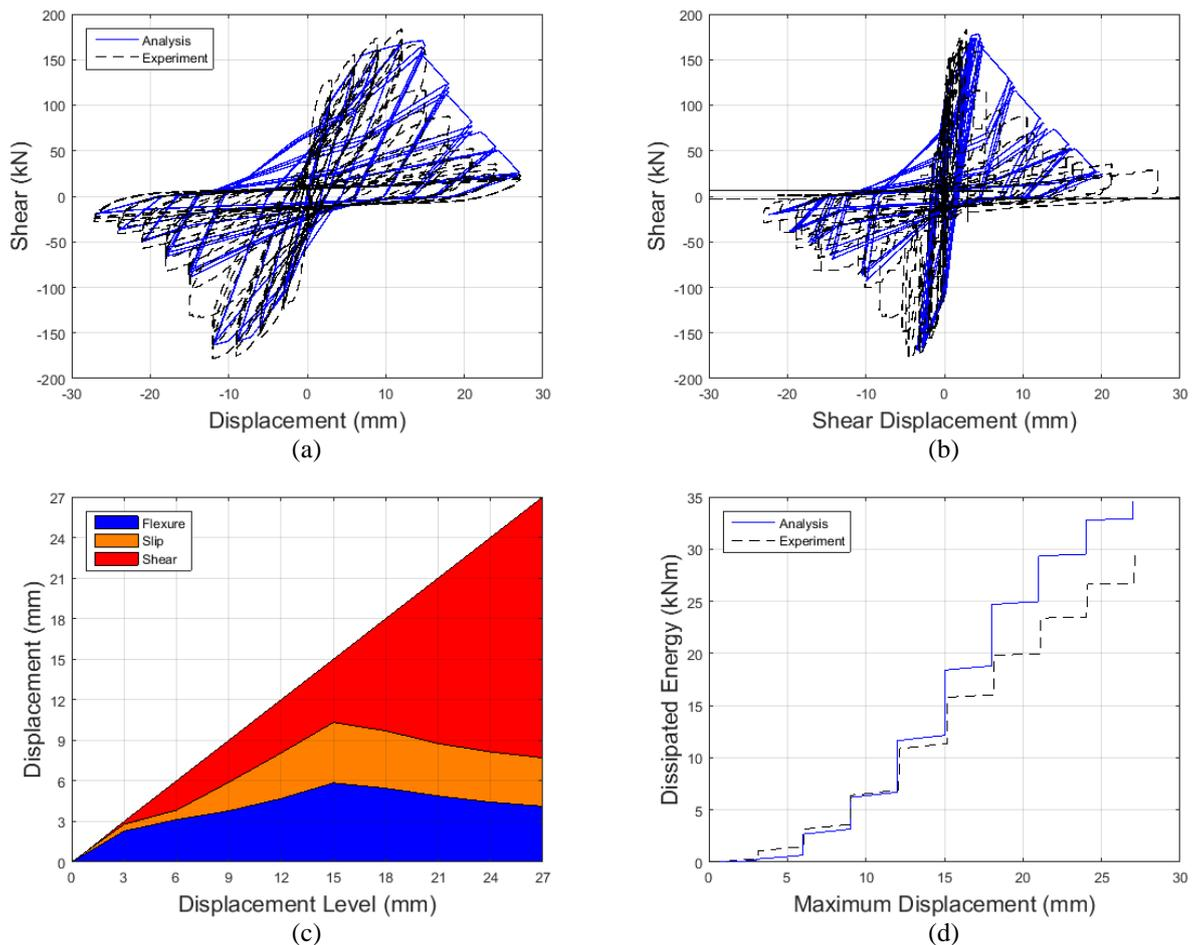
Figure 9-8: Comparison between the predicted response of SC\_1 by the proposed model and the experimental one in terms of (a) shear force against lateral displacement, and (b) shear displacement. (c) Decomposition of the element's lateral displacement components throughout the analysis. (d) Comparison between predicted and experimental cumulative dissipated energy.
