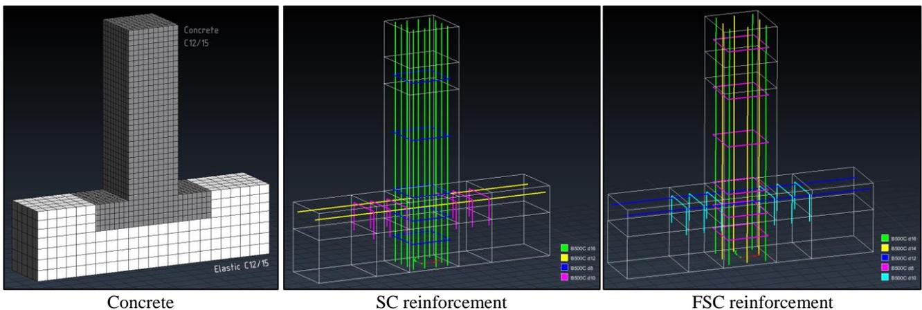
Figure 6-10: Numerical 3D finite element model (concrete / reinforcement).
