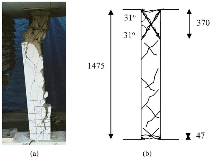
Figure 9-17: (a) Photographic documentation of the damage sustained by Frame 2 (Elwood & Moehle, 2008b); (b) predicted damage by the proposed model.
