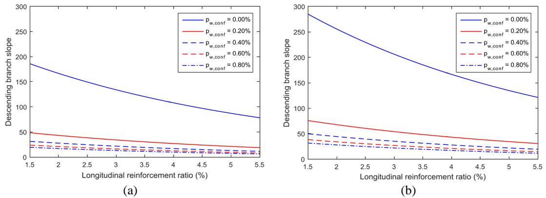
Figure 4-11: Descending branch slope ( $S_{pp}$ ) predicted by Eq. 4-6 along the range of potential longitudinal reinforcement ratios over relative confined concrete area ( $\rho_l/a_{conf}$ ), for different transverse reinforcement ratios over confined concrete area ( $\rho_{w,conf}$ ), for axial load ratios ( $\nu$ ) of (a) 0.2 and (b) 0.5.
