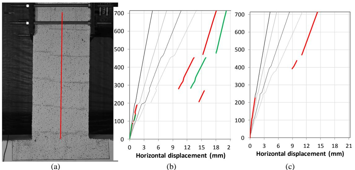
Figure 7-22: Lateral displacement profiles along the centroidal axis of specimen (b) SC\_2 (displacement levels +3 mm until +18 mm from left to right), and (c) FSC\_3 (+3 mm until +15 mm from left to right).
