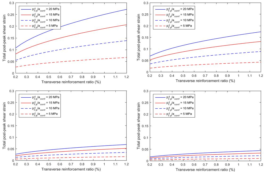
Figure 4-16: Total post-peak shear strain predicted by Eq. 4-16 along the range of longitudinal reinforcement ratios (over confined area) and transverse reinforcement ratios (over confined concrete area), for longitudinal reinforcement axial load ratios of 0.2 (top) and 0.5 (bottom) and maximum shear stress of 0.25 (left) and 0.75 (right).
