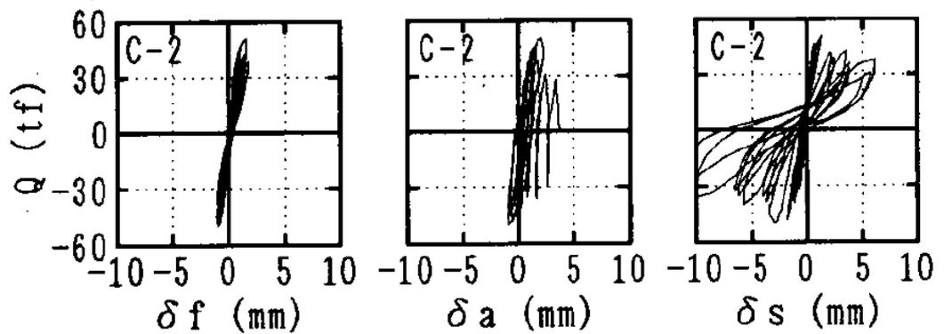
Figure 2-2: Deformation components of specimen C-2's response. (Lejano *et al.* 1995)
