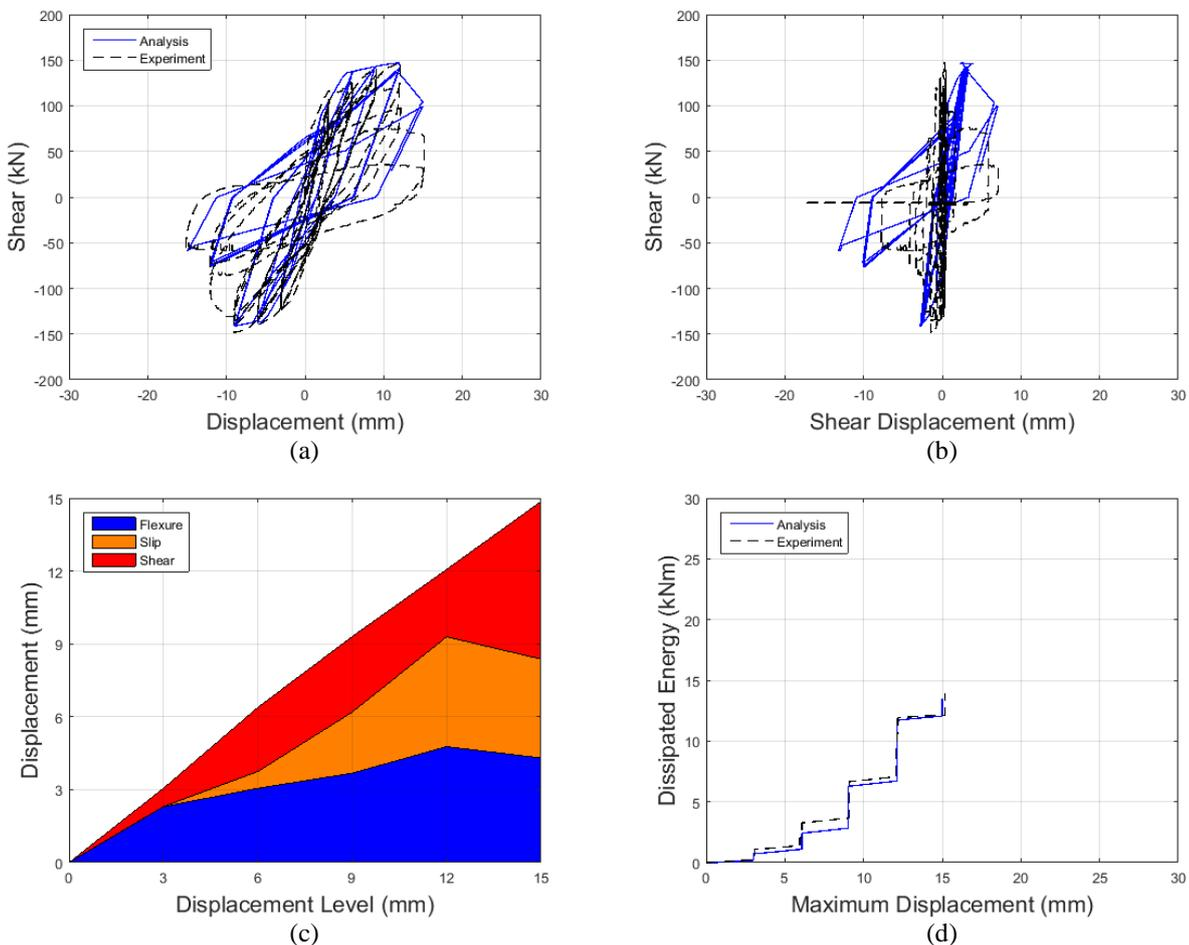
Figure 9-21: Comparison between the predicted response of FSC\_3 by the proposed model and the experimental one in terms of (a) shear force against lateral displacement, and (b) shear displacement. (c) Decomposition of the element's lateral displacement components throughout the analysis. (d) Comparison between predicted and experimental cumulative dissipated energy.
