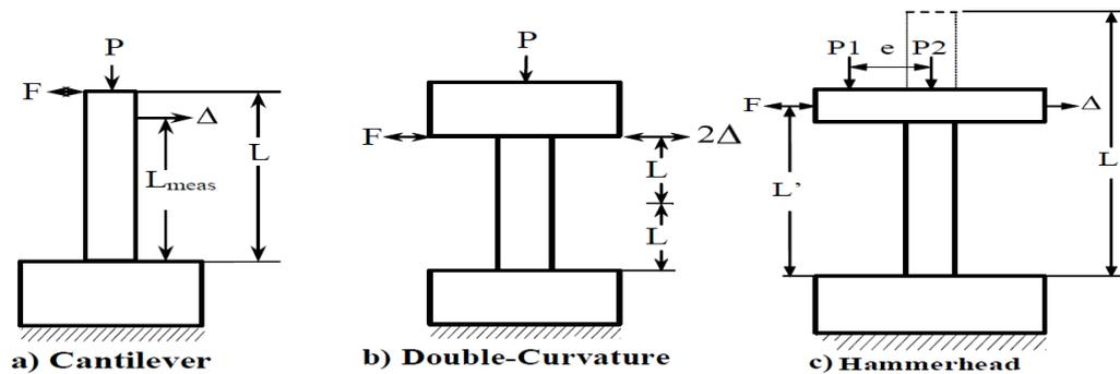
Figure 3-5: Column test configuration types. (Berry et al., 2013)
