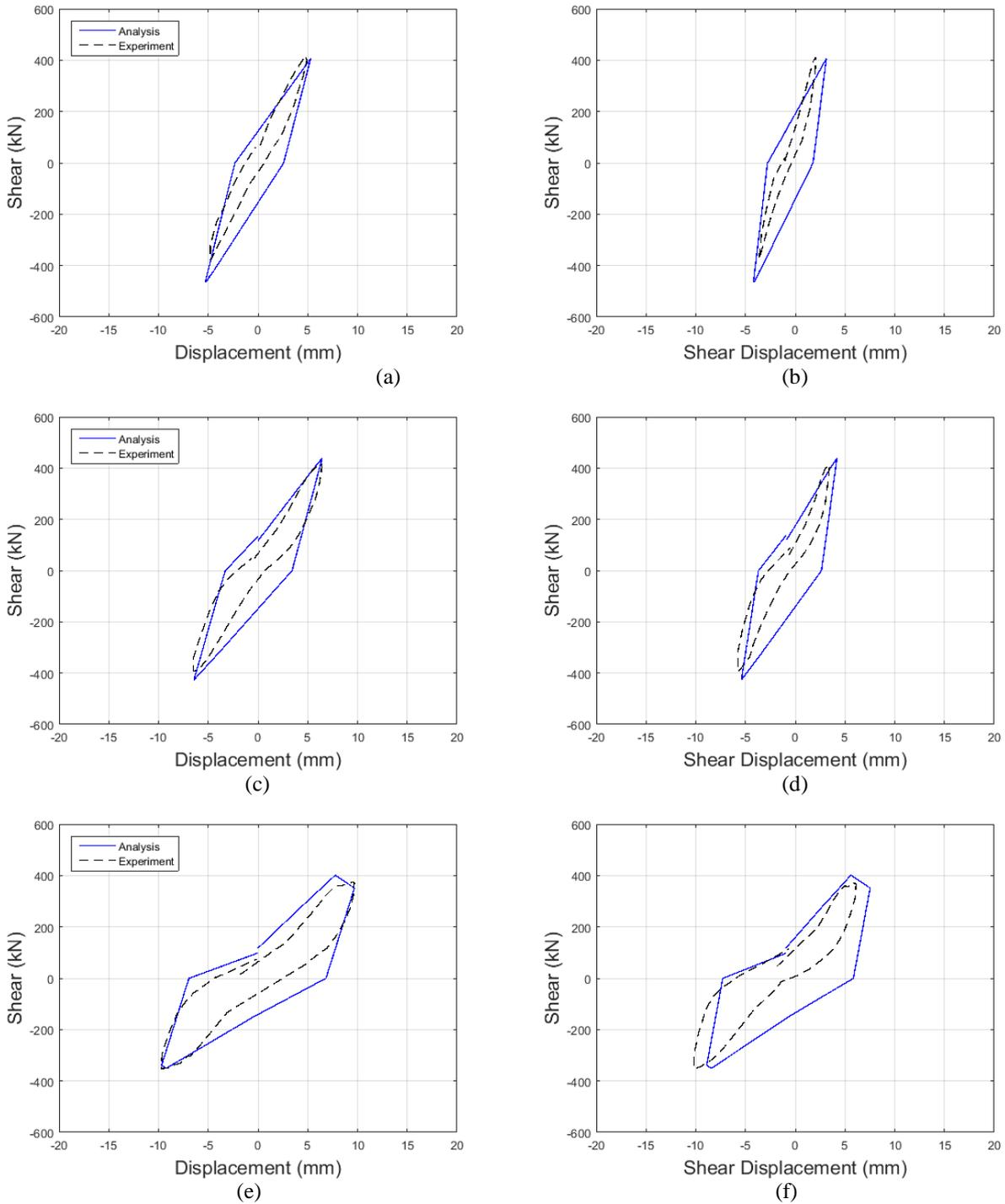
Figure 9-6: Comparison between individual cycles of the predicted response of C-2 by the proposed model and the experimental one: (a, b) 2<sup>nd</sup> cycle at +/- 5 mm, (c, d) 1<sup>st</sup> cycle at +/- 6.5 mm, and (e, f) 1<sup>st</sup> cycle at +/- 10 mm. (left) Total displacements and (right) shear displacements.
