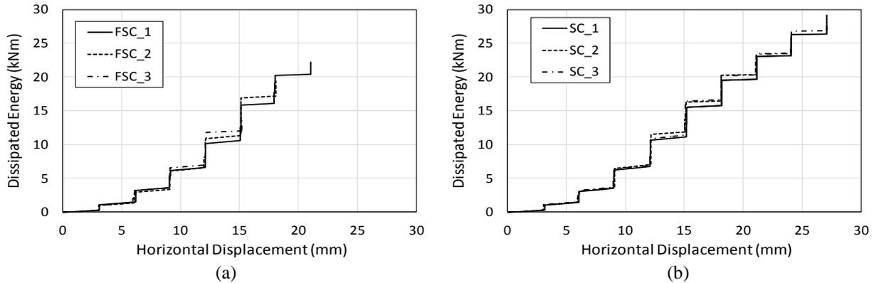
Figure 7-26: Cumulative dissipated energy against displacement level for (a) FSC, and (b) SC specimens.
