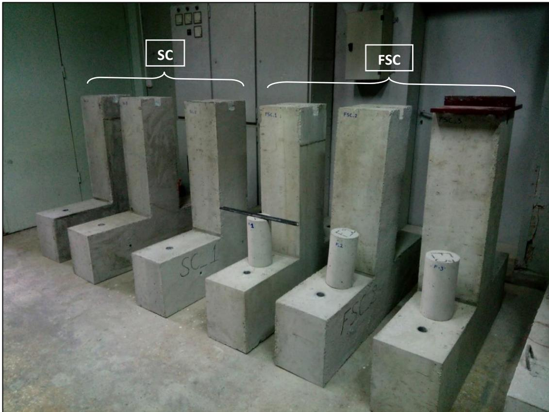
Figure 6-17: Shear critical (SC) and flexure-shear critical (FSC) specimens after construction.
