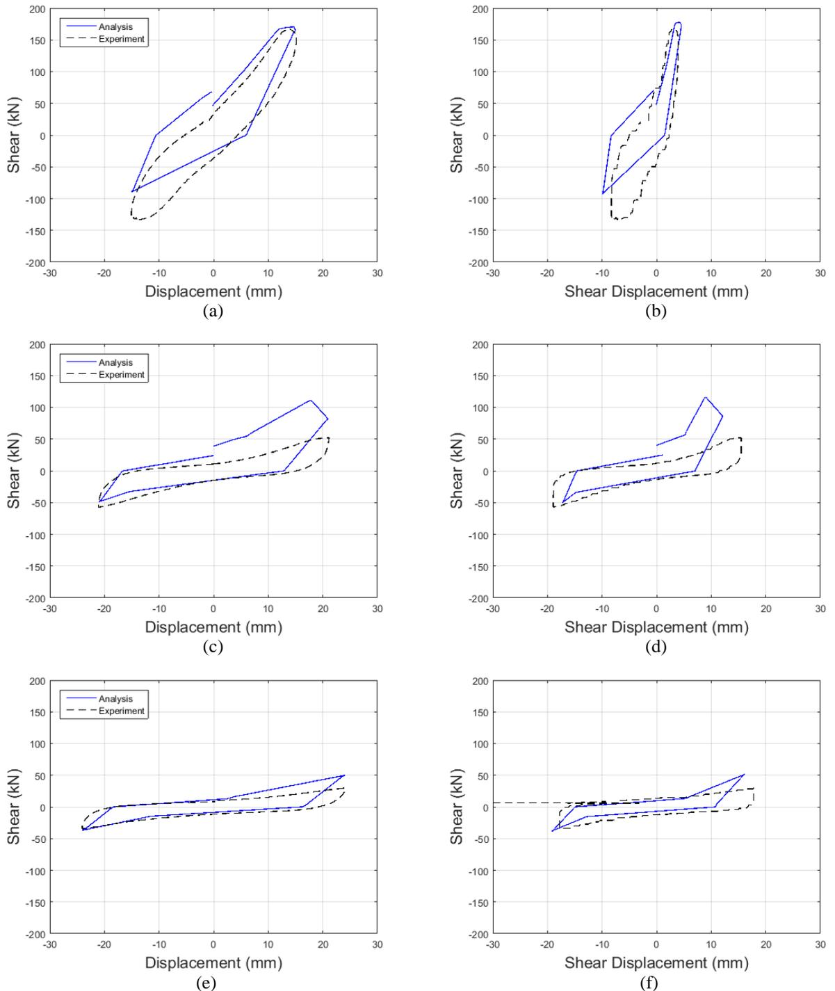
Figure 9-9: Comparison between individual cycles of the predicted response of SC\_1 by the proposed model and the experimental one: (a, b) 1<sup>st</sup> cycle at +/- 15 mm, (c, d) 1<sup>st</sup> cycle at +/- 21 mm, and (e, f) 2<sup>nd</sup> cycle at +/- 24 mm. (left) Total displacements and (right) shear displacements.
