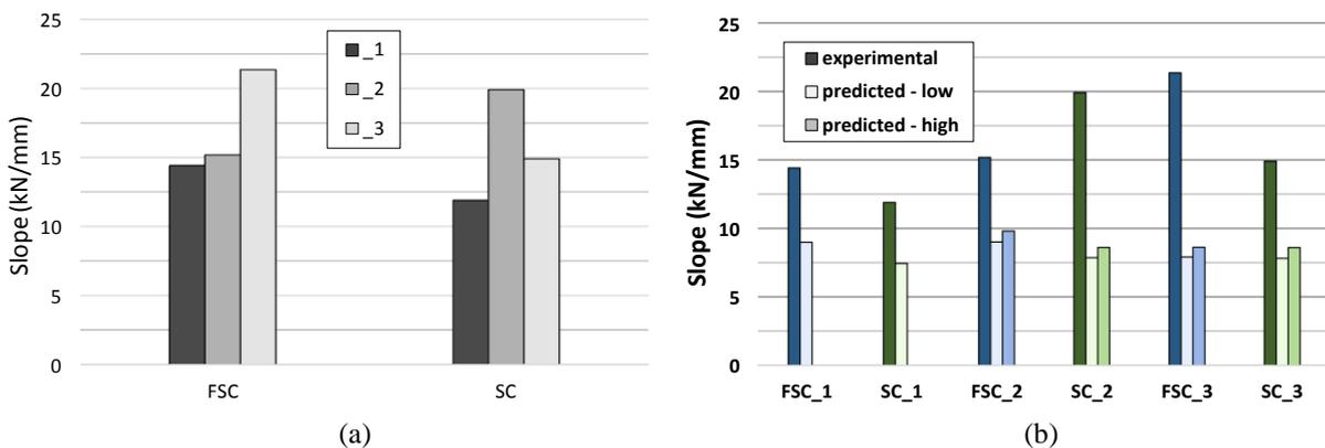
Figure 7-29: (a) Experimentally obtained descending branch slopes of FSC and SC specimens. (b) Comparison of experimentally obtained against analytically predicted descending branch slopes of each specimen.
