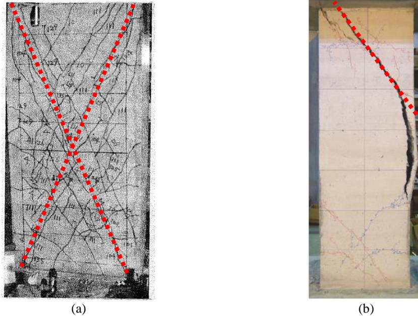
Figure 3-11: Indicative extraction of critical shear crack angle from experimental photographic documentation: specimens by (a) Umehara & Jirsa (1982), and (b) Nakamura & Yoshimura (2014).
