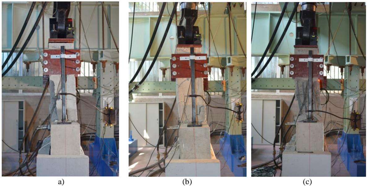
Figure 7-5: Side view at the onset of axial collapse of (a) FSC\_2, (b) FSC\_3 and (c) SC\_2.
