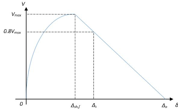
Figure 5-5: Schematic representation of displacement derived from Elwood & Moehle model.
