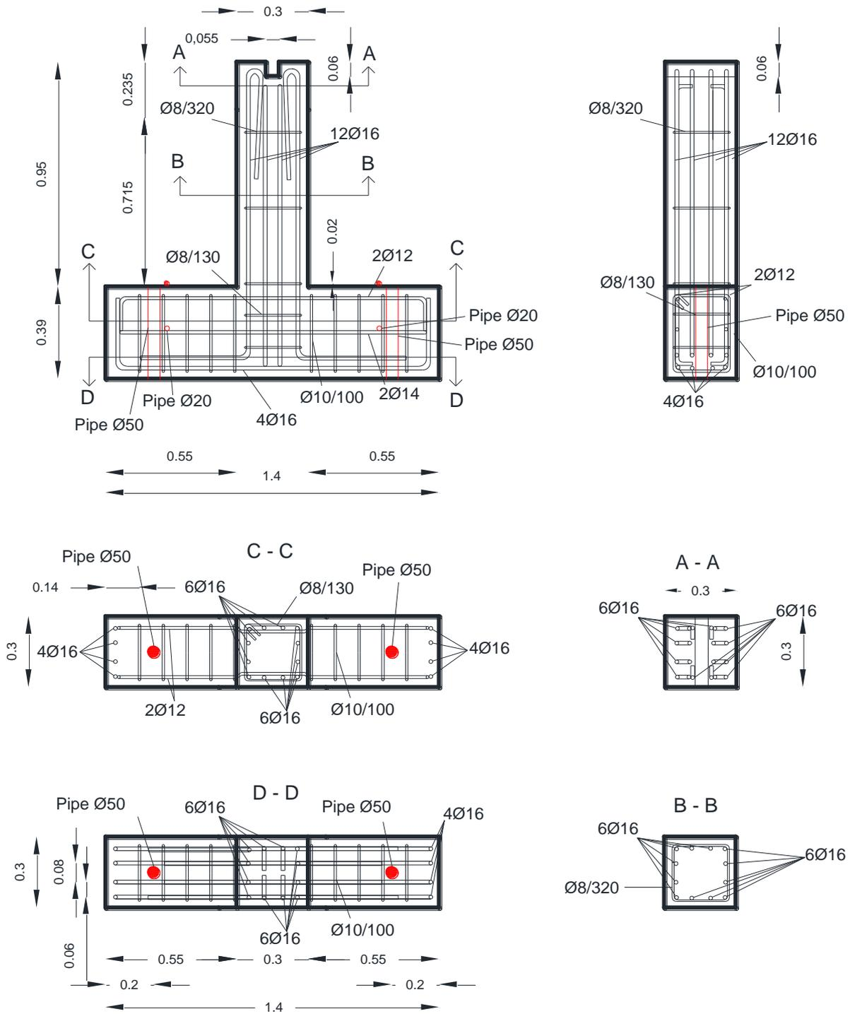
Figure C-2: As-built design drawings of SC specimens.
