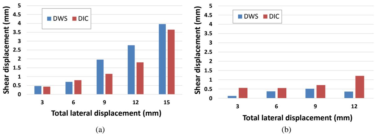
Figure 7-14: Comparison between shear displacement recorded by the Draw-Wire Sensors (DWS) and calculated via Digital Image Correlation (DIC) for specimens (a) SC\_1, and (b) FSC\_3.
