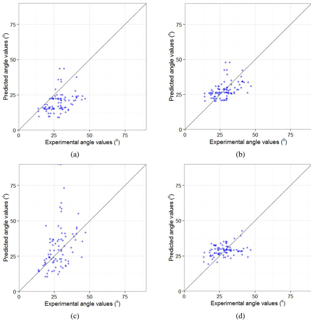
Figure 4-2: Shear crack angles measured experimentally against those calculated using the predictive models of (a) Chang (1993), (b) Kim & Mander (1999), (c) Ousalem et al. (2003), and (d) Elwood & Moehle (2005a).
