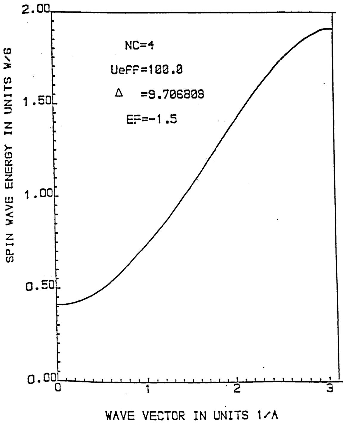
Fig.27. Spin wave energies for a single-adlayer system calculated from Eq.(3.8) without  $\text{Im}G_{11\downarrow}$ . This is an example of not treating the  $\chi^{\text{HF}}(\omega, q_{\parallel})$  exactly in the HF approximation which gives rise to an unphysical gap and breaks the Goldstone theorem
