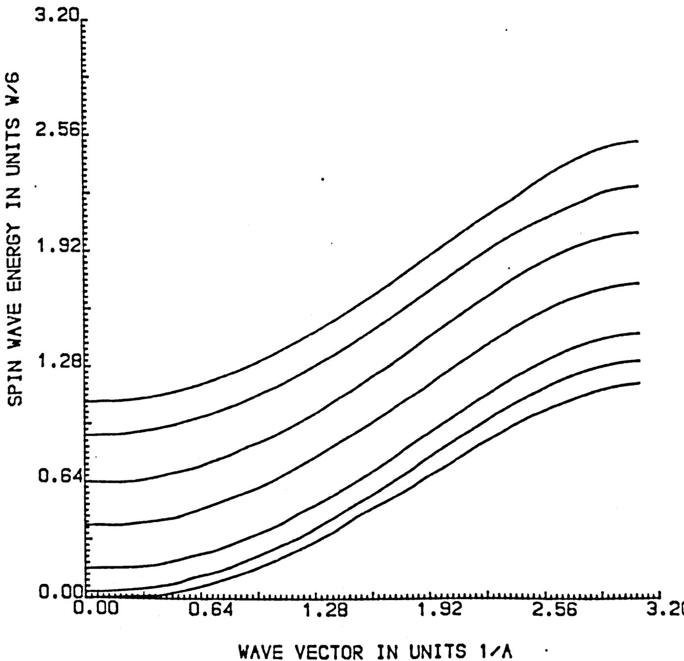
Fig.33. Spin wave modes in an overlayer of seven atomic planes above a (100) non-magnetic metallic substrate with  $E_F = -1.5$ ,  $UHUB = 30.5$  and  $NC = 4$ . The dashed lines indicate spin waves decay into the Stoner continuum.
