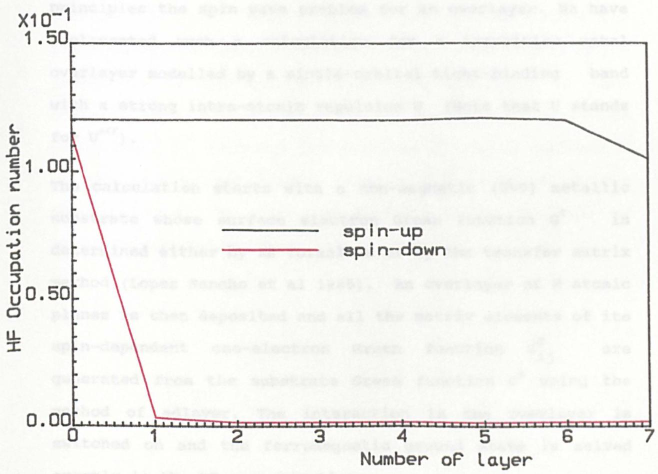
Fig.18 Distribution of spin-up and spin-down particles per atom at Fermi energy  $E_F = -1.5$ ,  $U_{eff} = 30.5$  and  $N_C = 64$ .
