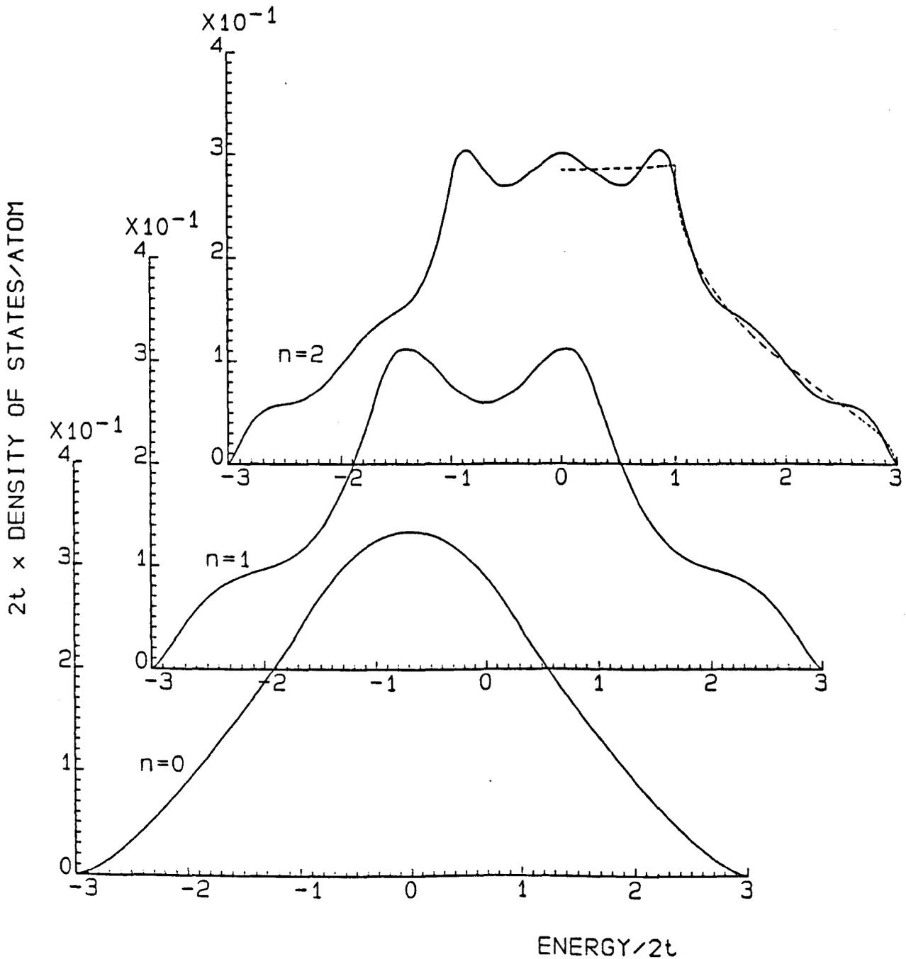
Fig.5. Local density of states for the surface( $n=0$ ) and the first two interior planes in the presence of a (100) surface. The surface perturbation  $U_s$  is zero. The dashed curve in the upper figure is the infinite crystal density of states per atom.
