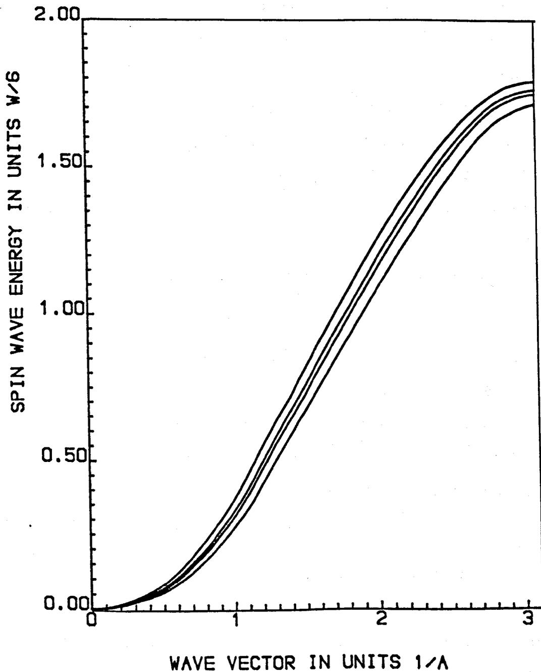
Fig.25. Spin wave spectrums For a single-adlayer on top of a  $(100)$  non-magnetic metallic substrate with different coulomb interactions  $U = 100.0, 39.97, 30.5$  and  $20.5$  starts from top to bottom curve respectively. Here  $E_F = -1.5$  and  $NC=4$  in all four spectrums of spin wave.
