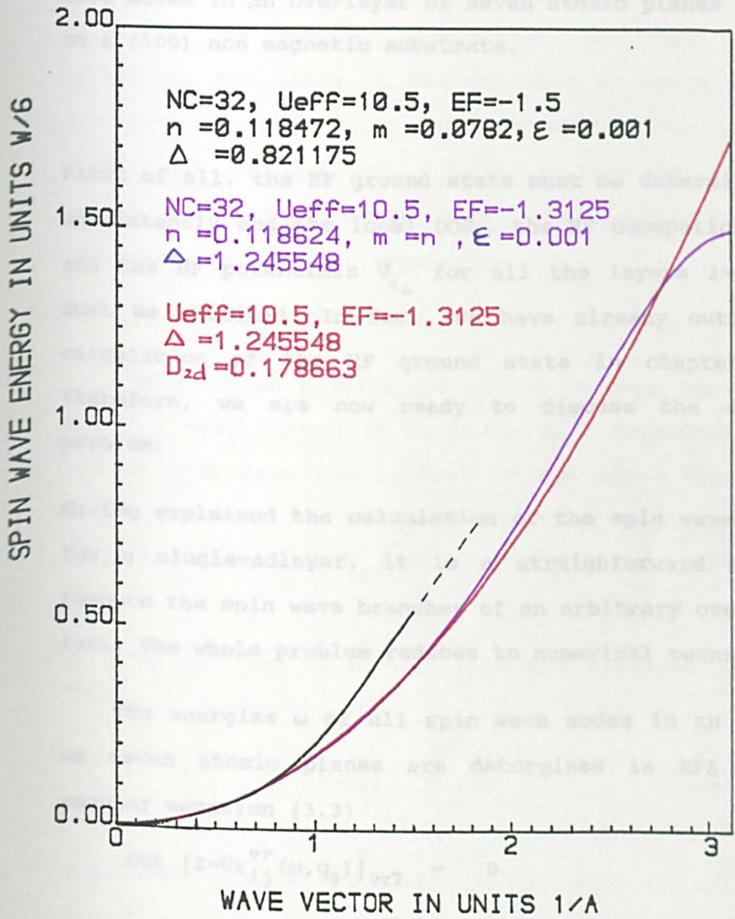
Fig.30. A comparison between spin wave energies of a single-adlayer (black colour) and an unsupported layer (purple colour) are presented. The red curve represents the  $Dq_x^2$  relation with D in two-dimensional of an infinite Ferromagnetic system. The dashed line indicates the spin wave enters the Stoner continuum.
