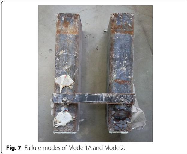
**Fig. 7** Failure modes of Mode 1A and Mode 2.
