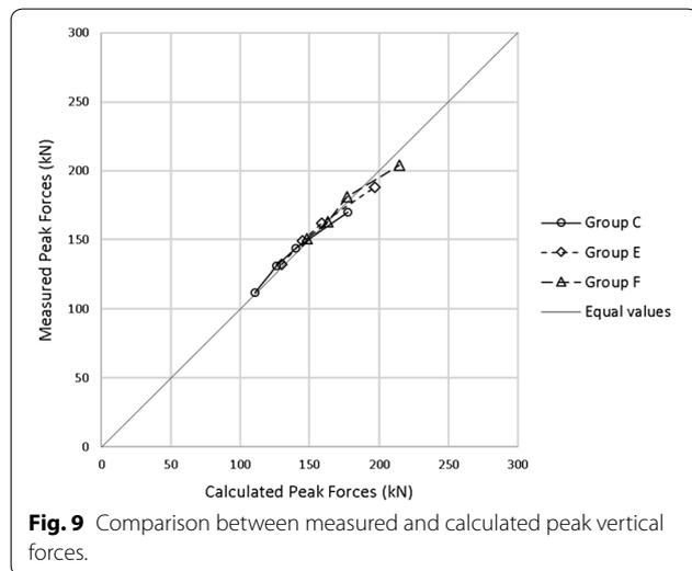
**Fig. 9** Comparison between measured and calculated peak vertical forces.
