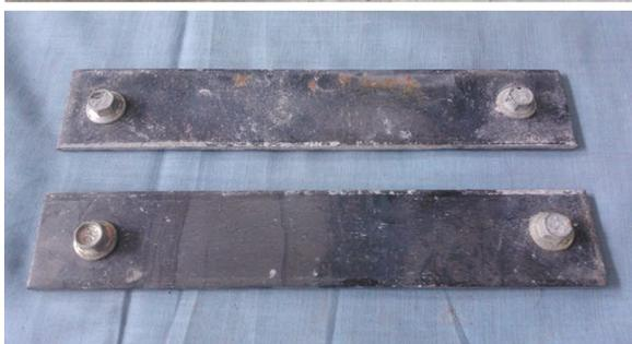
(b) Failure Mode of Flange Connectors
