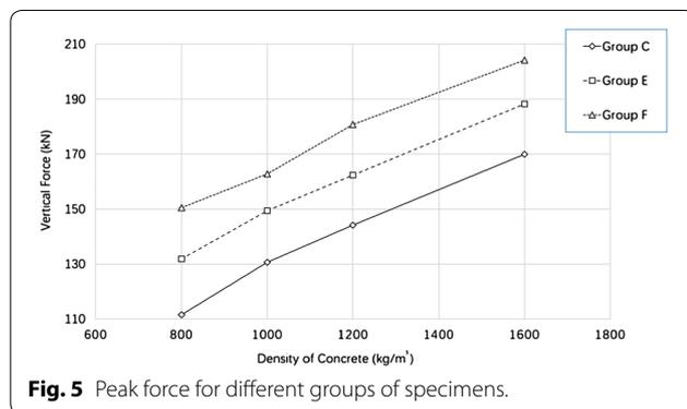
**Fig. 5** Peak force for different groups of specimens.
