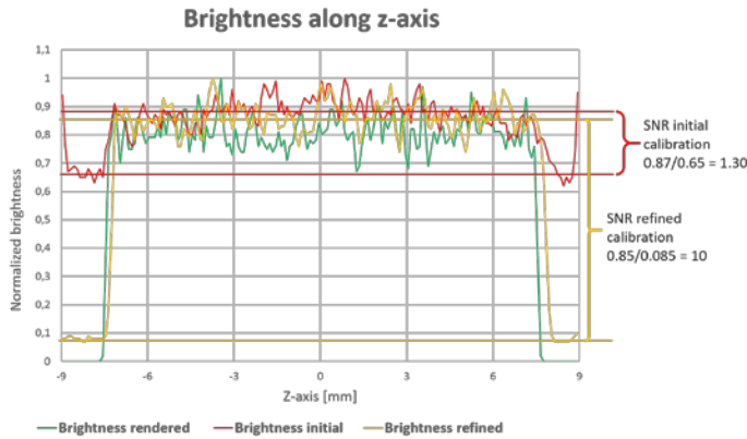
Fig. 11: comparison of z-axis intensity profiles in the 3 different voxel-spaces. Red: Voxel space from initial calibration. Green: Voxel space from simulated voxel space. Yellow: Voxel space from refined calibration.
