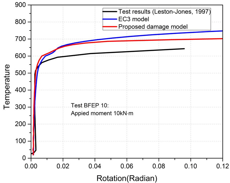
Fig. 4.17 Comparison of connection response between numerical cases and fire test 2 (BFEP10)
