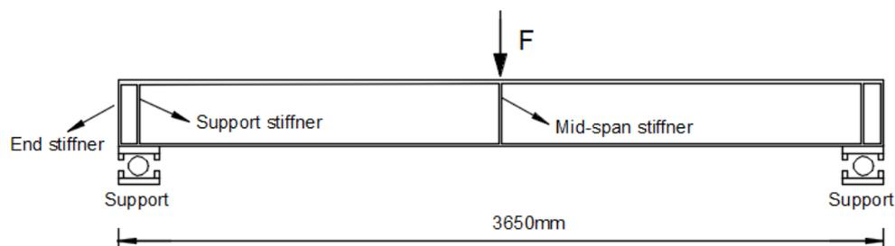
Fig. 4.1 Test set-up (Dharma and Tan, 2007)
