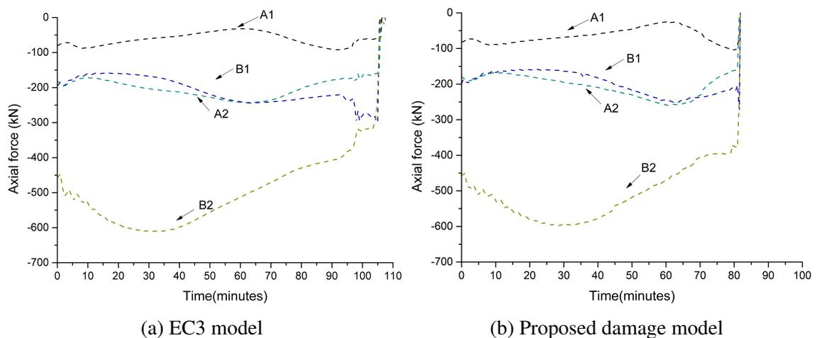
Fig. 5.29 Axial forces in columns during fire event
