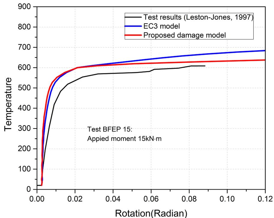
Fig. 4.18 Comparison of connection response between numerical cases and fire test 3 (BFEP15)
