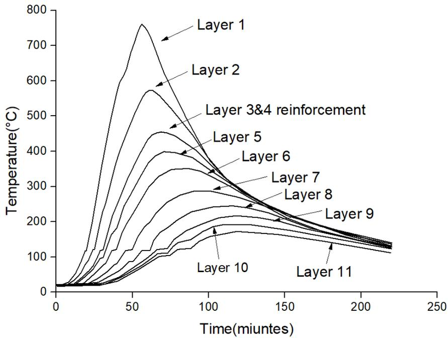
Fig. 4.48 Temperature variation throughout the depth of slab (Foster et al., 2007)
