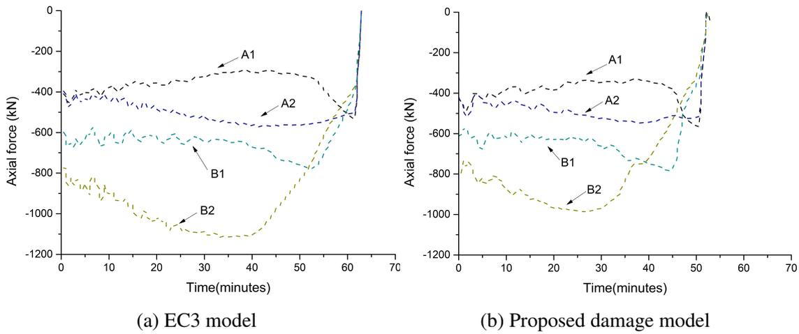
Fig. 5.62 Axial forces in columns during fire event
