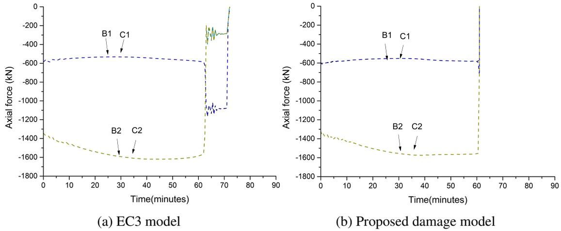
Fig. 5.26 Axial forces in columns during fire event
