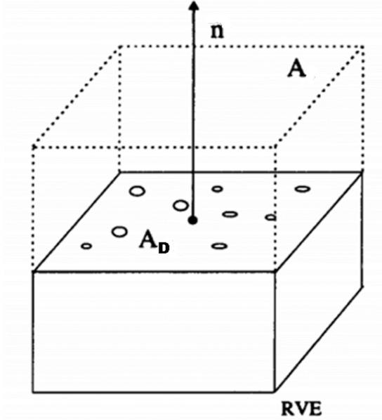
Fig. 2.9 Damaged element (Lemaitre, 1985)
