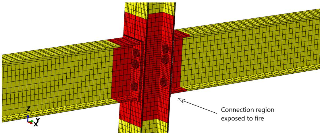
Fig. 4.14 Fire exposed region within connection model
