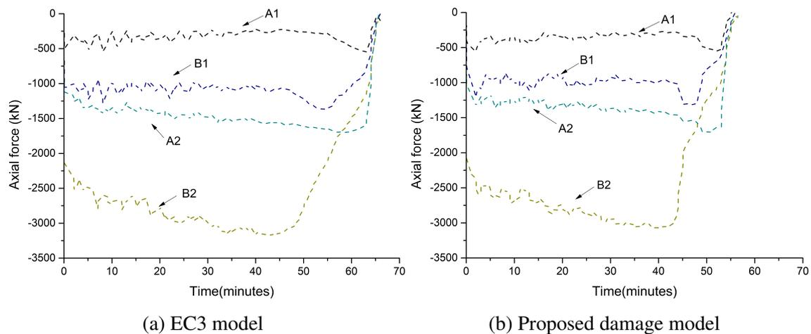
Fig. 5.76 Axial forces in columns during fire event
