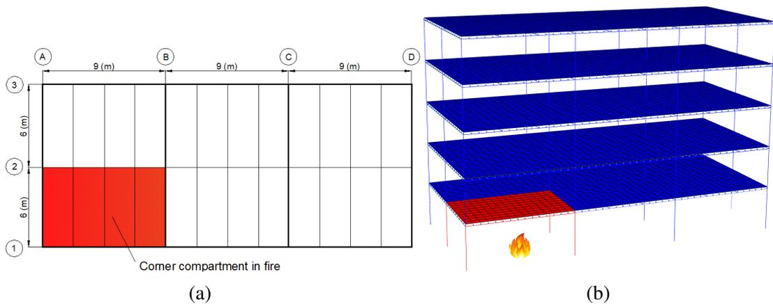
Fig. 5.11 Location of the corner compartment fire on the ground floor
