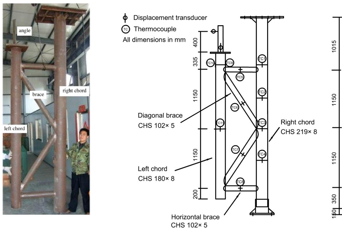
Fig. 4.21 Test set-up (Liu et al., 2010)
