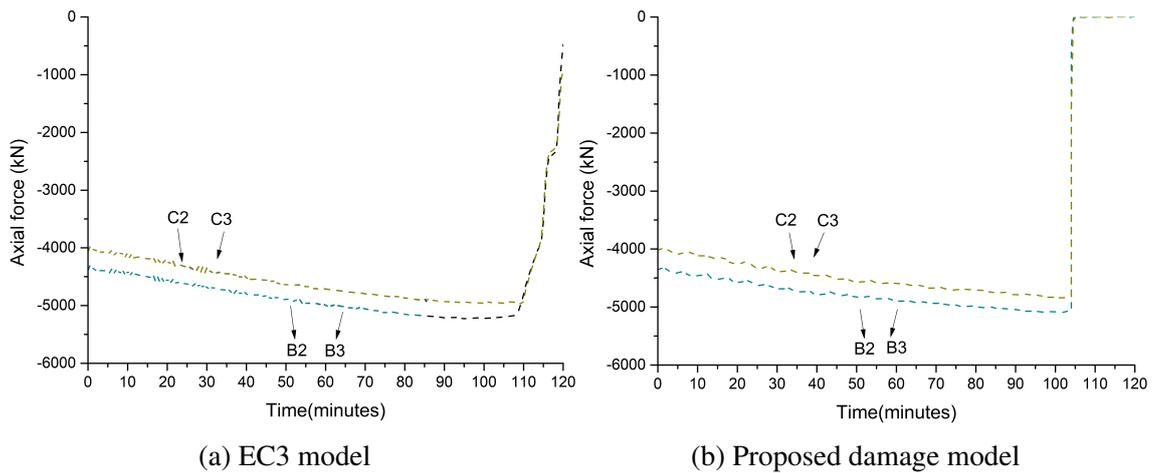
Fig. 5.40 Axial forces in columns during fire event
