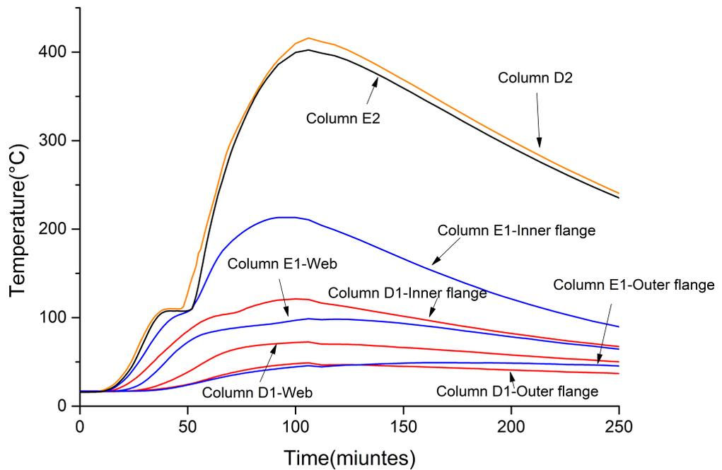
Fig. 4.47 Measured temperatures of columns (Lennon, 2003)
