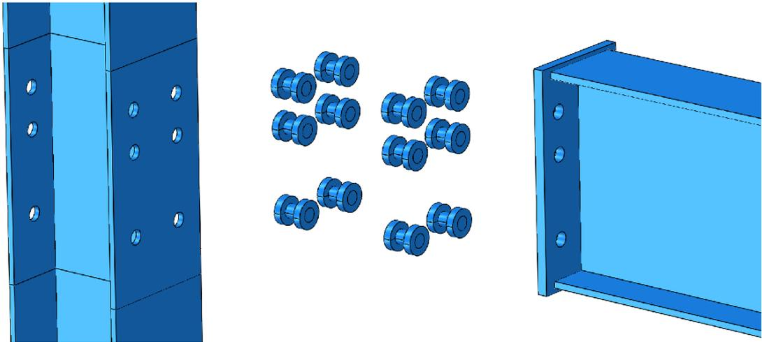
Fig. 4.10 Modelling details of flush end plate connection
