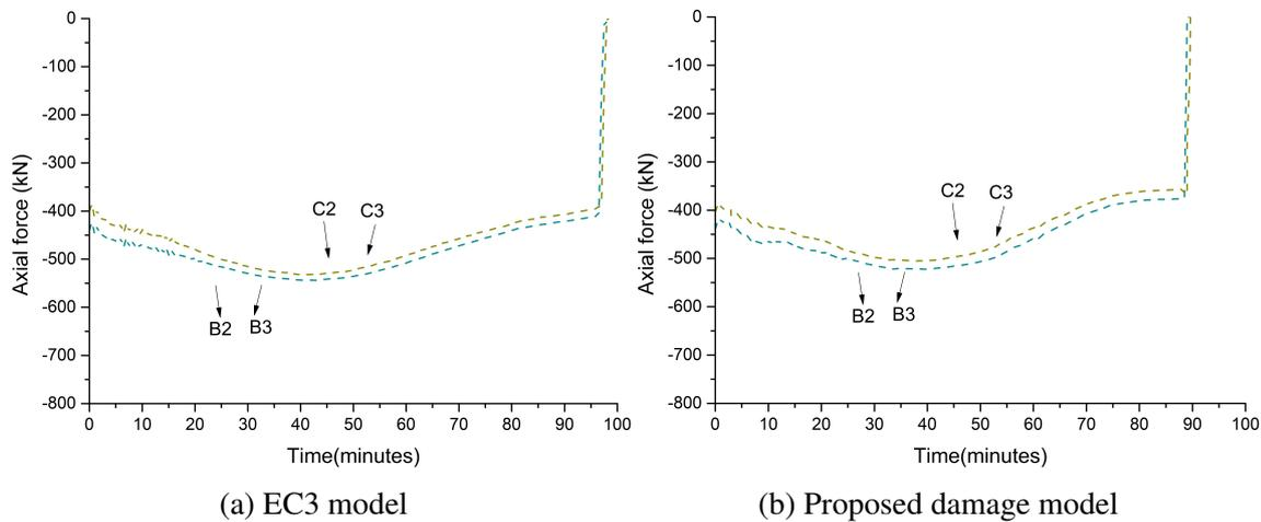
Fig. 5.52 Axial forces in columns during fire event
