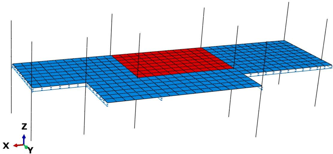
Fig. 4.44 FE model of Cardington test 7 in ABAQUS
