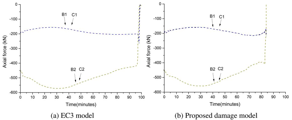
Fig. 5.32 Axial forces in columns during fire event
