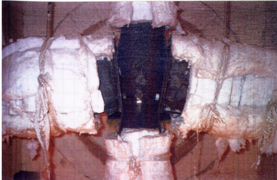
(a) Connection failure mode observed in test BFEP5 (Leston-Jones, 1997)
