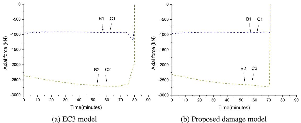
Fig. 5.18 Axial forces in columns during fire event
