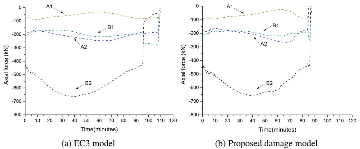
Fig. 5.49 Axial forces in columns during fire event
