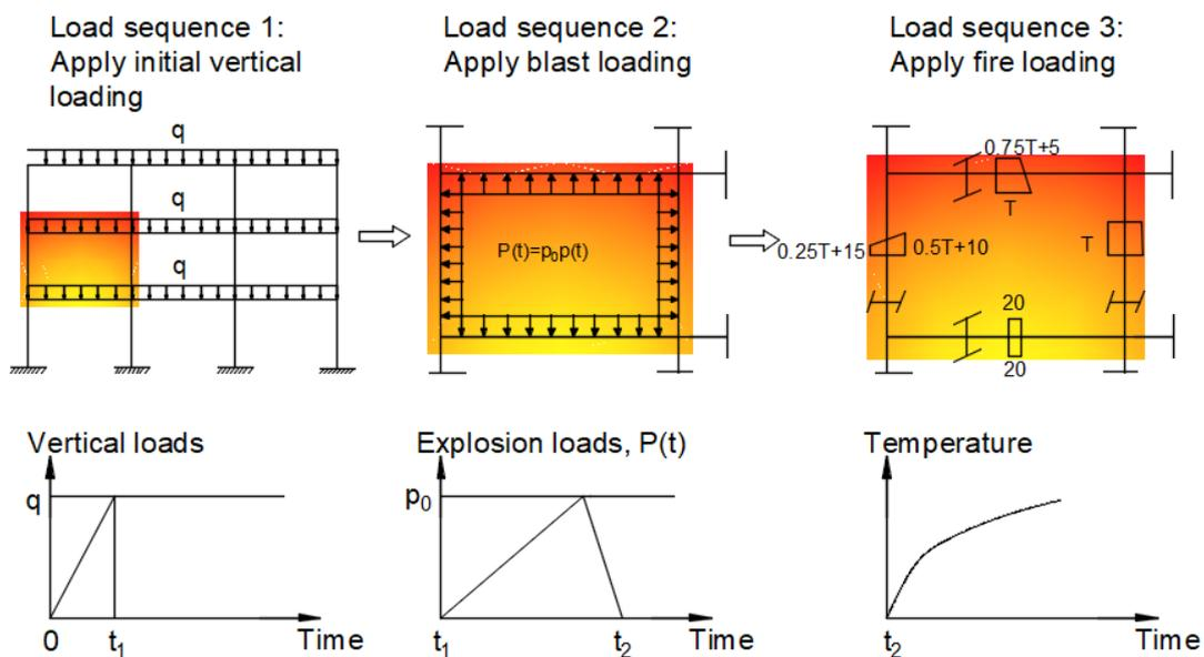
Fig. 4.28 Load sequences in explosion and fire analysis
