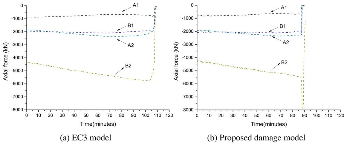
Fig. 5.36 Axial forces in columns during fire event
