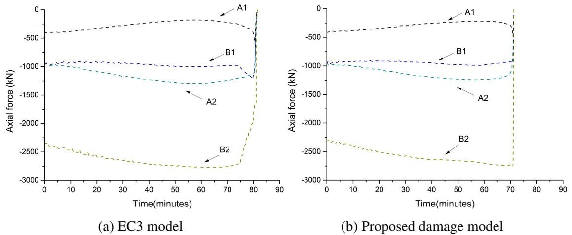
Fig. 5.14 Axial forces in columns during fire event
