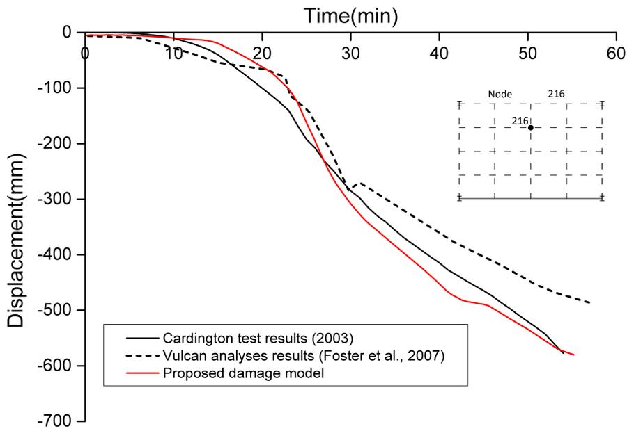
Fig. 4.53 Comparison of displacements at nodes 216 between numerical cases and test
