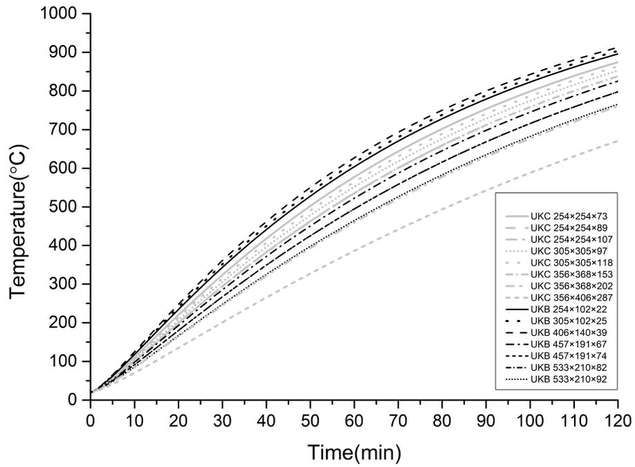
Fig. 5.4 Temperature histories of steel structural members
