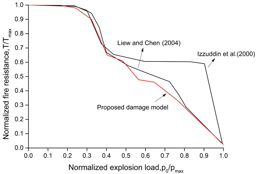
Fig. 4.34 Influence of explosion loads on the fire resistance of steel frame
