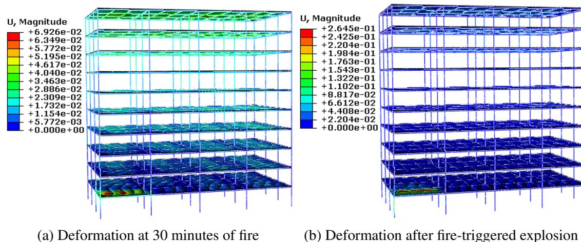
Fig. 5.91 Deformation before and after fire-triggered explosion occurrence
