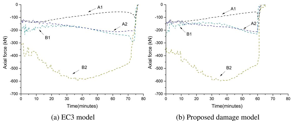
Fig. 5.69 Axial forces in columns during fire event
