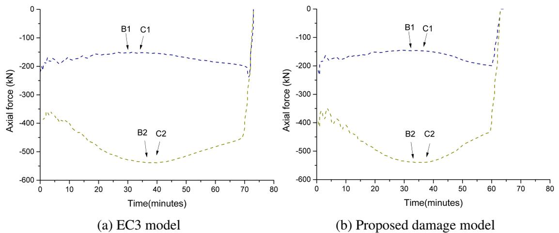
Fig. 5.72 Axial forces in columns during fire event
