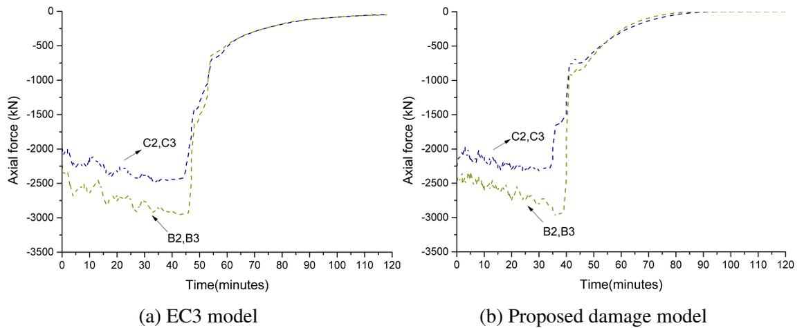
Fig. 5.80 Axial forces in columns during fire event
