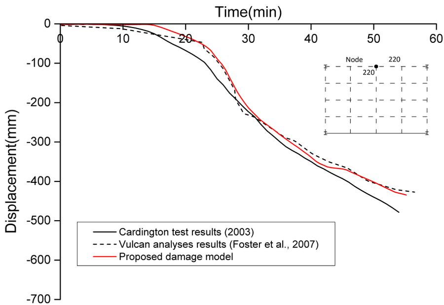
Fig. 4.54 Comparison of displacements at nodes 220 between numerical cases and test
