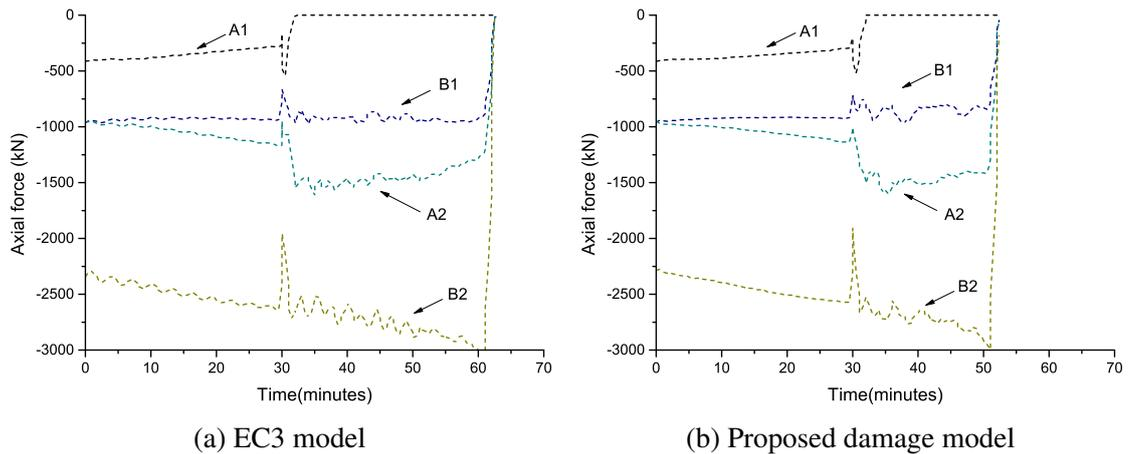
Fig. 5.89 Axial forces in columns during fire event
