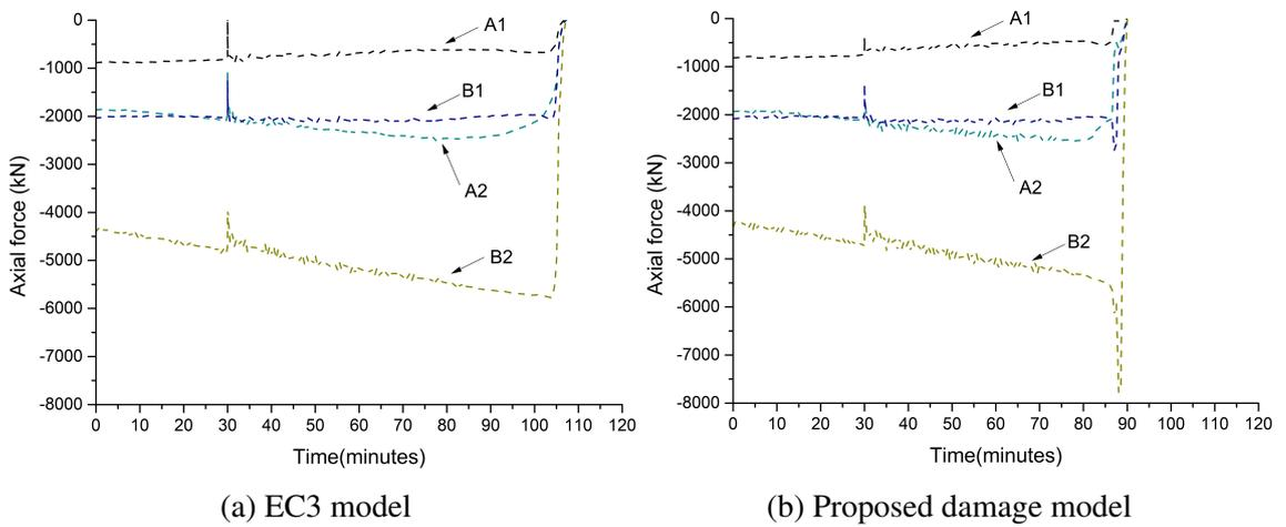
Fig. 5.93 Axial forces in columns during fire event
