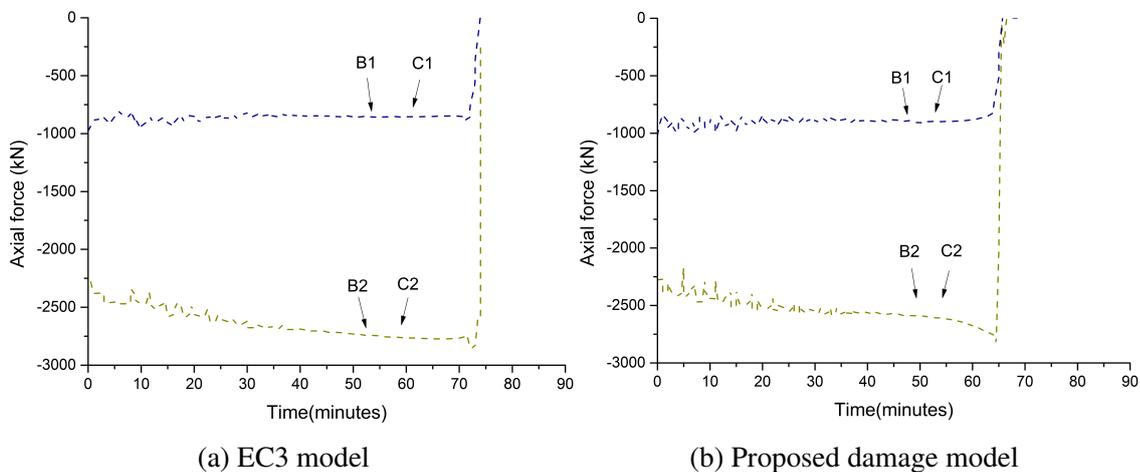
Fig. 5.59 Axial forces in columns during fire event
