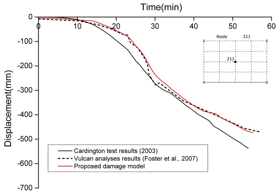
Fig. 4.52 Comparison of displacements at nodes 211 between numerical cases and test of simulating responses of structural systems subjected to fire where the dynamic load transfer and tensile membrane mechanism are present.
