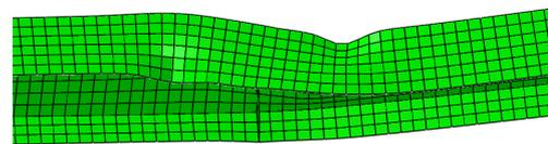
(a) Local and lateral torsional buckling observed in test (Dharma and Tan, 2007)
