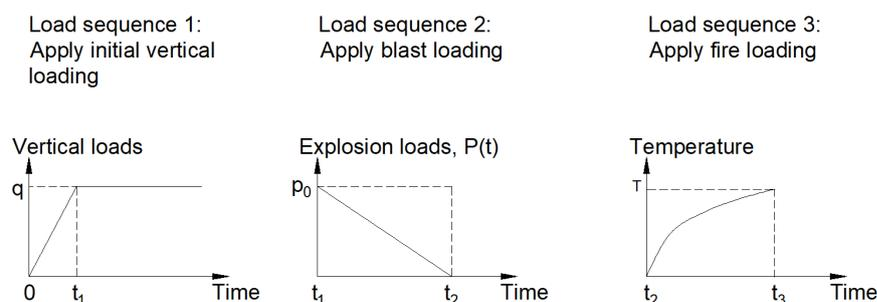
Fig. 5.8 Load sequences in post-blast fire analysis
