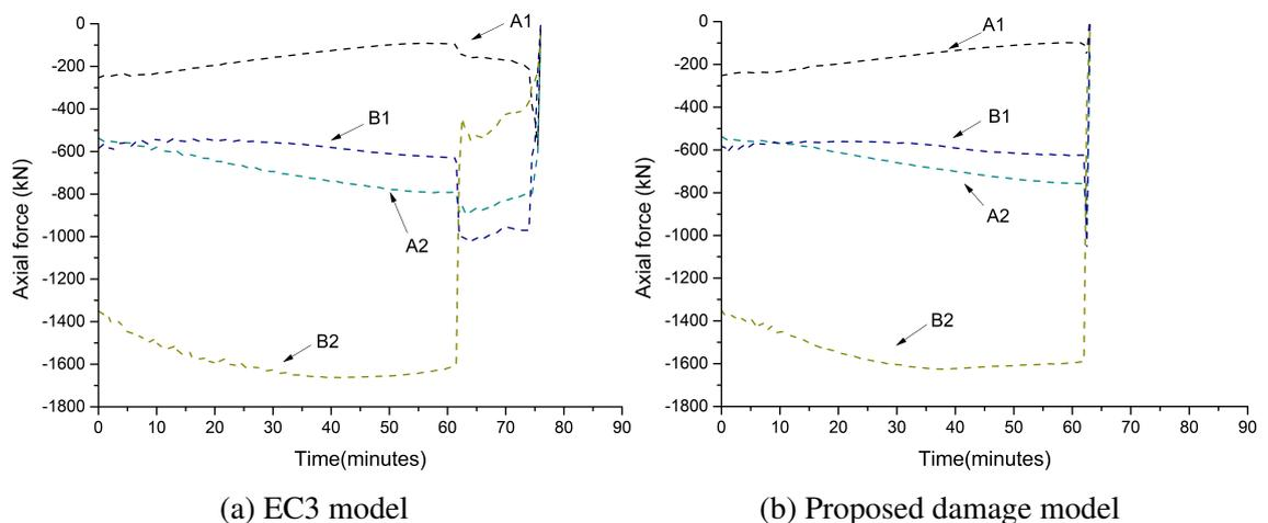
Fig. 5.22 Axial forces in columns during fire event
