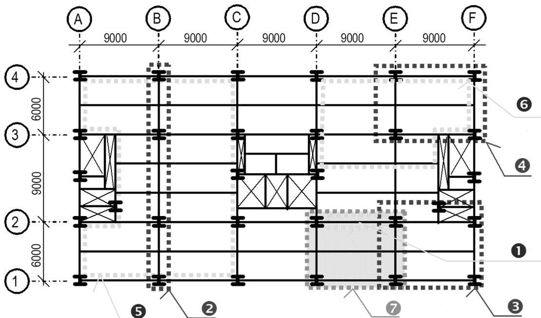
Fig. 2.4 Floor layout and location of the fire tests (Foster et al., 2007)
