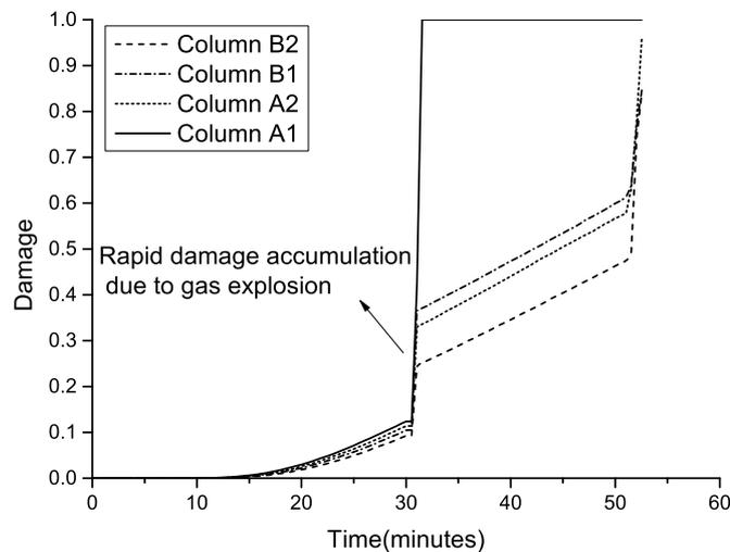
Fig. 5.90 Damage development in the top of blast-damaged columns
