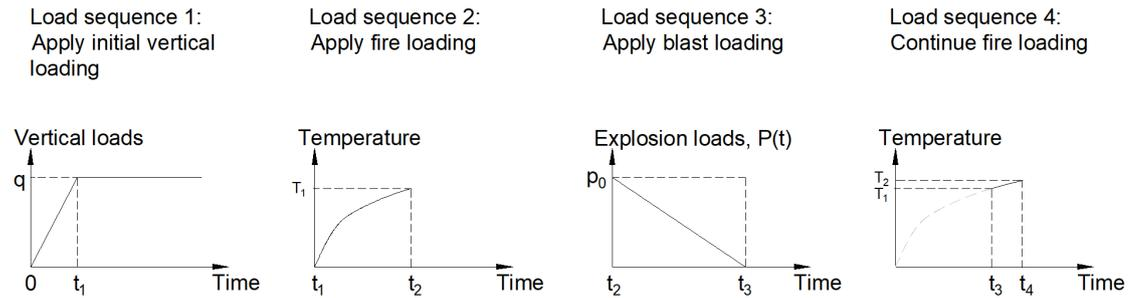
Fig. 5.10 Load sequences in fire and gas explosion analysis
