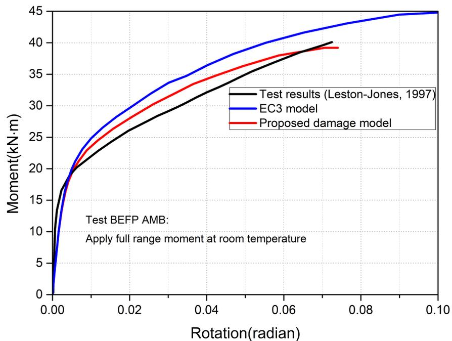
Fig. 4.11 Comparison of ambient-temperature connection response between numerical cases and test data
