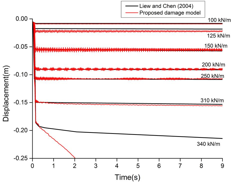
Fig. 4.31 Responses of steel frame under explosion only
