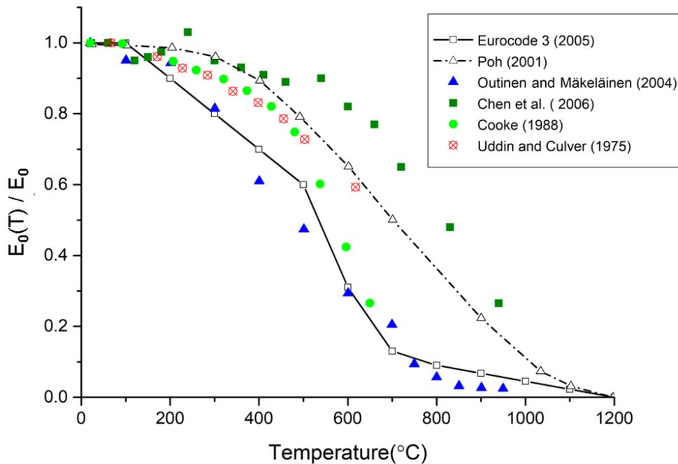
Fig. 2.6 Normalized elastic modulus of steel reported in literature sources
