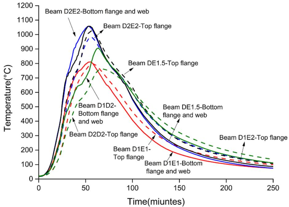
Fig. 4.46 Measured temperature distributions of beams (Lennon, 2003)
