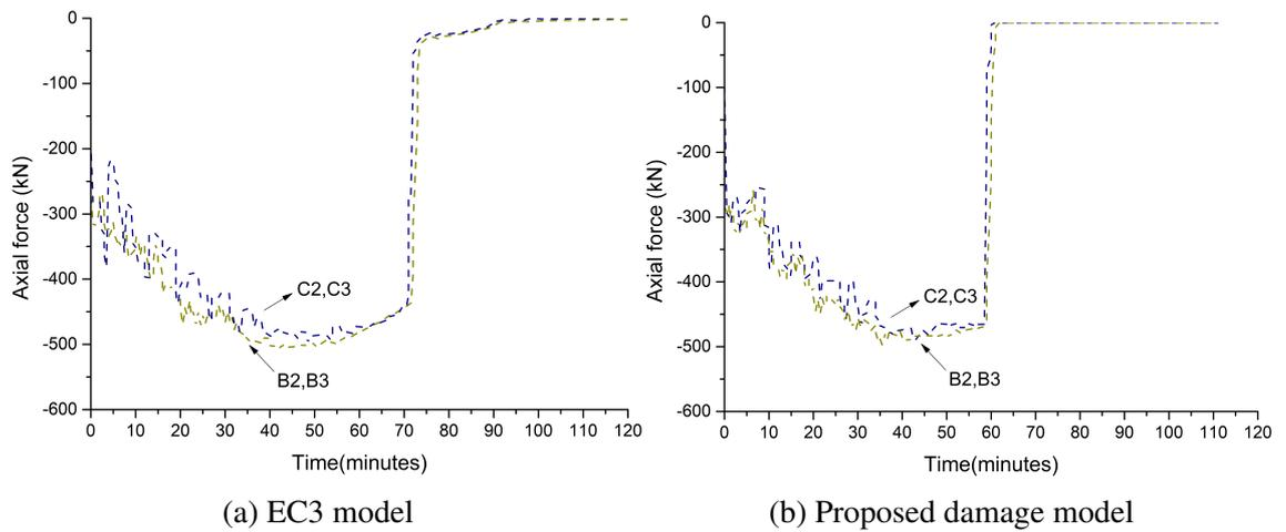
Fig. 5.86 Axial forces in columns during fire event
