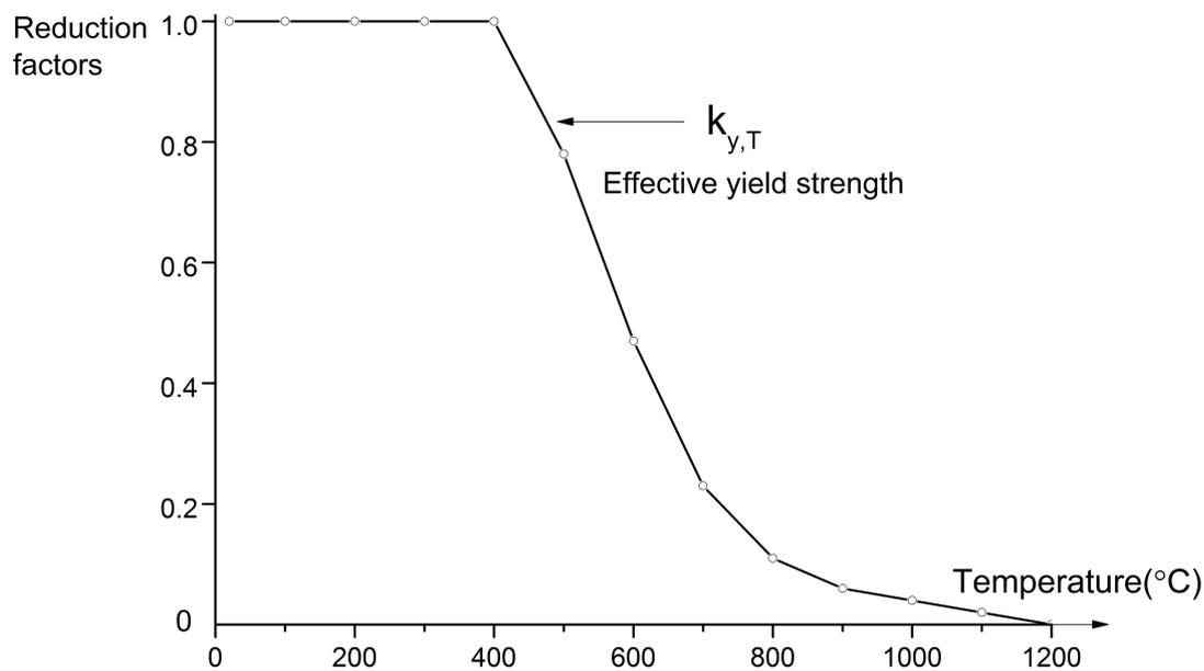
Fig. 3.4 Reduction factors for effective yield strength of structural steel at elevated temperatures (EN 1993-1-2, 2005)
