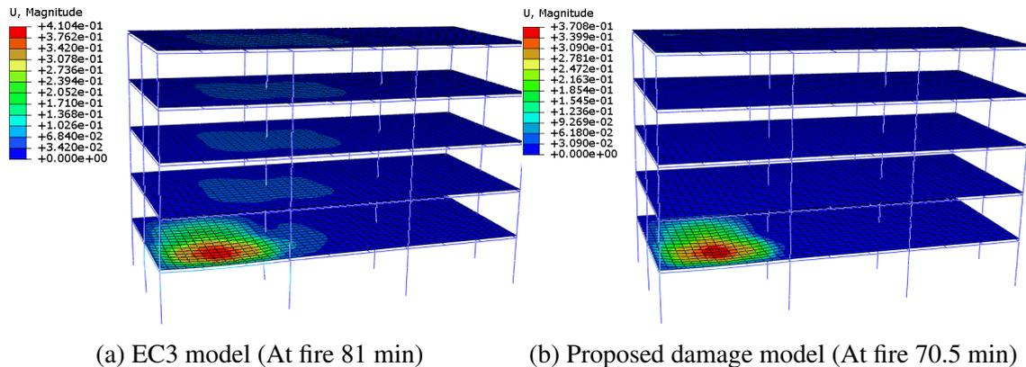
Fig. 5.13 The deformed shape of the building before column buckling initiates
