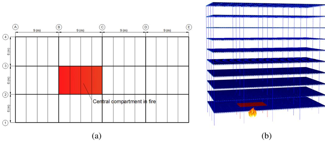
Fig. 5.38 Location of the central compartment fire on the ground floor
