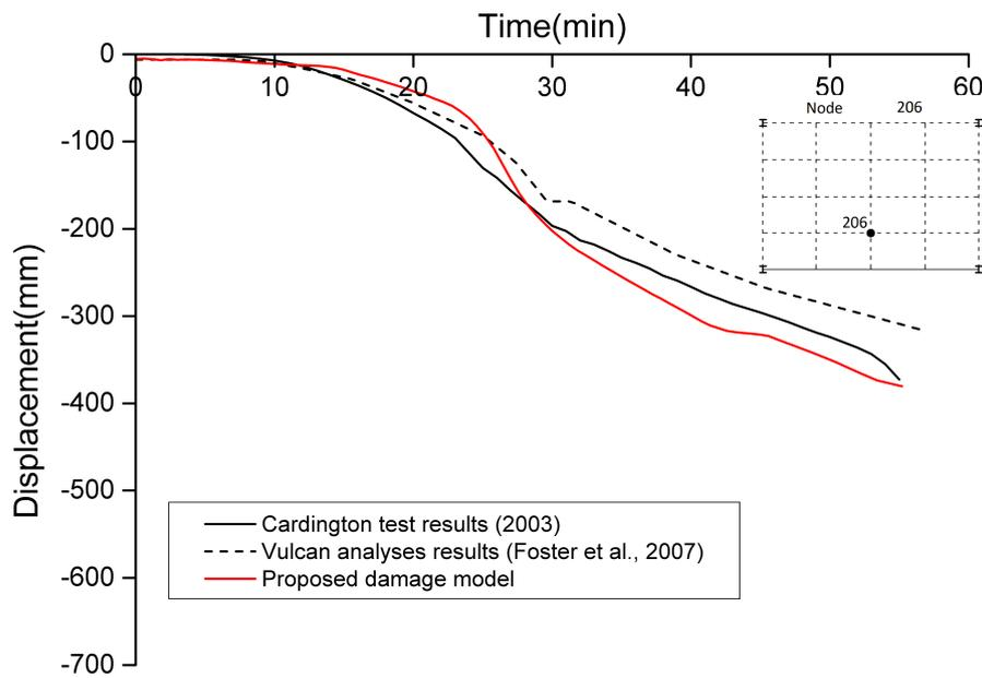
Fig. 4.51 Comparison of displacements at nodes 206 between numerical cases and test
