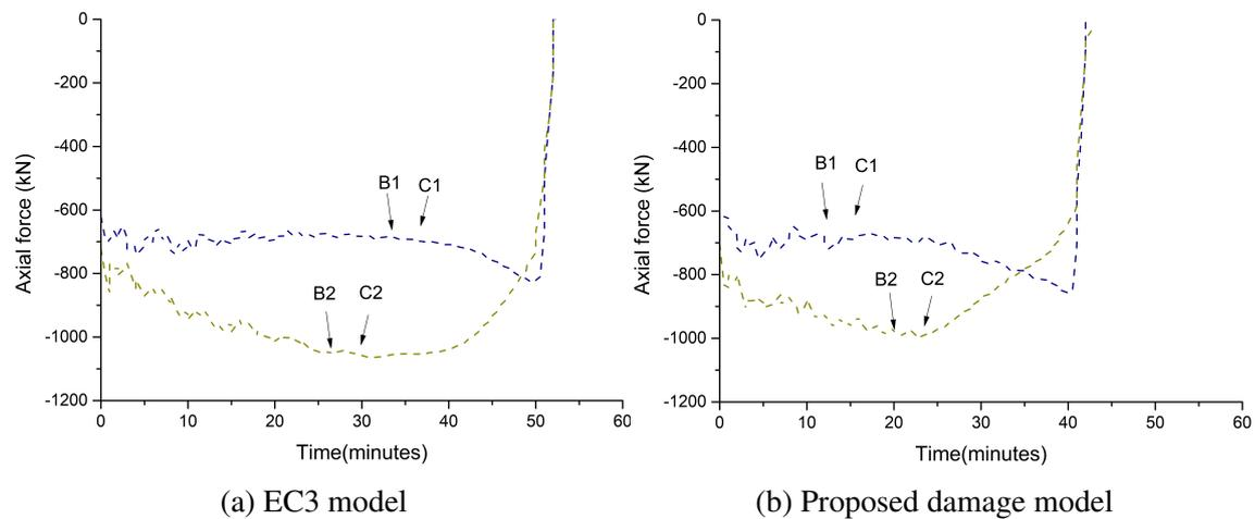
Fig. 5.66 Axial forces in columns during fire event
