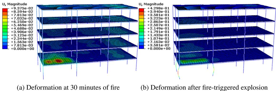
Fig. 5.87 Deformation before and after fire-triggered explosion occurrence
