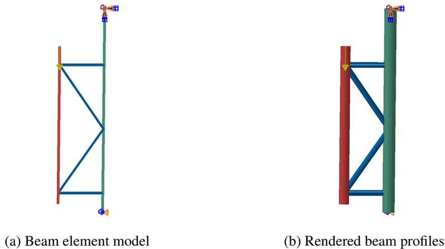
Fig. 4.22 Numerical model of steel tubular truss in ABAQUS
