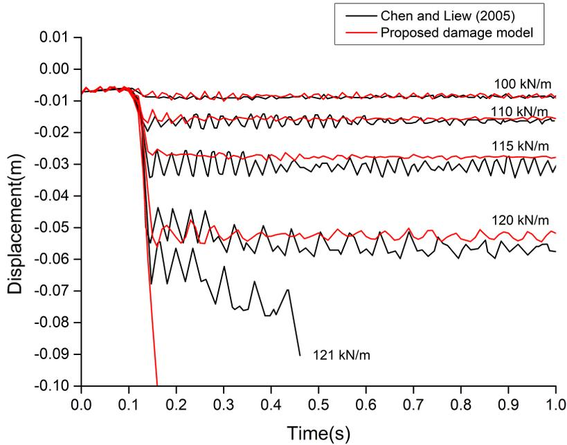
Fig. 4.37 Responses of steel frame under explosion only
