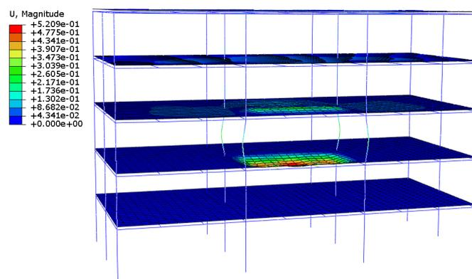
Fig. 5.64 Blast induced deformation after the blast analysis in the central compartment on the third floor
