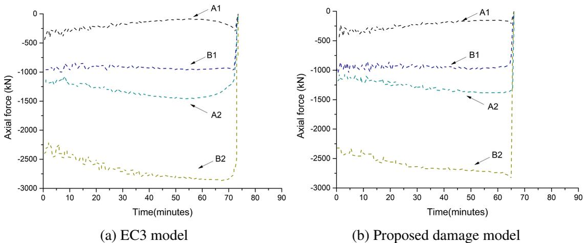
Fig. 5.55 Axial forces in columns during fire event
