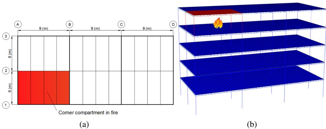
Fig. 5.27 Location of the corner compartment fire on the top floor
