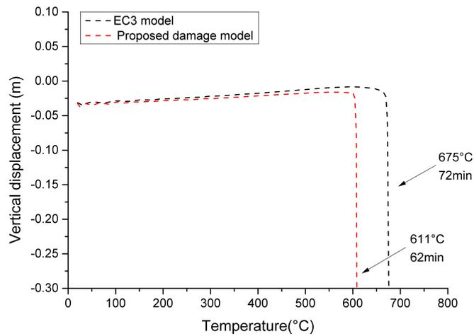
Fig. 5.71 Vertical displacement of the heated interior column
