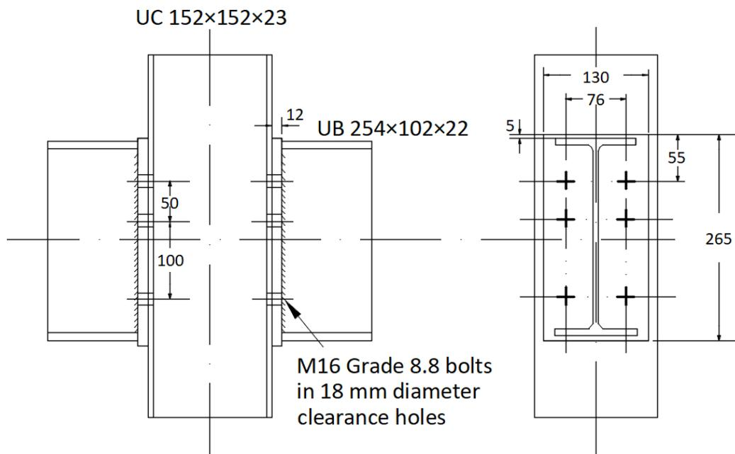
Fig. 4.8 Flush end plate connection detail (Leston-Jones, 1997)
