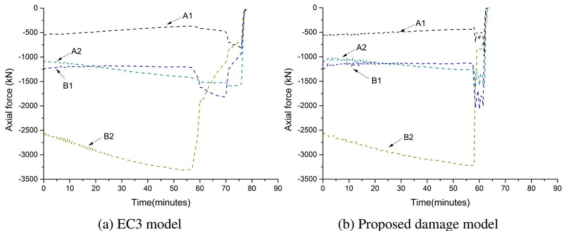
Fig. 5.43 Axial forces in columns during fire event
