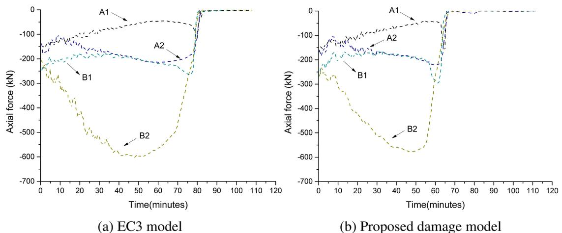
Fig. 5.83 Axial forces in columns during fire event
