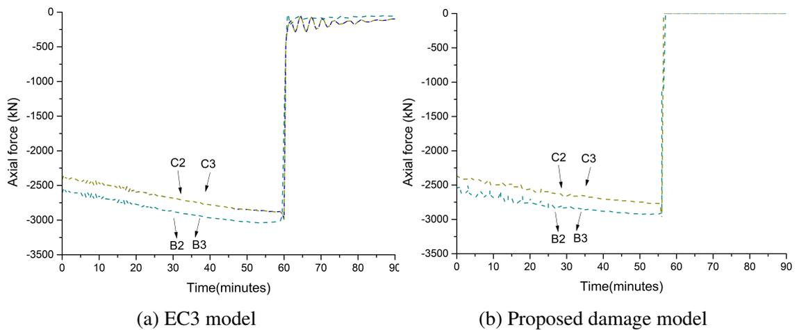
Fig. 5.46 Axial forces in columns during fire event
