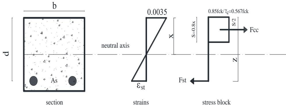
Figure B.0.2 Illustration of strain and rectangular stress diagrams of reinforced concrete beam under ultimate bending moment
