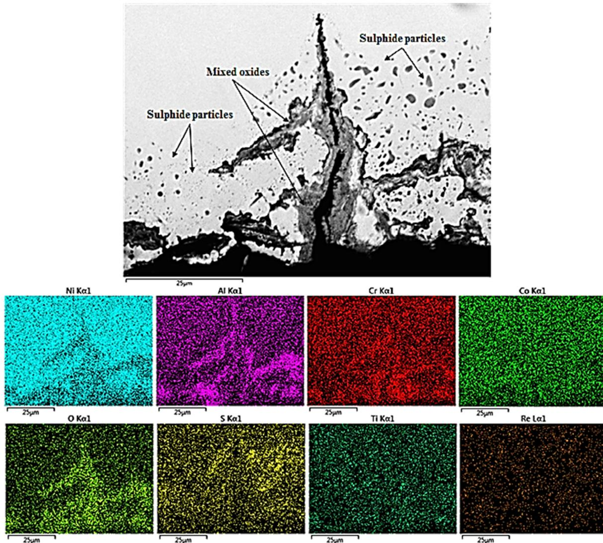
**Fig. 8.** Backscattered electron image of a typical sulphidation cracking found under a tested specimen (LTD set A). Also shown is the element mapping of main mixed oxides and sulphur compounds detected by the EDX analyser.
