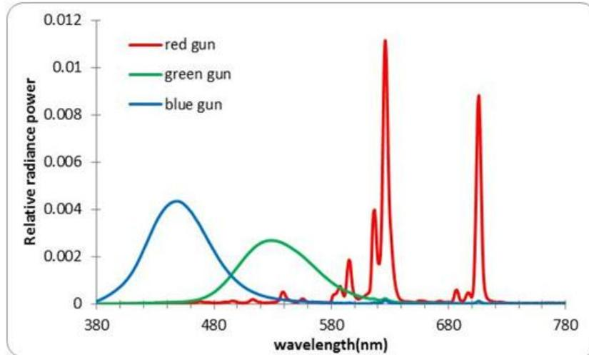
Figure 3-8. The QAA spectral radiance scan results.
