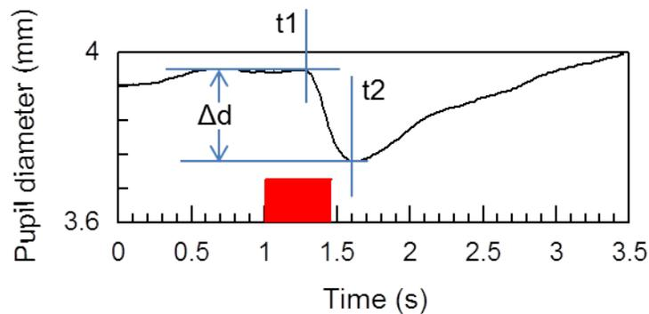
Figure 4-20. Example of pupil response diagram showing how the pupil response amplitude was extracted.
