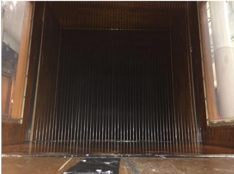
**Figure 3.38:** Turbulence generating grid mounted vertically in the wind tunnel.
