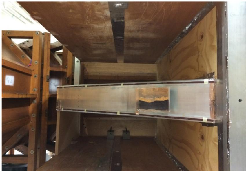
**Figure 3.11:** Front view of the model mounted in the Gaster wind tunnel with the device to prevent contamination.
