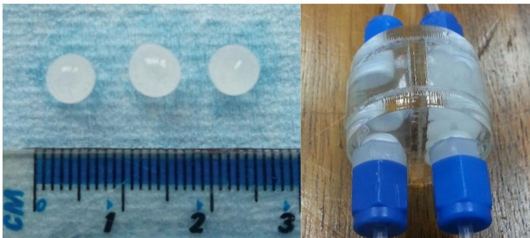
**FIGURE 1** Left: Alginate spheres with microbubbles appear milky and the size is approximately 5 mm. Right: Twin-compartment sample holder containing both preparations of alginate spheres in water suspension, equipped with Swagelok (Solon, OH) connectors, enabling the pressure being applied into the system to be changed
