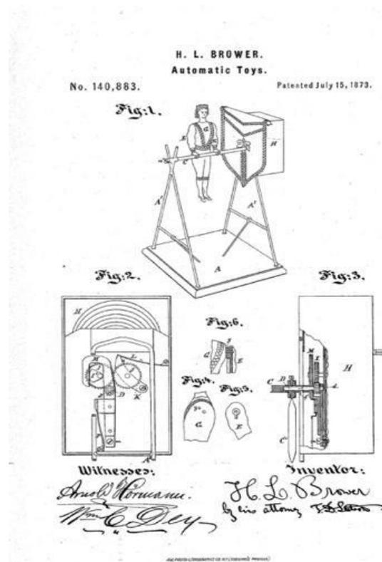
Image Description: A patent drawing of a small figure attached by a string to two wooden sticks, which when squeezed force the figure to spin around on the string. The drawing includes the text, “H. L. Brower. Automatic Toys. No. 140,883. Patented July 15, 1873. Witness [signature of two witnesses] and Inventor [signature of two inventors]”. This version includes a more stable base, and a widening mechanism.
