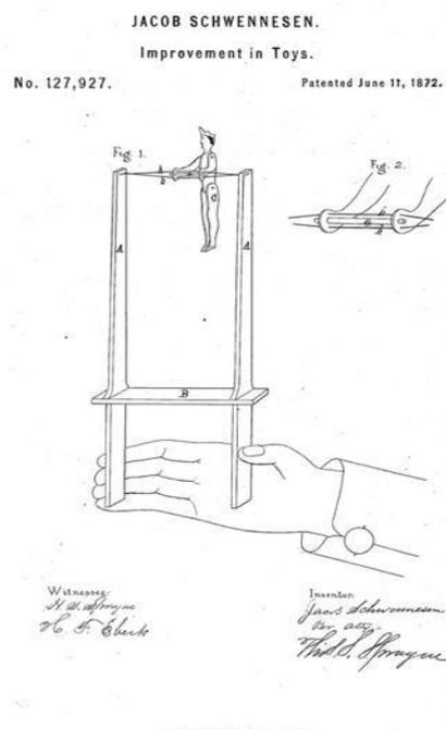
Image Description: A patent drawing of a small figure attached by a string to two wooden sticks, which when squeezed force the figure to spin around on the string. The drawing includes the text, “JACOB SCHWENNESEN. Improvement in Toys. No. 127, 927. Patented June 11, 1872. Witness [signature of two witnesses] and Inventor [signature of three inventors].”
