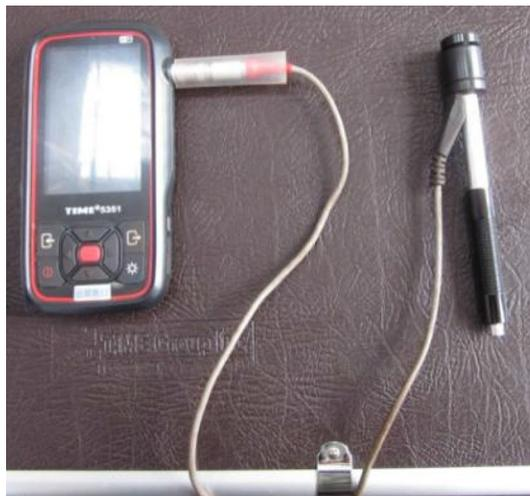
**Figure 5. TIME5351 Leeb hardness tester.**
