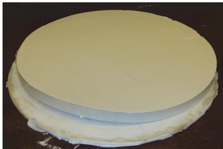
Figure 4.25 Excess soil trimmed with wire cutter.
