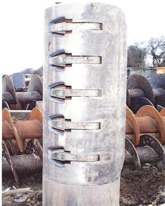
Figure 2.12 Expanded Piling construction issue rib cutting tool.
