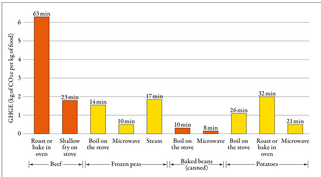
Figure 4. GHGE (kg of CO<sub>2</sub>e per kg of food) of different foods, showing the relationship of various preparation techniques and the average cooking times used in the UK, from Frankowska et al., (2019)
