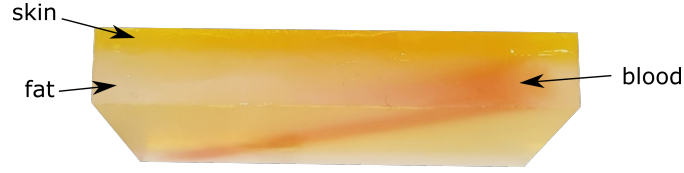
Figure 3.7: DRE gelatin phantom comprising skin (yellow), fat (white) and blood vessel (red)
