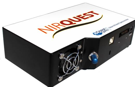
**Figure 3.9:** The NIRQuest 512 spectrometer, from Ocean Optics (*Largo, FL, USA*). Picture taken from <sup>154</sup>.
