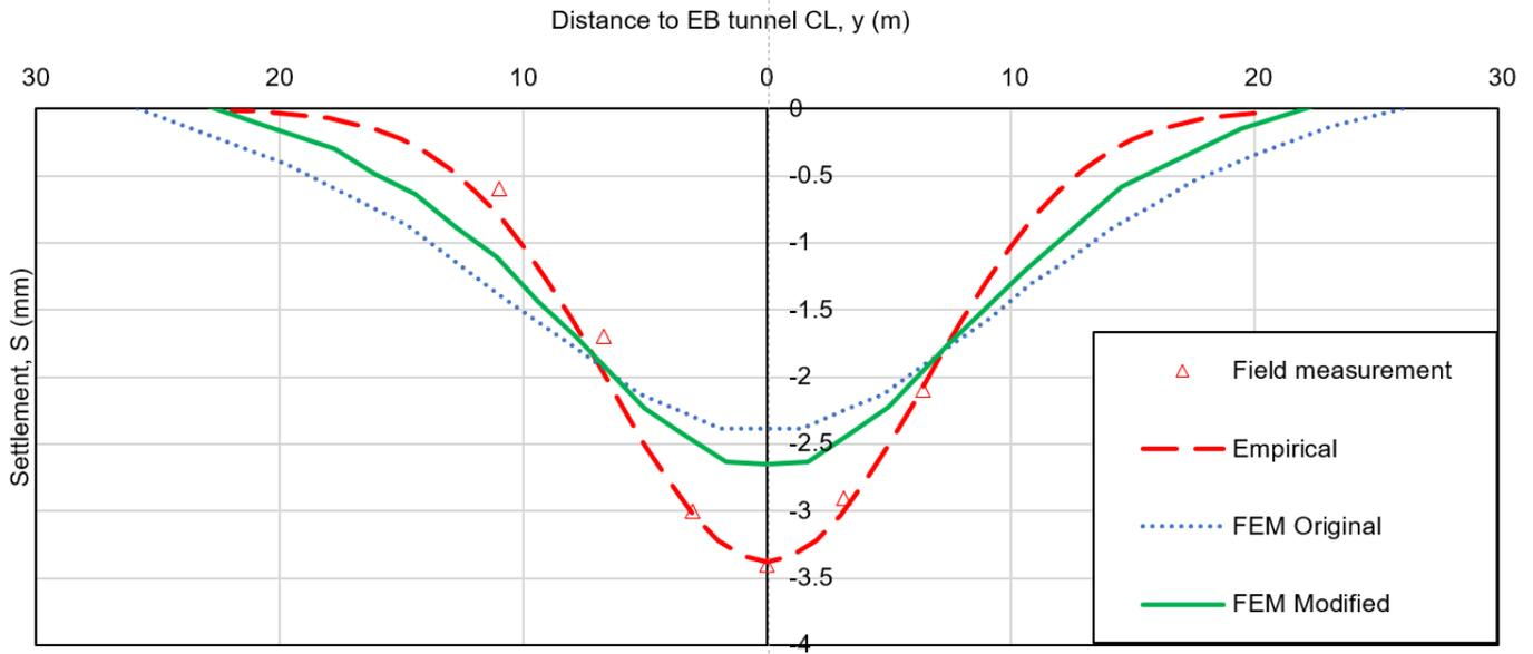
Figure 7. Ground surface settlement after EB tunnel construction.
