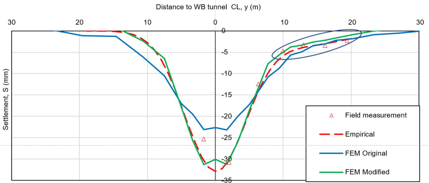
Figure 8. Ground surface settlement after WB tunnel construction.
