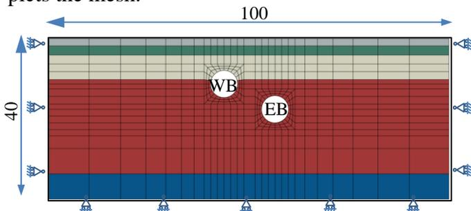
Figure 5. Finite element model in Abaqus.
