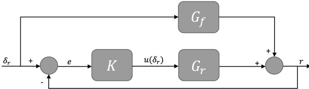
Figure 3.2: 4WS vehicle closed-loop control system[2]
