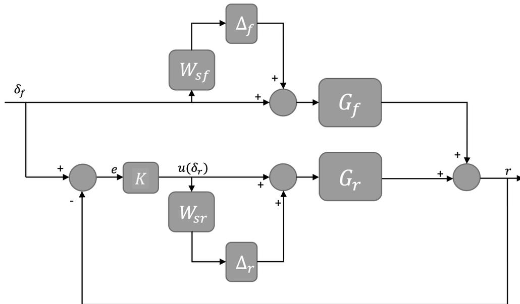
Figure 3.3: 4WS vehicle closed-loop control system in  $\mu$  framework[2]
