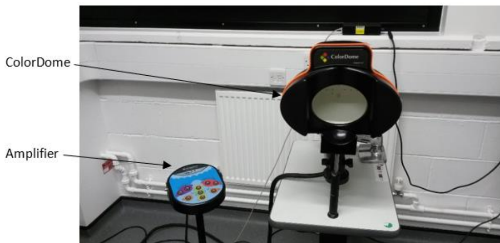
Figure 3.2. Ganzfeld ColorDome stimulator and amplifier.
