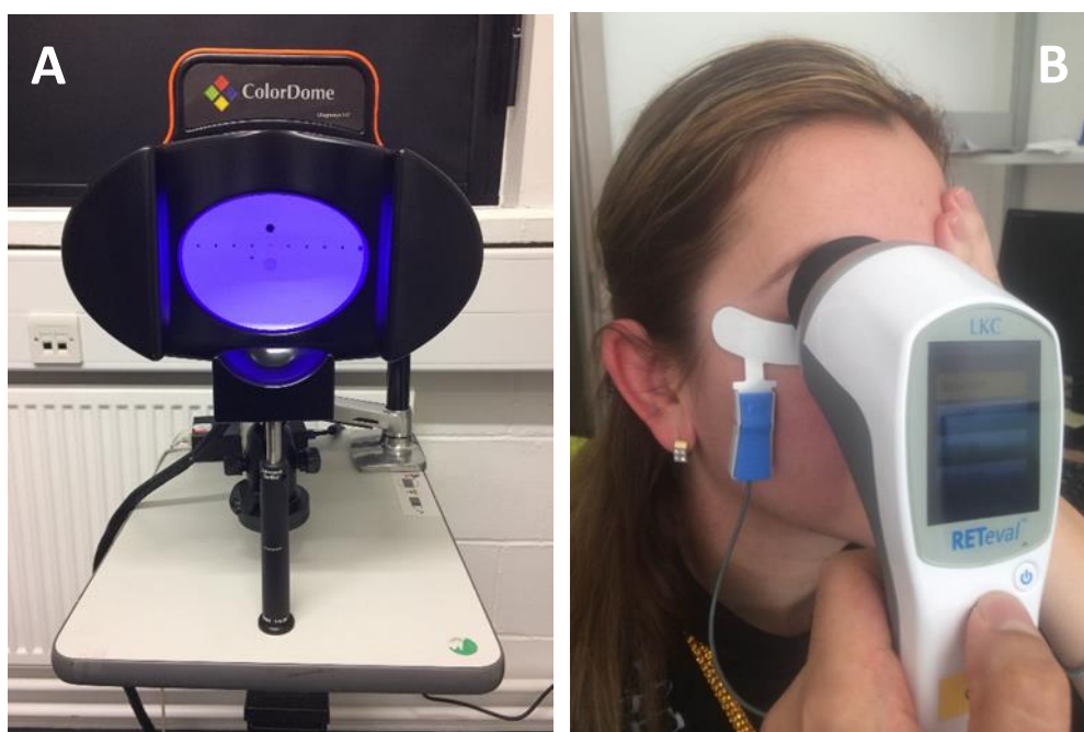
Figure 4.1. Images showing the two types of ERG stimulator device used in this study. A; ColorDome Ganzfeld stimulator by Diagnosys, Cambridge, UK. B; RETeval® ERG system by LKC Technologies, Inc., Gaithersburg, MD, USA.
