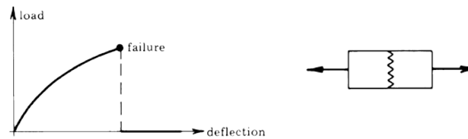
(a) Perfectly brittle failure element
