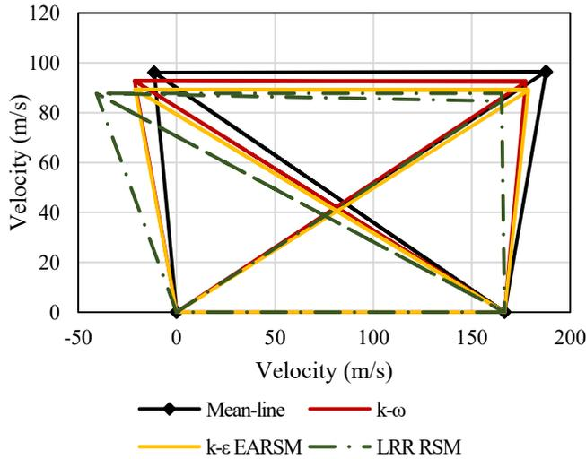
FIGURE 11 VELOCITY TRIANGLES FOR DIFFERENT TURBULENCE MODELS
