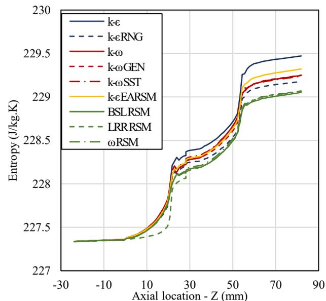
FIGURE 17 COMPARISON OF THE ENTROPY FROM INLET TO OUTLET FOR DIFFERENT TURBULENCE MODELS
