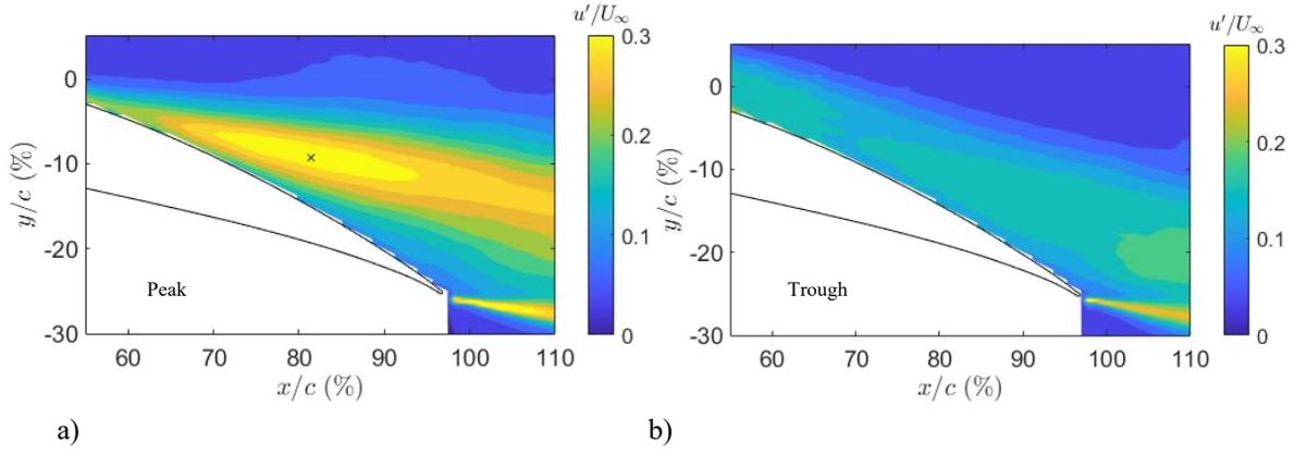
**Fig. 17** Colour contours of the turbulence intensity  $u'/U_\infty$  downstream of the LEU peak (a) and the trough (b) of an optimized LEU profile ( $\lambda 30h6$ ) at  $\alpha = 15.3^\circ$  with grid.
