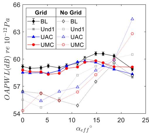
**Fig. 8 Overall sound-power level variations with the attack angle of the aerofoils. The amplitude and the wavelength of the LE undulation are 6 mm ( $h/c = 6\%$ ) and 20 mm ( $\lambda/c = 20\%$ ), respectively.**
