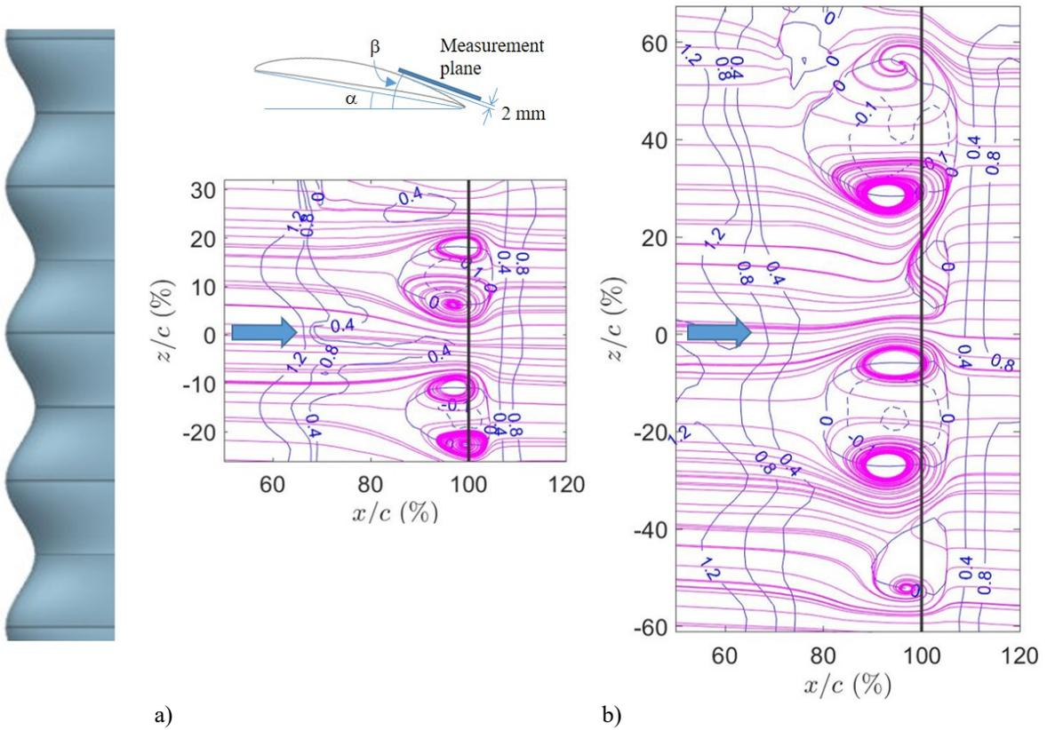
**Fig. 16 Time-averaged streamlines (in pink) and  $\bar{U}/U_\infty$  contours (in blue) for  $\alpha = 10.8^\circ$  with  $\beta = 23^\circ$  (a) and  $\alpha = 15.3^\circ$  with  $\beta = 35^\circ$  (b).**
