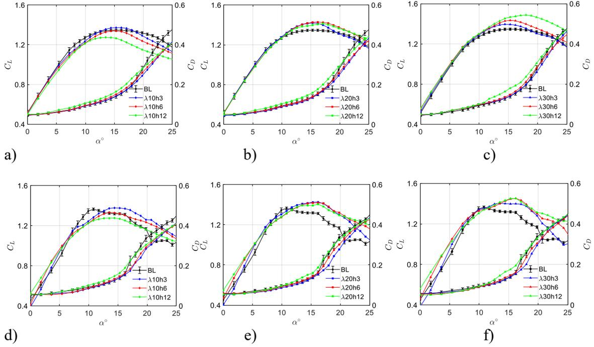
**Fig. 11**  $C_L$  and  $C_D$  of UMC leading-edge profile with various  $h$  and  $\lambda$  against  $\alpha$ : (a), (b) and (c) with grid; (d), (e) and (f) without grid. The baseline data are also shown for comparison. The legends in the figure represent the percentage value of each parameter, e.g.,  $\lambda 10h3$  indicates a LEU with 10%  $\lambda/c$  and 3%  $h/c$ .
