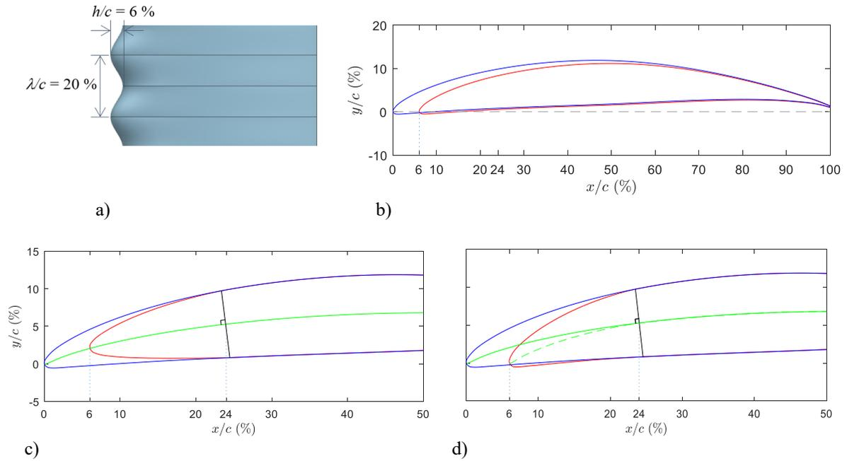
**Fig. 6** Definition of the amplitude and wavelength of the leading-edge undulation (a), and the profiles of Und1 (b), UAC (c) and UMC (d) showing camber lines at the peak (blue) and trough (red) sections.
