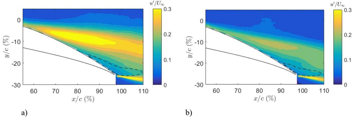
**Fig. 19** Colour contours of the turbulence intensity  $u'/U_\infty$  downstream of the LEU peak at  $0 < tU_\infty/c < 20$  and  $120 < tU_\infty/c < 165$  (a) and at  $20 < tU_\infty/c < 120$  (b) of an optimized LEU profile ( $\lambda 30/h6$ ) at  $\alpha = 15.3^\circ$  with grid. The dotted lines indicate the region of flow separation with negative velocity.
