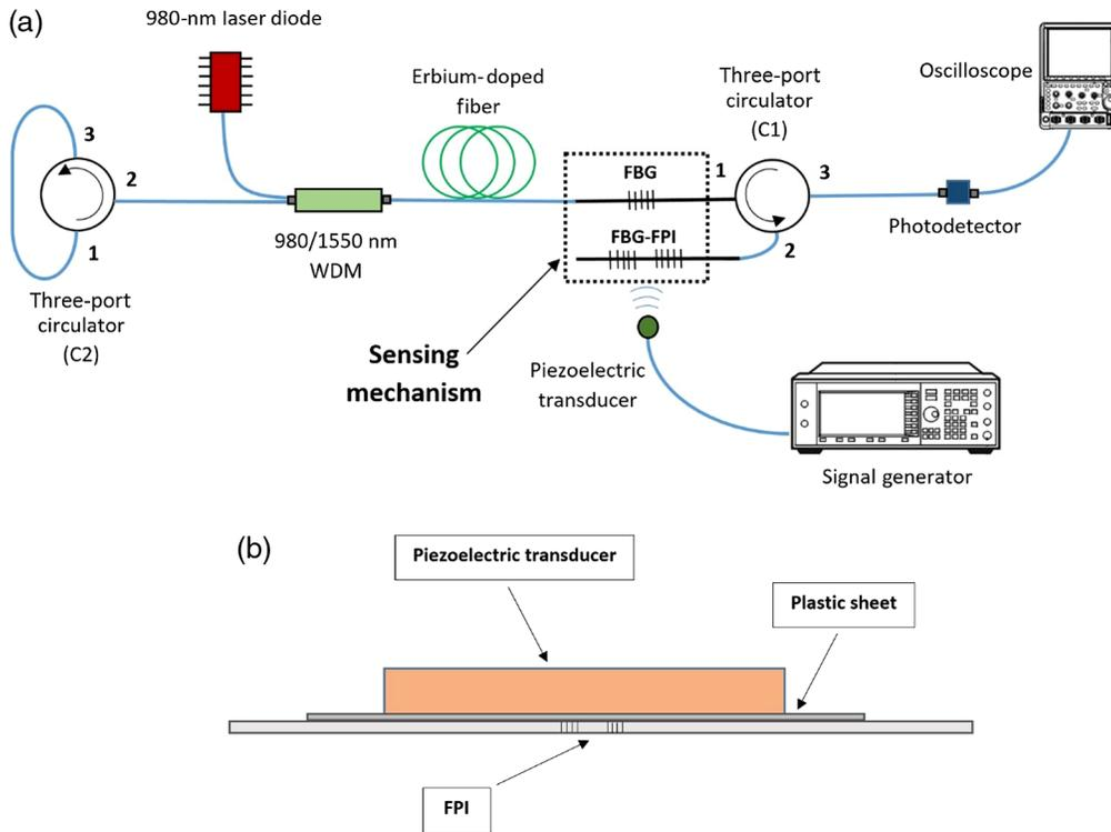
**Fig. 3** Illustration of the (a) experimental setup for verifying the performance of the FBG-FPI cavity subjected to a simulated seismic-induced vibration and (b) a closer look from the side view of the signal transfer setup at the FBG-FPI.
