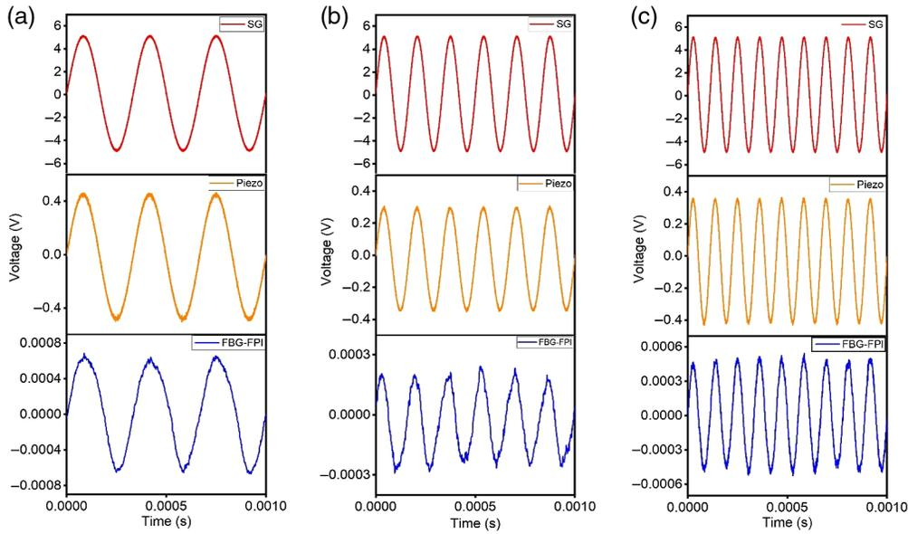
**Fig. 9** Output signal comparison between the SG (SG—in red), the piezoelectric sensor (Piezo—in orange), and the FBG-FPI sensor (FBG-FPI in blue) for three different frequencies (a) 3, (b) 6, and (c) 9 kHz.
