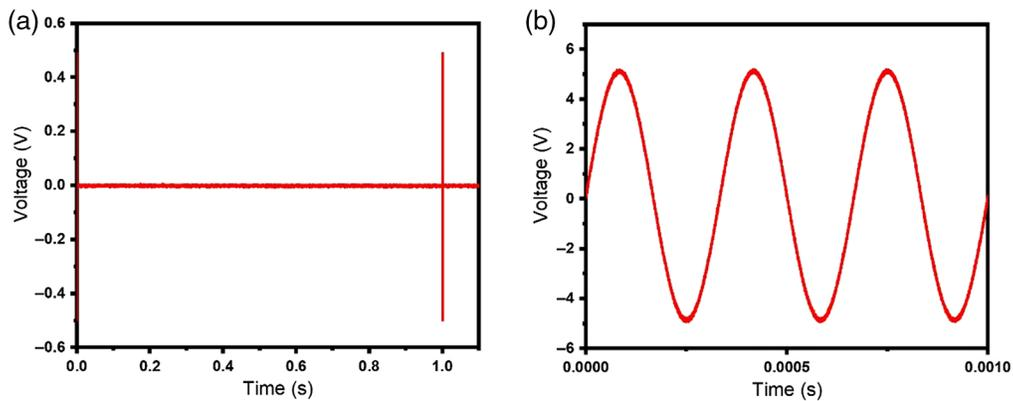
**Fig. 6** (a) Signals directly from the SG: 3-kHz burst at a 1-Hz interval and (b) 3-kHz sine wave, generated by the SG.
