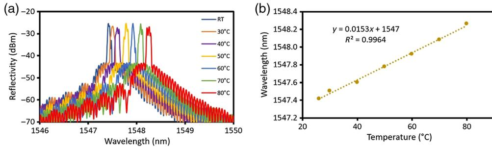
**Fig. 10** (a) Output spectra of the FBG-FPI when subjected to different temperatures and (b) the linear response of the FBG-FPI when it is subjected to different temperatures from 26°C to 80°C in 10°C intervals.
