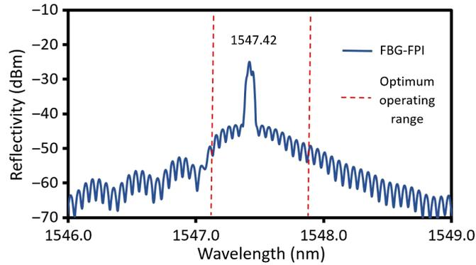
**Fig. 4** The output spectrum of FBG and FBG-FPI from port 3 of the circulator when connected to an OSA.
