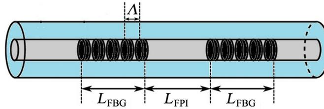
**Fig. 1** Illustration of the FBG-FPI fabricated in this work where  $L_{\text{FBG}}$  is the length of the grating used (of period  $\Lambda$ ) and  $L_{\text{FPI}}$  is the separation of the gratings, and thus the interferometric cavity length.
