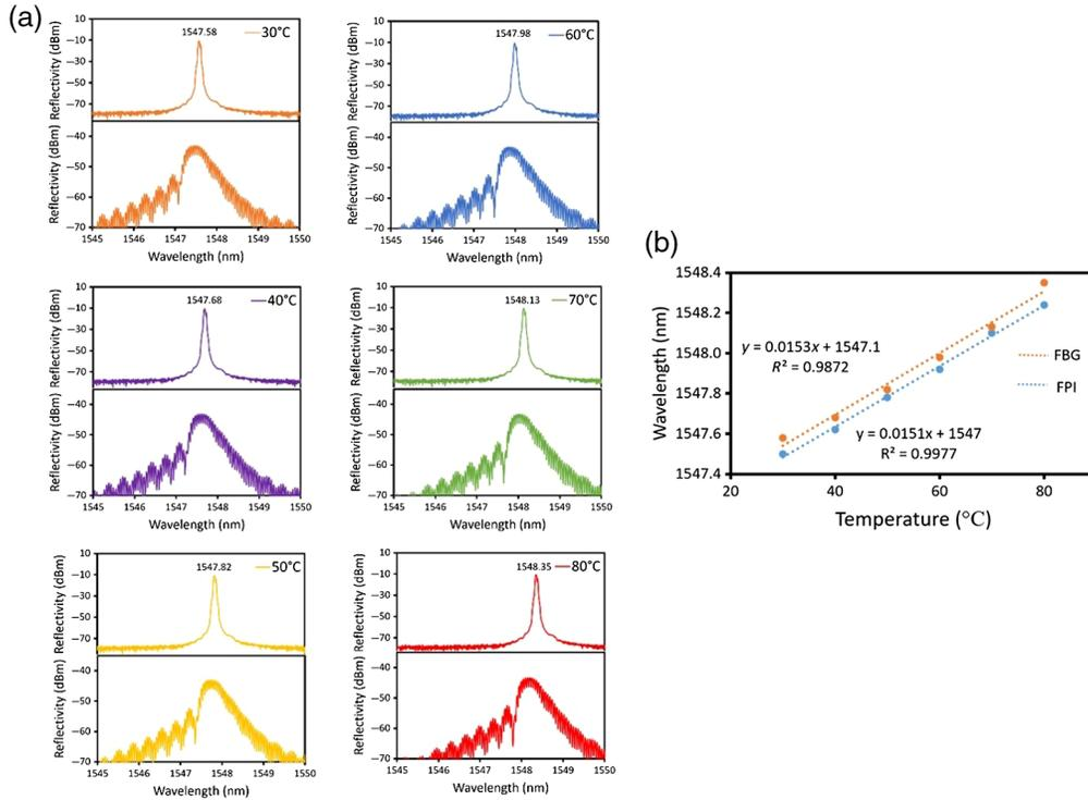
**Fig. 11** (a) Response spectra of each FBG and FPI at 30°C, 40°C, 50°C, 60°C, 70°C, and 80°C and (b) the linear relationship for both FBG and FBG-FPI simultaneously when they were subjected to different temperature parameters.
