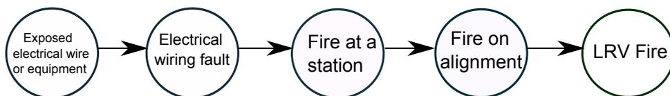
Figure 9.11: Hazard path for "LRV Fire"
