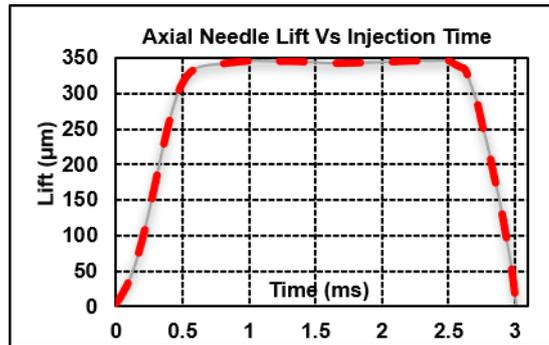
Figure 6. 2. Needle motion of the injector.
