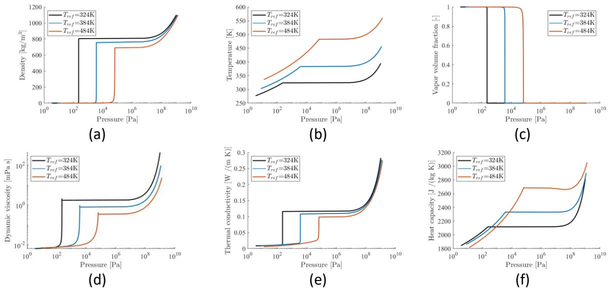
Figure 5. 2. Thermodynamic data following an isentropic expansion of the Diesel surrogate. Three cases are shown depending on the reference temperature at 5MPa: (i) 324K for the
