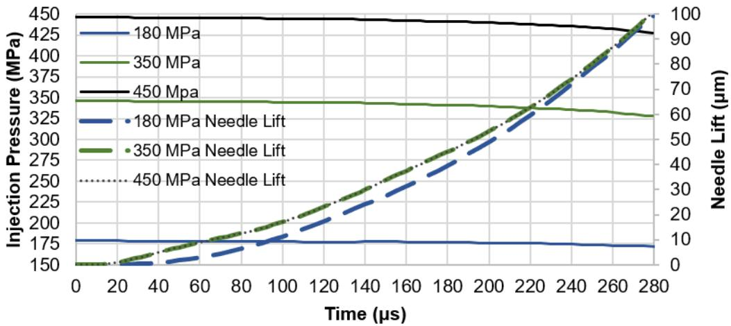
Figure 4. 2. Injection pressure and needle lift profile utilised as boundary conditions until 100µm needle lift.
