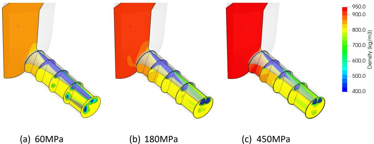
Figure 5. 4. Predicted time-averaged density on different slices at the sac volume and orifice for three injection pressures. Thermal effects are considered. The iso-surface for vapor volume fraction of 50% is included, which shows two coherent structures separated at the midplane for (b) and (c).
