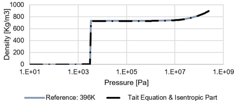
Figure 3. 4. Utilised density variation with pressure, as predicted by the relevant barotropic fluid EoS.
