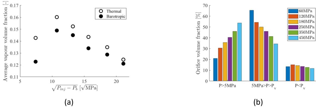
Figure 5. 12. (a) Time-averaged vapor volume fraction inside the injector orifice versus the square root of the pressure drop estimated utilising both the barotropic and thermal models. (b) Orifice volume fraction histogram for different pressure ranges inside the orifice volume when thermal effects are considered.
