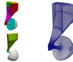
Figure 6. 4. Computational Volume of the 1/5th of injector.
