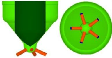
Figure 6. 3. Different views of the Diesel injector.
