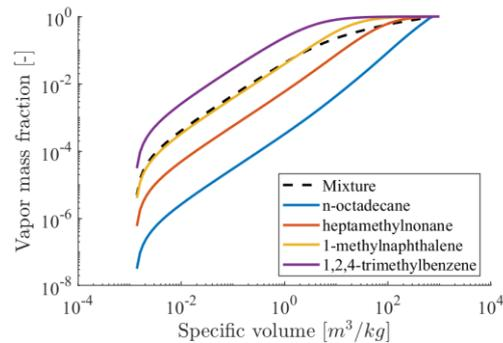
Figure 5. 17. Vapor mass fraction of representative components of the fuel surrogate (the heaviest, lightest and two intermediate) as a function of specific volume for a OD expansion of the fuel at 350K.
