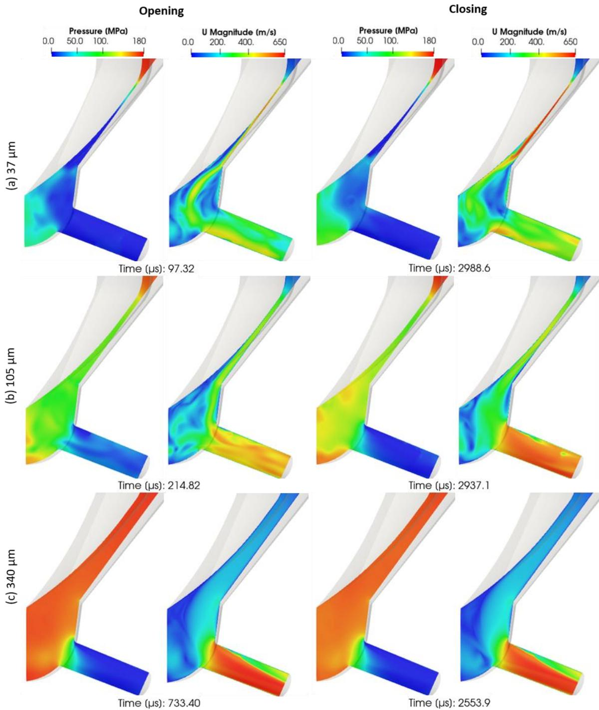
Figure 3. 14. Snapshots of instantaneous pressure and velocity magnitude at time instances corresponding to (a) 37 μm, (b) 105 μm and (c) 340 μm.
