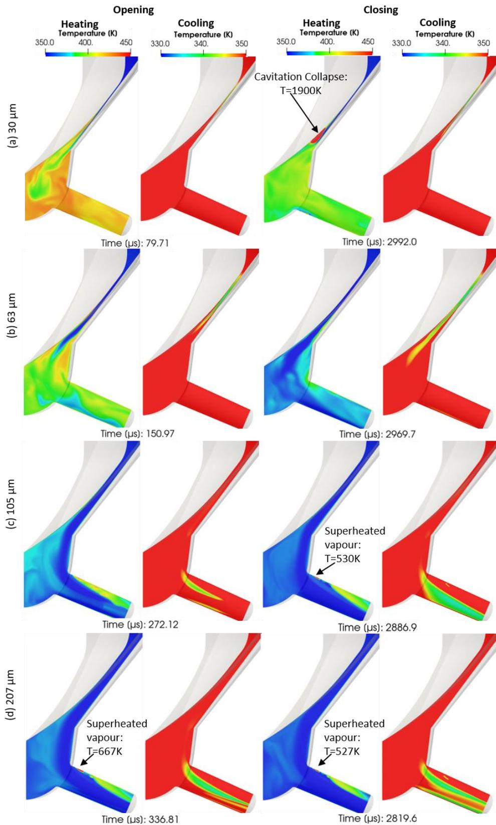
Figure 3. 15. Snapshots of instantaneous temperature field on the mid-plane of the injector. The time instants correspond to needle lifts (a) 30 μm, (b) 63 μm, (c), 150 μm and (d) 207 μm.
