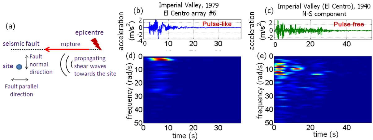
Figure 2. (a) Generation of forward directivity effects, (b),(c) Acceleration trace of a typical pulse-like and pulse-free ground motion, respectively, (d),(e) Harmonic wavelet based time-frequency representation of a typical pulse-like and pulse-free ground motion, respectively.
