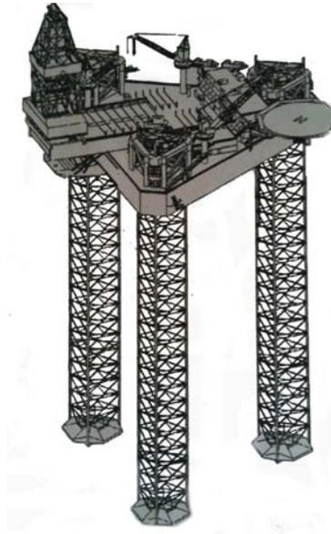
Figure 1. A typical three-legged Jack-Up platform (adopted from [1])
