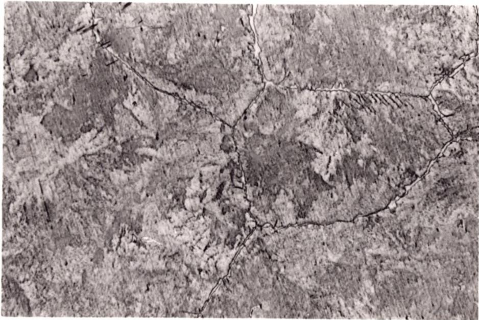
Fig. 10.13 High carbon steel tested at 670°C showing austenite grains with ferrite films surrounding the grains. (not quenched) 200 μm
