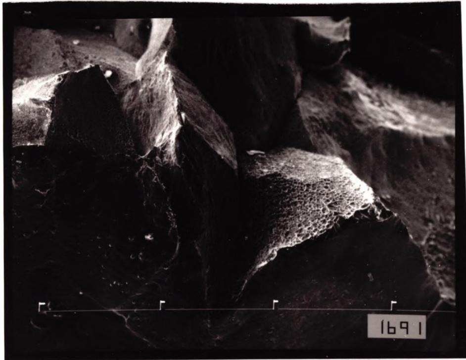
Fig. 6.9 Fracture surface of as-cast Ti steel, tested at 850°C, showing a mixture of inter granular microvoid coalescence and intergranular decohesion (R of A 47%).
