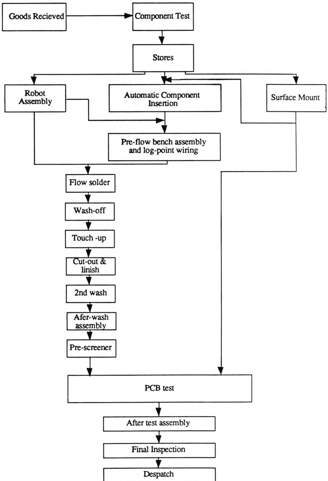
Figure A1.1 the manufacturing and testing process of PCB's
