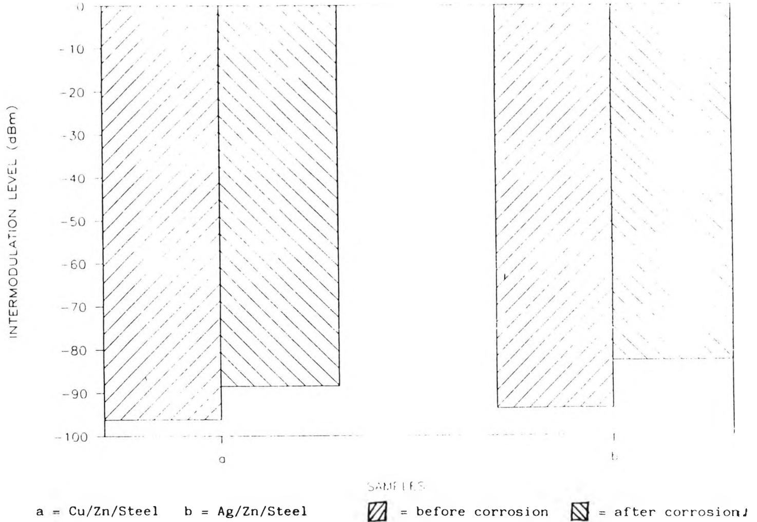
FIGURE 6.6 IMI of multi-layer metal-plated samples before and after corrosion
