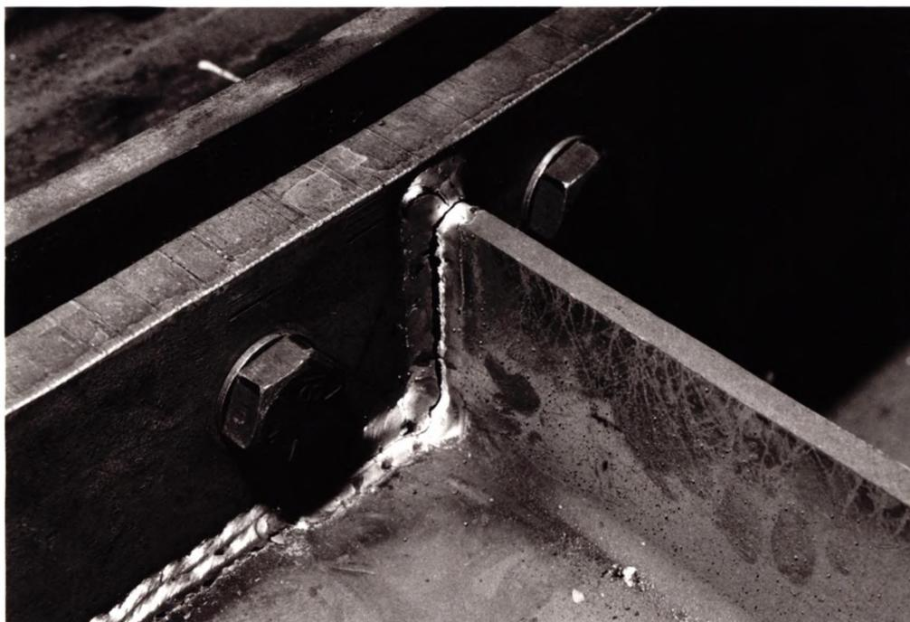
Figure 4.18 Beam Tension Flange Weld Failure (Test B1).
