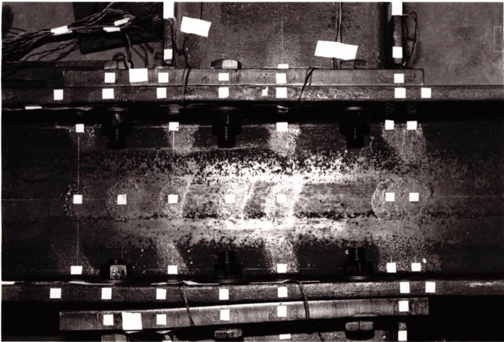
Figure 4.10 Deformation of Endplate at Failure (Test A1).
