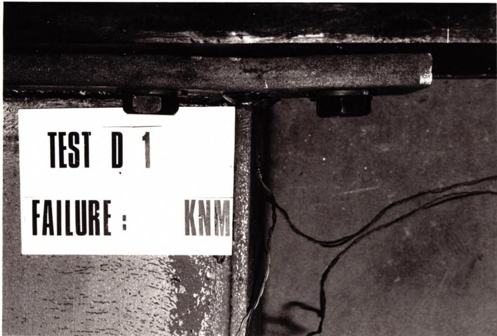
Figure 4.22 Endplate Deflection at Failure (Test D1).
