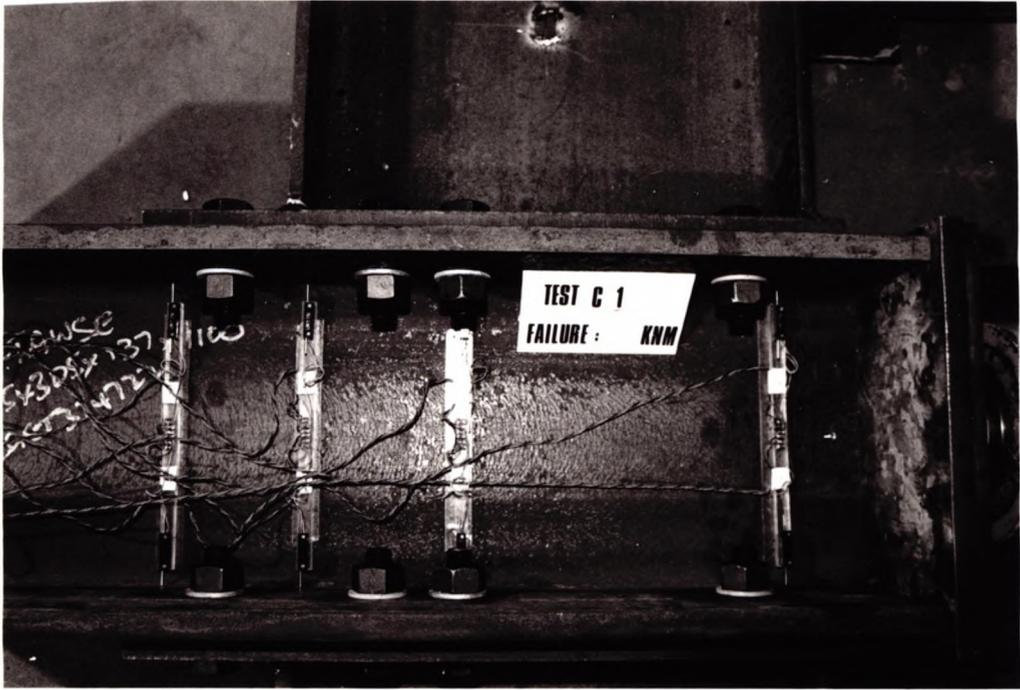
Figure 4.21 Proximity of Endplate to Specimen End (Test C1).
