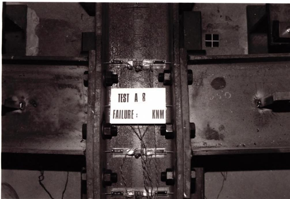
Figure 4.17 Deflection of Test A8 at Failure.
