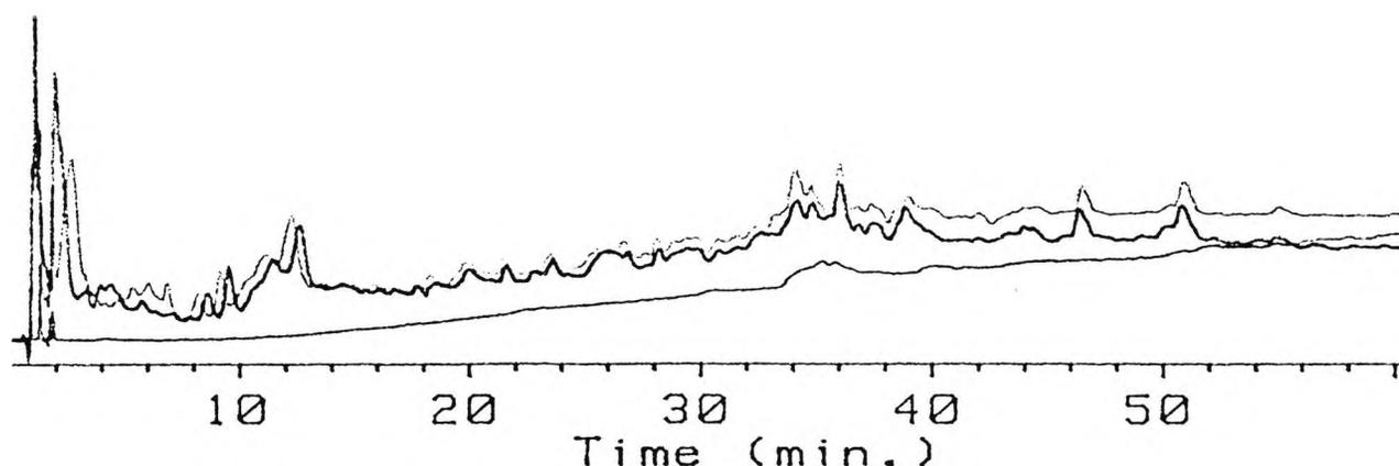
Figure 5-5. Reproducibility of continuous gradient elution profile of TW405 and comparison with a blank run, on a 25 x 0.45 cm Spherisorb-ODS1 5  $\mu$ m, with a continuous gradient elution from 10:10:80 MeCN/MeOH/H<sub>2</sub>O to 50:50 MeCN/MeOH using a 100 ml mixing flask at 2 ml/min and monitored at 230 nm.
