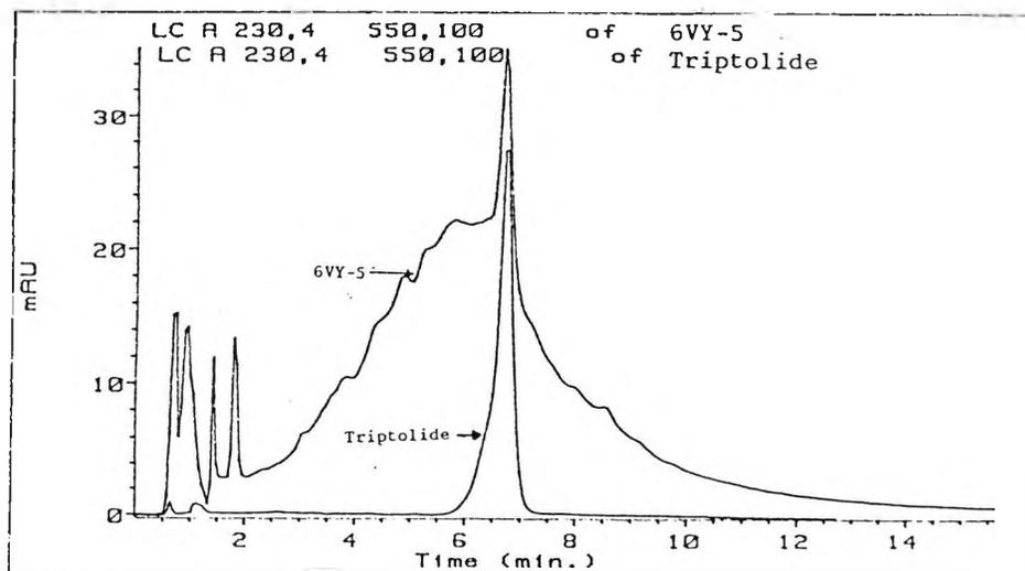
Figure 5-41. Superimposed chromatograms of the preparative subfraction 6VY-5 and a reference sample of triptolide, run under isocratic conditions on a 25 x 0.45 cm Hypersil-ODS 5 µm column, eluted with 28:72 MeCN/H<sub>2</sub>O at 2 ml/min, monitored at 230 nm.
