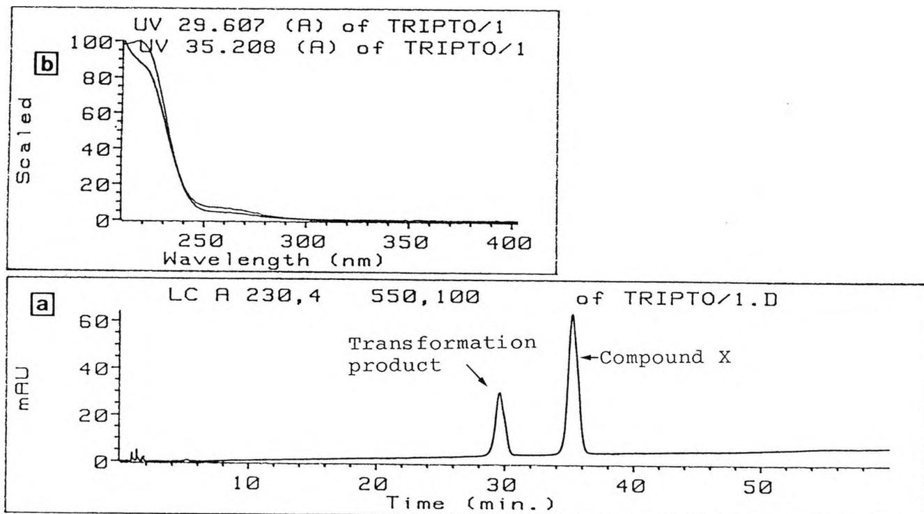
Figure 5-9. a) "Compound X", partially transformed on standing in methanol, chromatographed on a 25 x 0.45 cm Hypersil-ODS 5  $\mu$ m HPLC column, eluted with a continuous gradient from 10:10:80 to 22:22:56 MeOH/MeCN/H<sub>2</sub>O using a 50 ml mixing flask at 2 ml/min, monitored at 230 nm. b) UV spectra with the photodiode array detector of both, "Compound X" and its transformation product.
