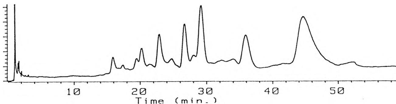
Figure 5-28. Resolution of P5 on a 25 x 0.45 cm Exsil-ODS 5  $\mu$ m column, eluted with 8:8:84 MeCN/MeOH/H<sub>2</sub>O at 2 ml/min and monitored at 230 nm.
