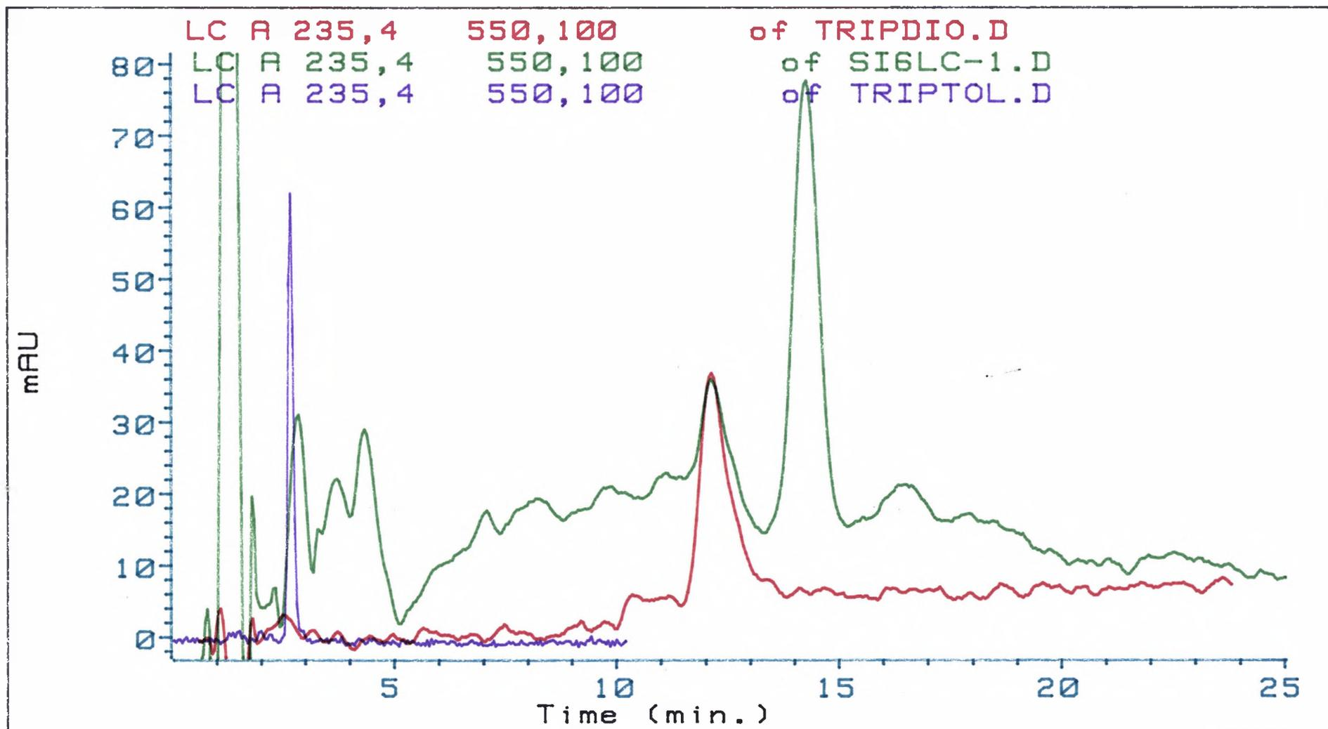
**Figure 5-44.** Normal phase HPLC method on Hypersil-silica to resolve the active materials triptolide and triptolide from the crude extract TW600. Samples were run on a 25 x 0.45 cm Hypersil-silica column, eluted with 99:1 CH<sub>2</sub>Cl<sub>2</sub>/MeOH at 2 ml/min and monitored at 230 nm.
