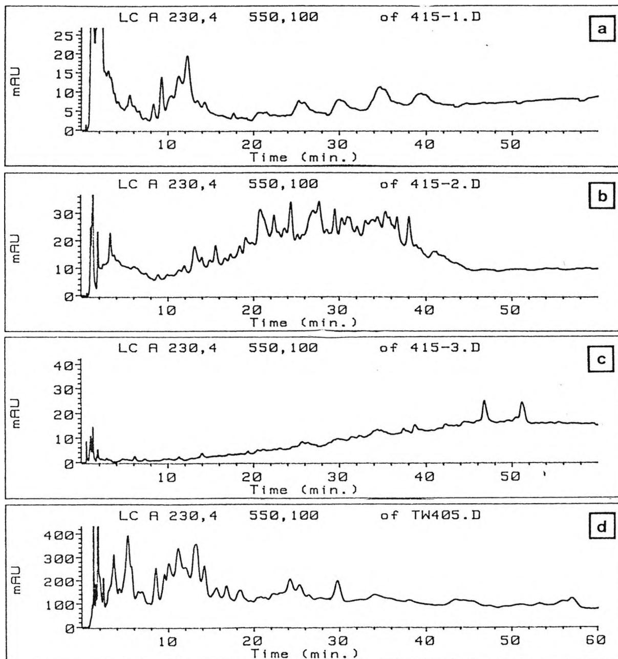
Figure 5-16. Fractions 415-1 (a), 415-2 (b), 415-3 (c) and starting material TW405 (d) run under continuous gradient elution on a 25 x 0.45 cm ODS-Hypersil 5  $\mu$ m column from 10:10:80 to 22:22:56 MeCN/MeOH/H<sub>2</sub>O using a 50 ml mixing flask at 2 ml/min, monitored at 230 nm. 415-2 is the only active fraction.
