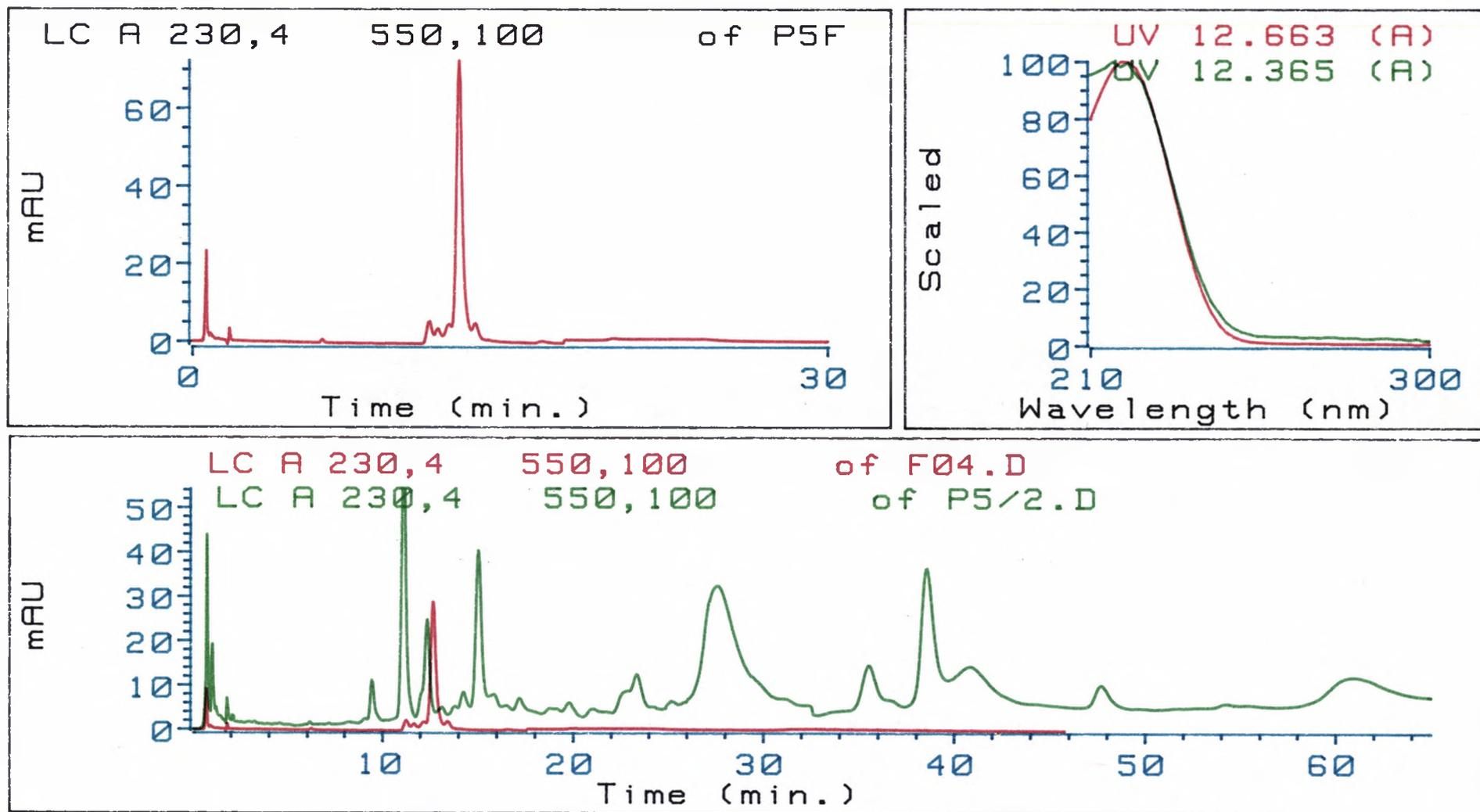
Figure 5-34. Analysis of the preparative subfraction P13 (top left) and superimposed chromatograms of P13 and the starting material P5 (bottom) on a 25 x 0.45 cm Exsil-ODS 5  $\mu$ m column, eluted with 96/4 H<sub>2</sub>O:THF at 2 ml/min and monitored at 230 nm with a HP 1040 photodiode array detector, using a 20  $\mu$ l sample loop. Top right: Superimposed UV spectra of P13 and that of the peak corresponding to P13 in the starting material P5.
