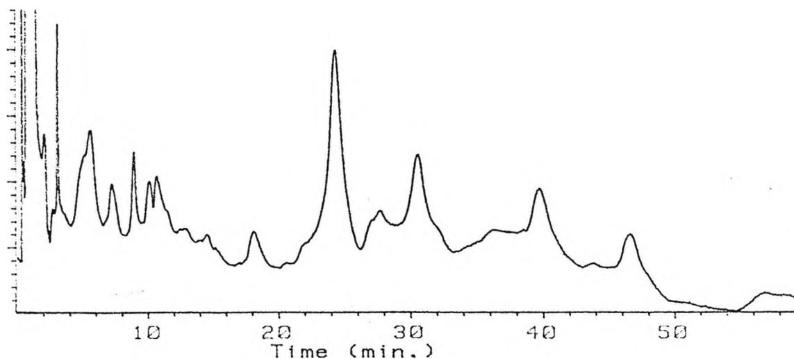
Figure 5-22. HPLC chromatogram corresponding to point 5 of the selectivity triangle in Figure 5-21, to achieve the optimum separation for 435-01-3 on a 25 x 0.45 cm ODS2-Spherisorb 5  $\mu$ m column, monitored at 230 nm. Mobile phase 2.5:2.1:1.4:94 MeOH/MeCN/THF/H<sub>2</sub>O, with a  $P'$  of 8.88.
