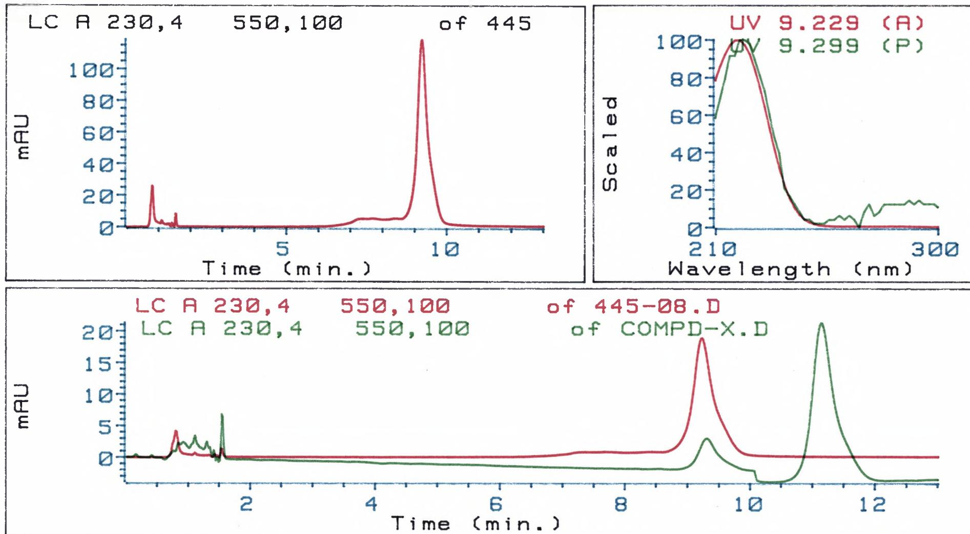
Figure 5-12. Purity assessment of 445-08, run under isocratic conditions with 25 x 0.45 cm Hypersil-ODS 5  $\mu$ m column, eluted with 28:72 MeCN/H<sub>2</sub>O at 2 ml/min, monitored at 230 nm (Top left). (Top right): Superimposed UV spectra of 445-08 and that of the transformation product of "Compound X". (Bottom): Superimposed chromatograms of 445-08 and the partially transformed reference sample of "Compound X". 445-08 corresponds to the transformation product of Compound X.
