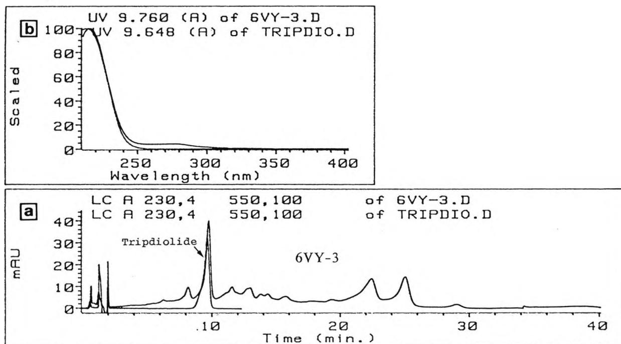
Figure 5-43. a) Superimposed analytical chromatograms of the preparative subfraction 6VY-3 and a reference sample of tripdiolide; run on a 25 x 0.45 cm Exsil-ODS 5  $\mu$ m column with 96:4 H<sub>2</sub>O/THF at 2 ml/min and monitored at 230 nm with a HP 1040 photodiode array detector. b) Superimposed UV spectra of the main peak of 6VY-3 and the reference sample of tripdiolide. The main component in 6VY-3 is tripdiolide.
