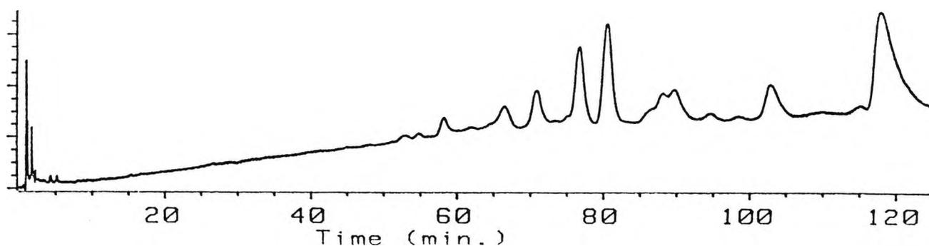
Figure 5-29. Resolution of P5 on a 25 x 0.45 cm Exsil-ODS 5  $\mu$ m column, eluted with a continuous gradient from 4:4:92 to 9:9:82 MeCN/MeOH/H<sub>2</sub>O at 2 ml/min using a 25 ml mixing flask and monitored at 230 nm.
