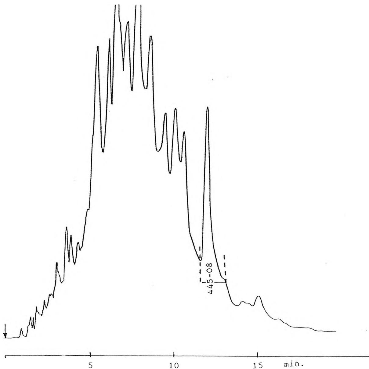
Figure 5-11. Semipreparative isocratic separation of the active fraction 425-08 on a 33 x 0.7 cm ODS-Hypersil 5  $\mu\text{m}$  column eluted with 28:72 MeCN/H<sub>2</sub>O at 5 ml/min and monitored at 230 nm at 0.02 AUFS to obtain subfraction 435-08. Loaded sample : 5 mg in MeCN on a 100  $\mu\text{l}$  injection loop.
