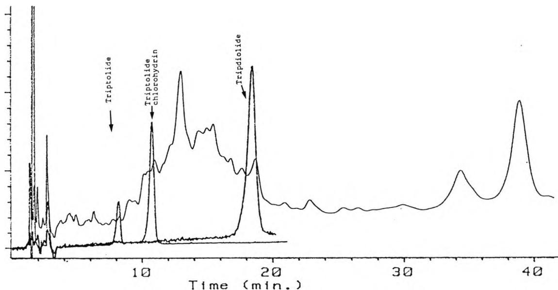
Figure 5-42. Normal phase HPLC separation of the crude fraction TW600 on 25 x 0.45 cm Nucleosil-nitro bonded 5  $\mu$ m column, eluted with 80:5:5:10 Hexane/ $\text{CH}_2\text{Cl}_2$ /THF/MeOH at 2 ml/min, monitored at 230 nm. Comparison with the active reference samples of triptolide, triptolide chlorohydrin and triptidiolide.
