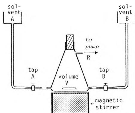
Fig. 5-3: Apparatus for generation of solvent gradients. <sup>1</sup>
