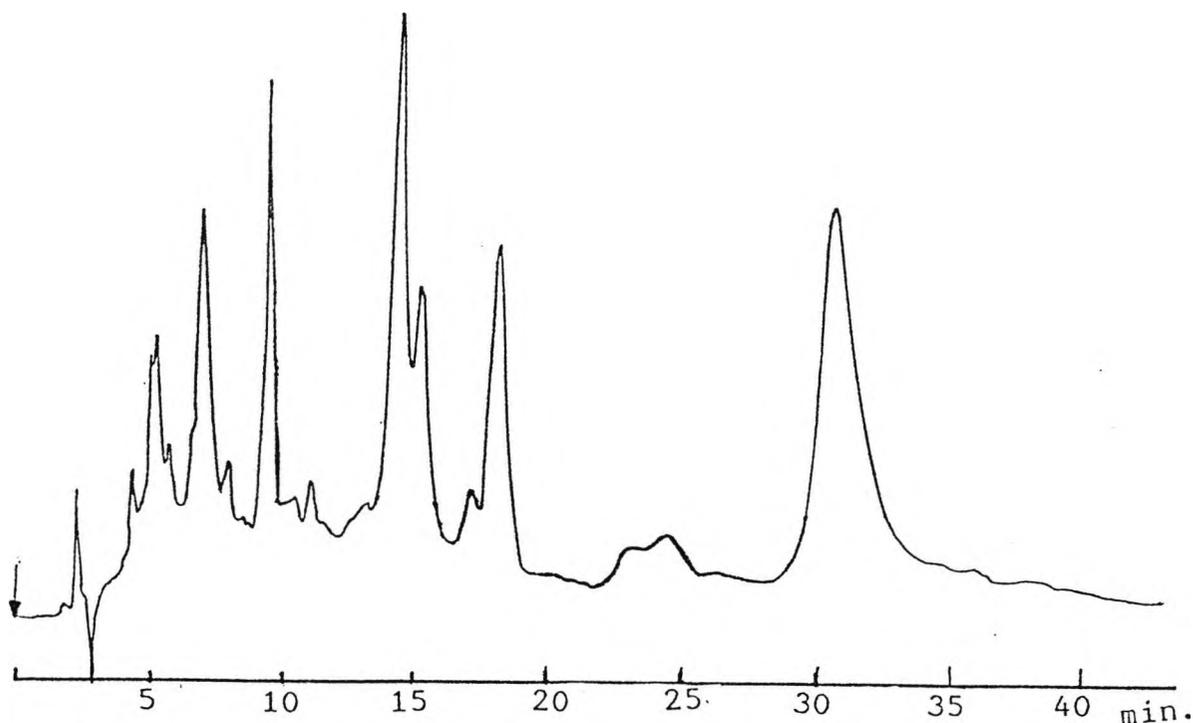
Figure 5-18. Normal phase HPLC separation of subfraction 435-01-3 in 25 x 0.45 cm Nucleosil-nitro bonded 5  $\mu$ m column, eluted with 80:5:5:10 Hexane/ $\text{CH}_2\text{Cl}_2$ /THF/MeOH at 2 ml/min, monitored at 230 nm.
