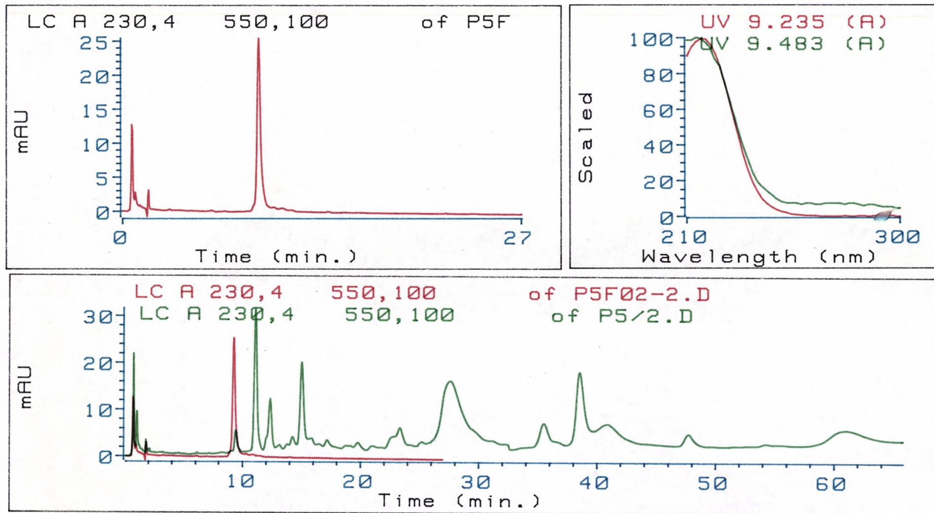
**Figure 5-32.** Analysis of the preparative subfraction P8 (top left) and superimposed chromatograms of P8 and the starting material P5 (bottom) on a 25 x 0.45 cm Exsil-ODS 5  $\mu\text{m}$  column, eluted with 96/4 H<sub>2</sub>O:THF at 2 ml/min and monitored at 230 nm with a HP 1040 photodiode array detector, using a 20  $\mu\text{l}$  sample loop. Top right: Superimposed UV spectra of P8 and that of the peak corresponding to P8 in the starting material P5.
