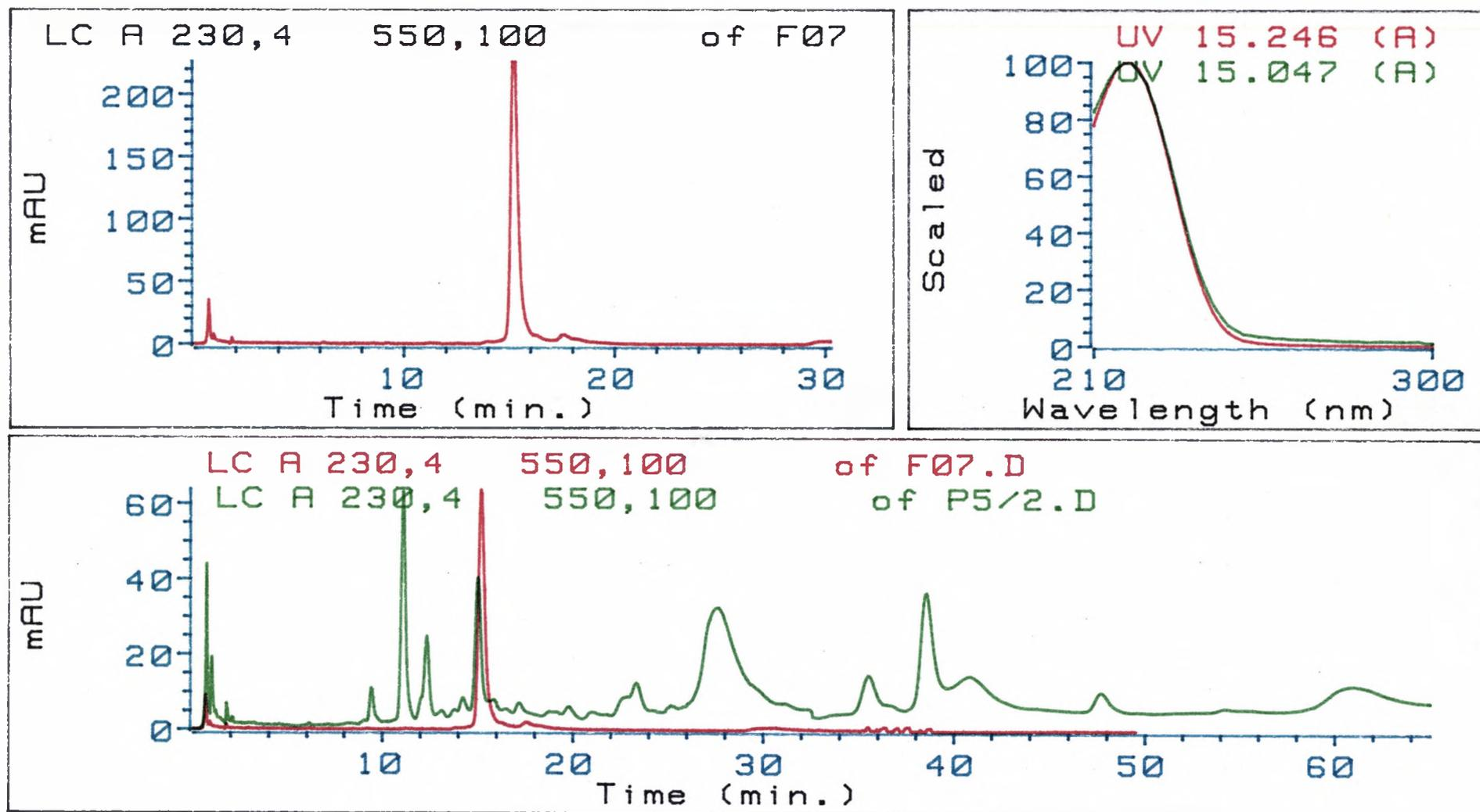
Figure 5-35. Analysis of the preparative subfraction P16 (top left) and superimposed chromatograms of P16 and the starting material P5 (bottom) on a 25 x 0.45 cm Exsil-ODS 5  $\mu$ m column, eluted with 96/4 H<sub>2</sub>O:THF at 2 ml/min and monitored at 230 nm with a HP 1040 photodiode array detector, using a 20  $\mu$ l sample loop. Top right: Superimposed UV spectra of P16 and that of the peak corresponding to P16 in the starting material P5.
