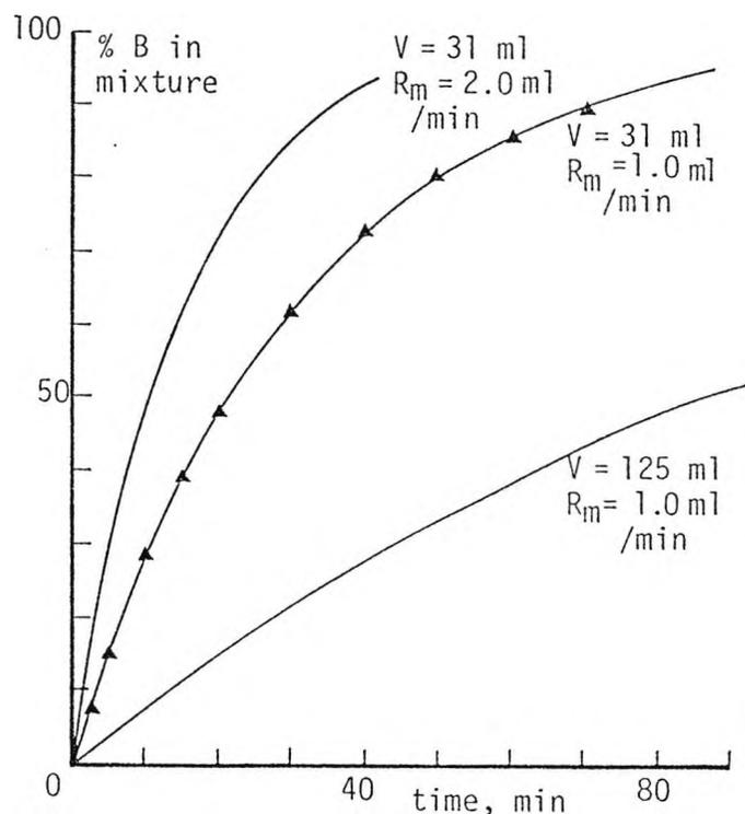
Figure 5-4. Gradient profiles produced by mixing vessels (calculated gradients). <sup>1</sup>
