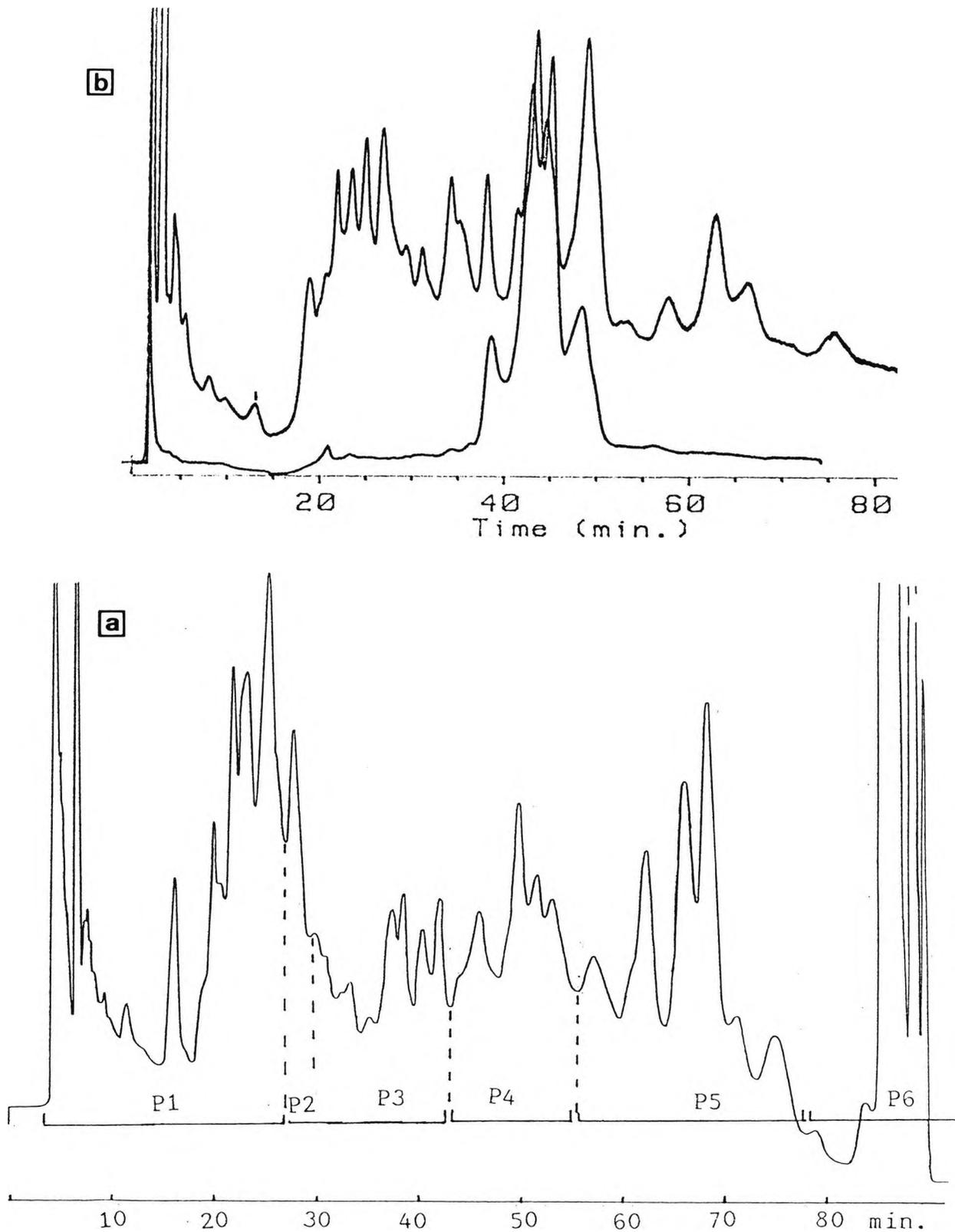
Figure 5-27. a) Separation of 402-S in 6 subfractions, on a 1" O.D. x 50 cm ODS-Vydac 300A 15-20  $\mu$ m preparative column (protected with a 9 cm x 1" ODS-Vydac 300A 15-20  $\mu$ m guard column), eluted for 5 min with 100% H<sub>2</sub>O, then gradient elution to 12:12:76 MeCN/MeOH/H<sub>2</sub>O at 36 ml/min using a 1 l mixing flask, monitored at 230 nm and 1 AUFS using an analytical flowcell. Loaded sample: up to 3 g dissolved in warm water and introduced with a 13 ml sample loop.
