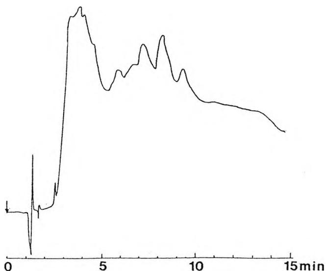
Figure 5-17. Normal phase HPLC separation of subfraction 435-01-3 in a 25 x 0.45 cm Ultrasphere-cyano 5  $\mu$ m column, eluted with 85:5:15 Hexane/ $\text{CH}_2\text{Cl}_2$ /MeOH at 2 ml/min, monitored at 230 nm.
