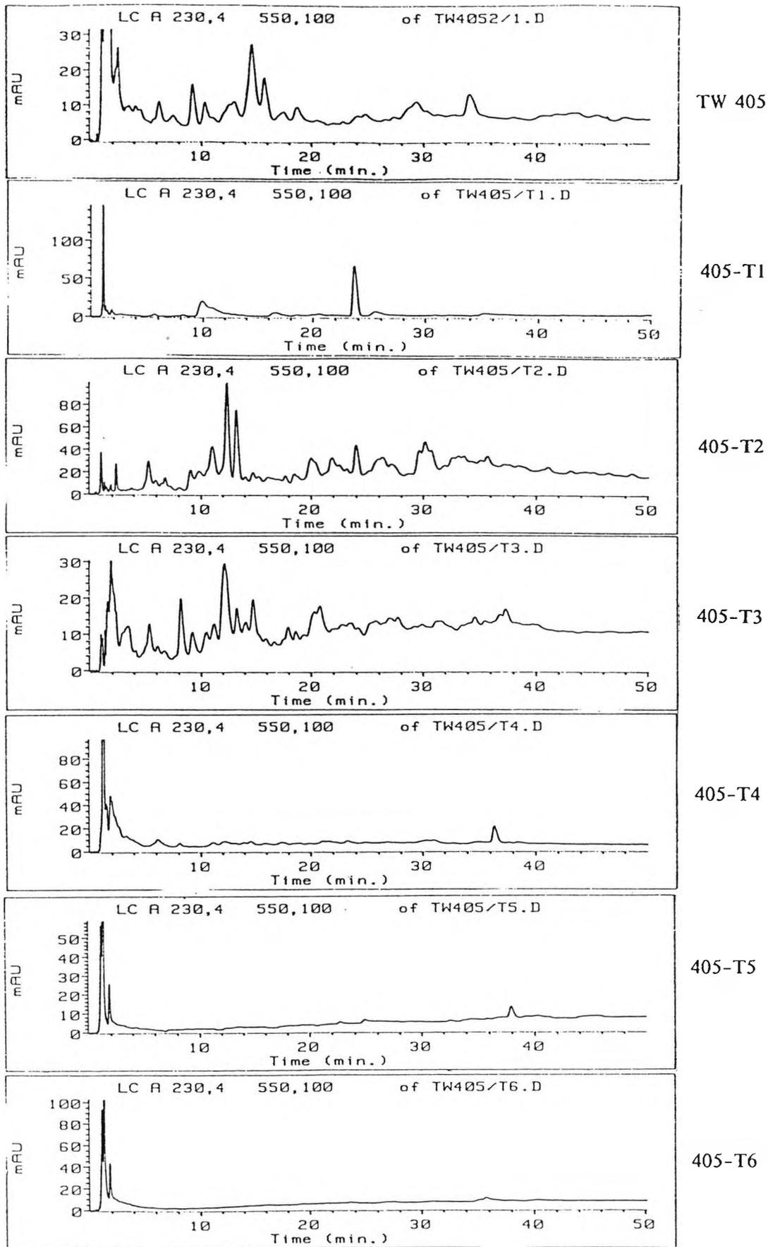
Figure 5-2. Comparison of the 6 preparative TLC fractions of TW405 (silica plate, 93:7 CHCl<sub>3</sub>/MeOH) with the starting material 405. HPLC run on a 25 x 0.45 cm ODS-Hypersil 5 μm, eluted with a continuous gradient elution from 10/10/80 to 22/22/56 MeCN/MeOH/H<sub>2</sub>O at 2 ml/min using a 25 ml mixing flask, monitored at 230 nm. Only 405-T2 and 405-T3 have male antifertility properties.
