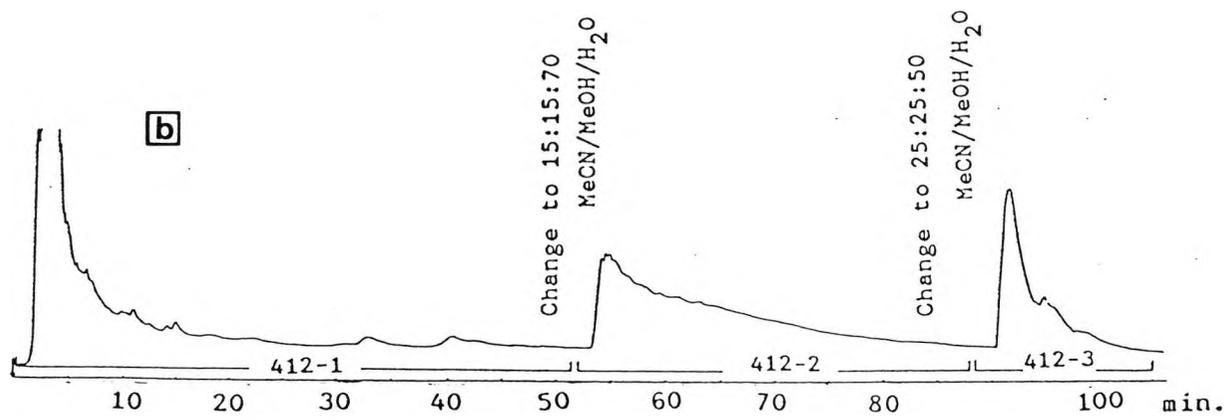
Figure 5-23. Multistep gradient separation of TW402 on ODS.
