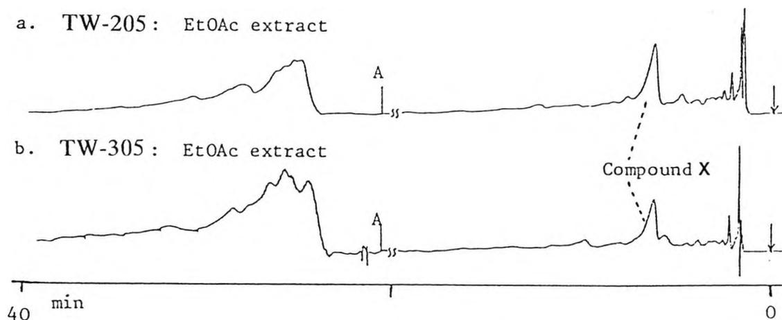
**Figure 4-3.** HPLC of solvent extraction fractions prepared from tablets of *Tripterygium wilfordii* according to Extraction Schemes 4-3 and 4-4. Column 25 x 0.45 cm Hypersil-APS 5  $\mu$ m, eluted initially with 8:2:10:80 MeCN-iPrOH-Hexane-CH<sub>2</sub>Cl<sub>2</sub>, switching to 15:5:80 MeCN-iPrOH-CH<sub>2</sub>Cl<sub>2</sub> at point A; monitored at 230 nm.
