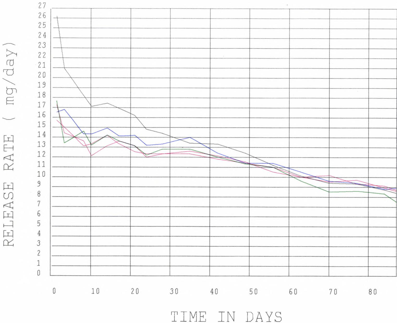
Fig. 9-3 Daily release rate of levonorgestrel 1.5 mm core diameter Dow Corning vaginal rings prepared for a linearity study.
