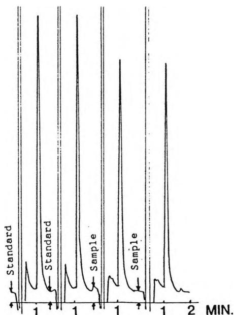
Fig. 9-1 Fast HPLC chromatogram of direct 200  $\mu$ l injections sample and standard levonorgestrel solutions on a 5 x 0.45 cm Hypersil-ODS 3  $\mu$ m column, eluted with 50:50 MeCN/H<sub>2</sub>O at 2 ml/min, monitored at 241 nm.
