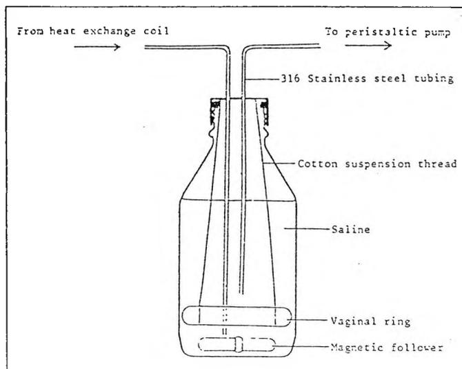
Fig. 8-1: Flow chamber for continuous elution of vaginal ring
