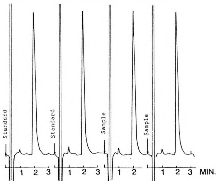
Fig. 8-5 Fast HPLC chromatogram of direct 200  $\mu\text{l}$  injection sample and standard progesterone solutions on a 5 x 0.45 cm Hypersil-ODS 3  $\mu\text{m}$  column, eluted with 50:50 MeCN/H<sub>2</sub>O at 2 ml/min, monitored at 241 nm.
