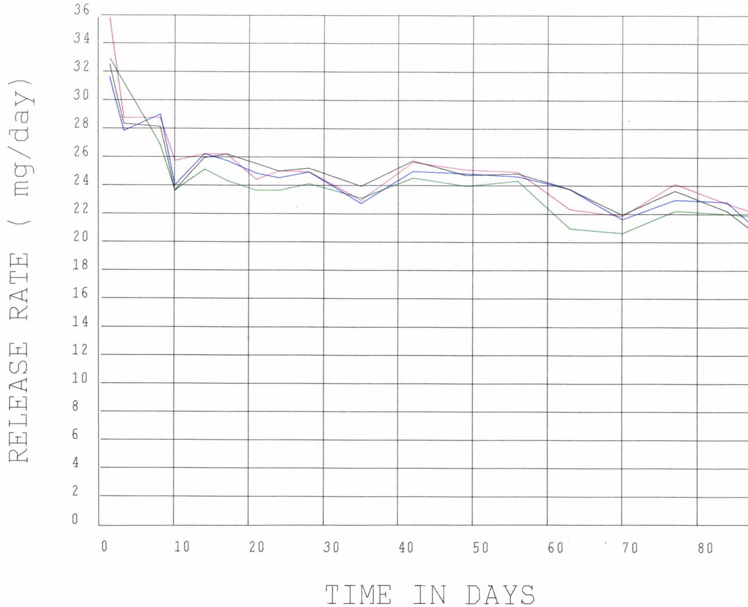
Fig. 9-6 Daily release rate of levonorgestrel 4 mm core diameter Dow Corning vaginal rings prepared for a linearity study.
