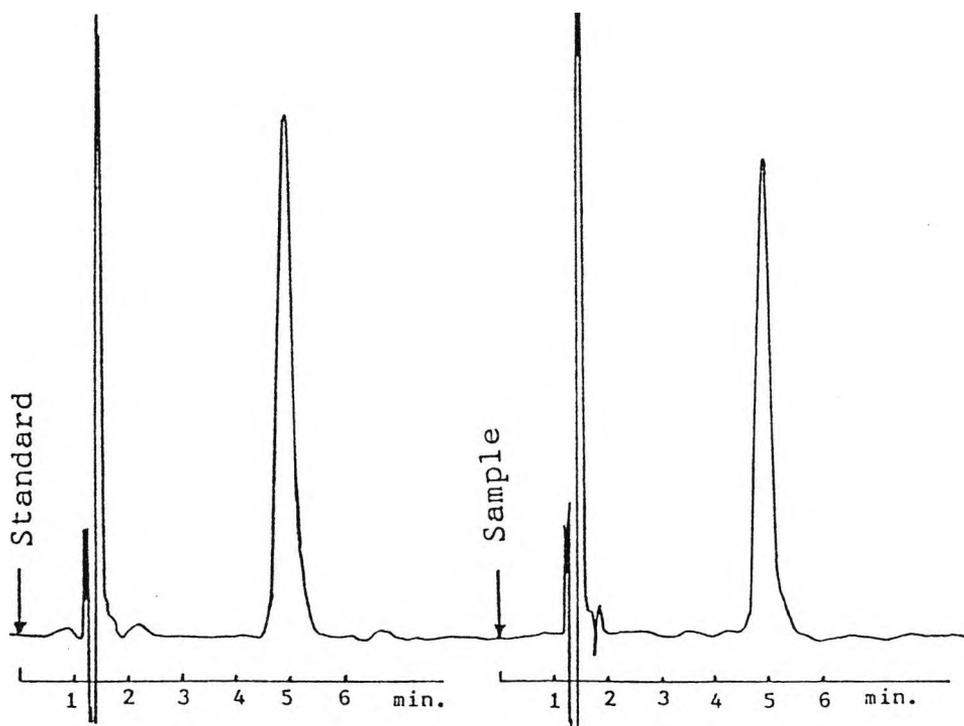
Fig. 8-4 HPLC chromatogram of standard and sample progesterone solution on a 25 x 0.45 cm Hypersil-ODS 5  $\mu$ m column, eluted with 50:50 MeCN/ $\text{H}_2\text{O}$  at 2 ml/min, monitored at 241 nm. 200 ml saline aliquots of sample and standard progesterone solutions, were extracted into chloroform, and the residue following evaporation were dissolved in MeCN prior to injection.
