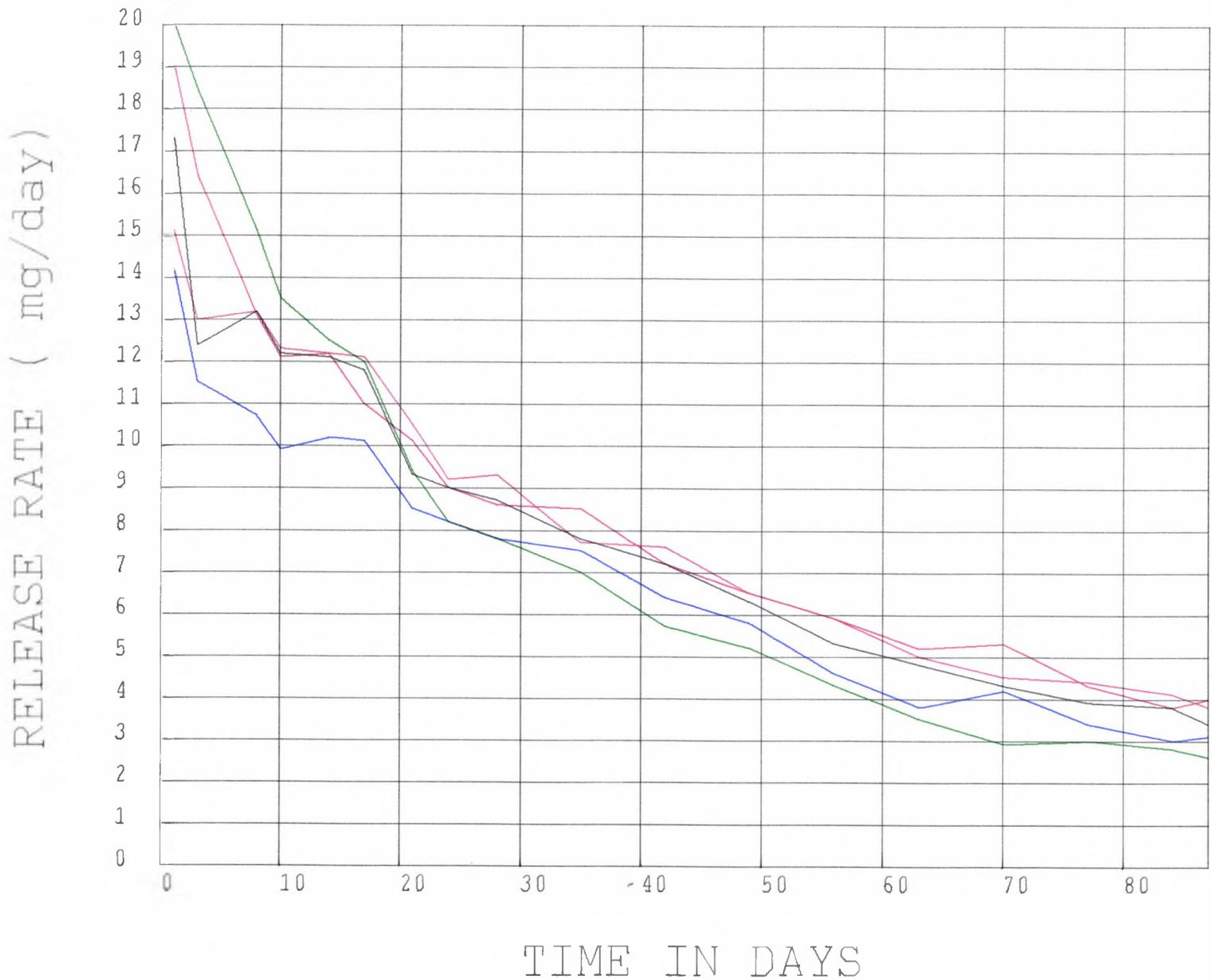
Fig. 9-2 Daily release rate of levonorgestrel 1 mm diameter Dow Corning vaginal rings prepared for a linearity study.
