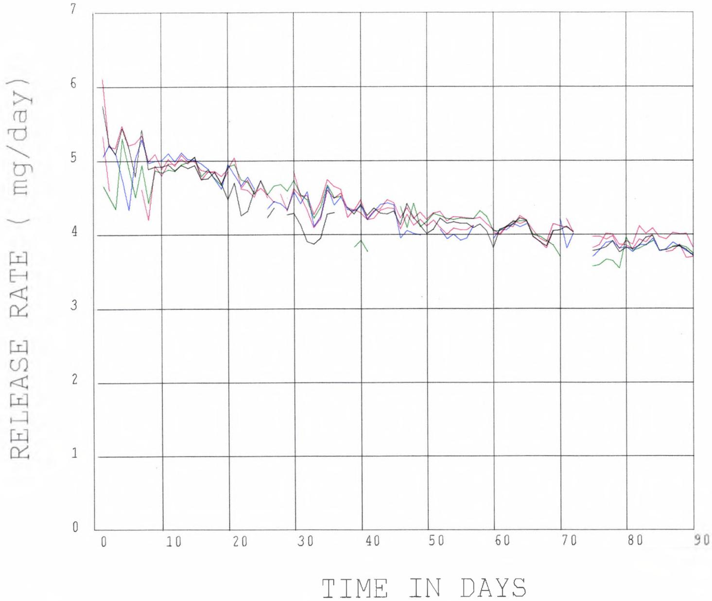
Fig. 8-10 Daily release rate of progesterone from 6 mm core diameter Dow Corning vaginal rings prepared for a linearity study.
