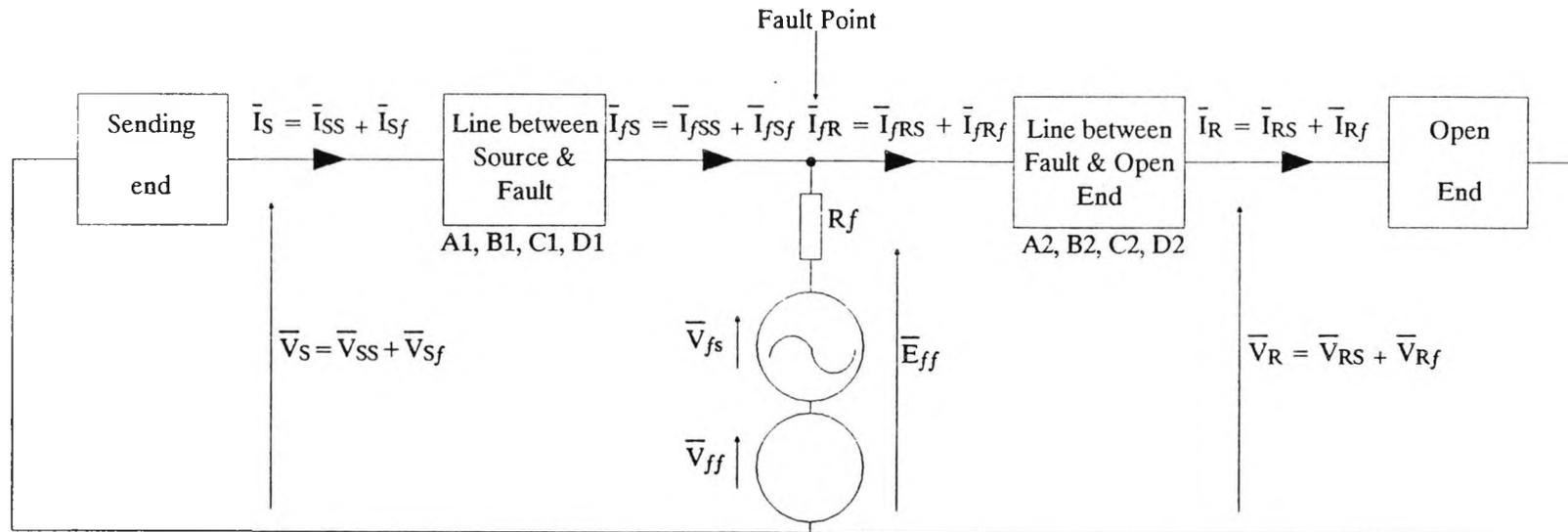
**FIG(4.4), FAULT TRANSIENT MODEL UTILISING SUPERIMPOSED FAULT VOLTAGE.**
