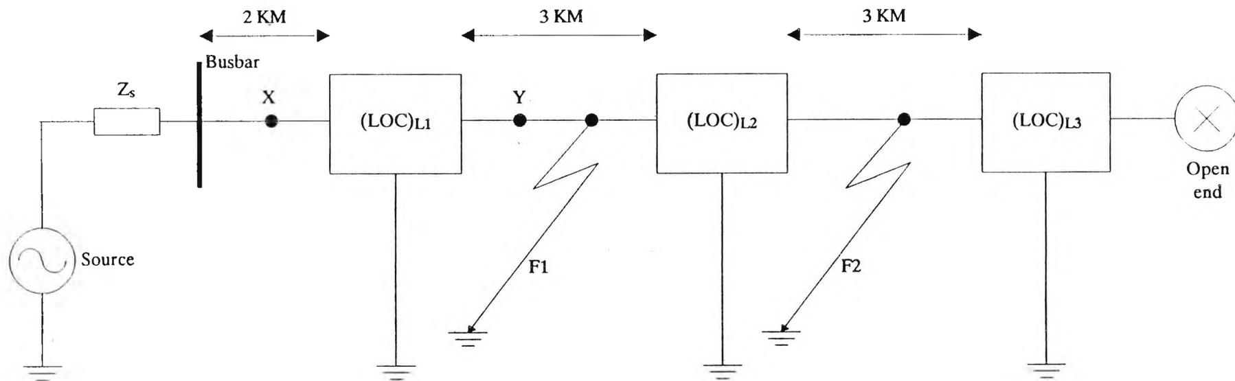
**FIG (6.1), SCHEMATIC DIAGRAM OF THE SYSTEM SIMULATED PER PHASE WITH IN-ZONE FAULT, F1 AND OUT-OF-ZONE FAULT, F2**
