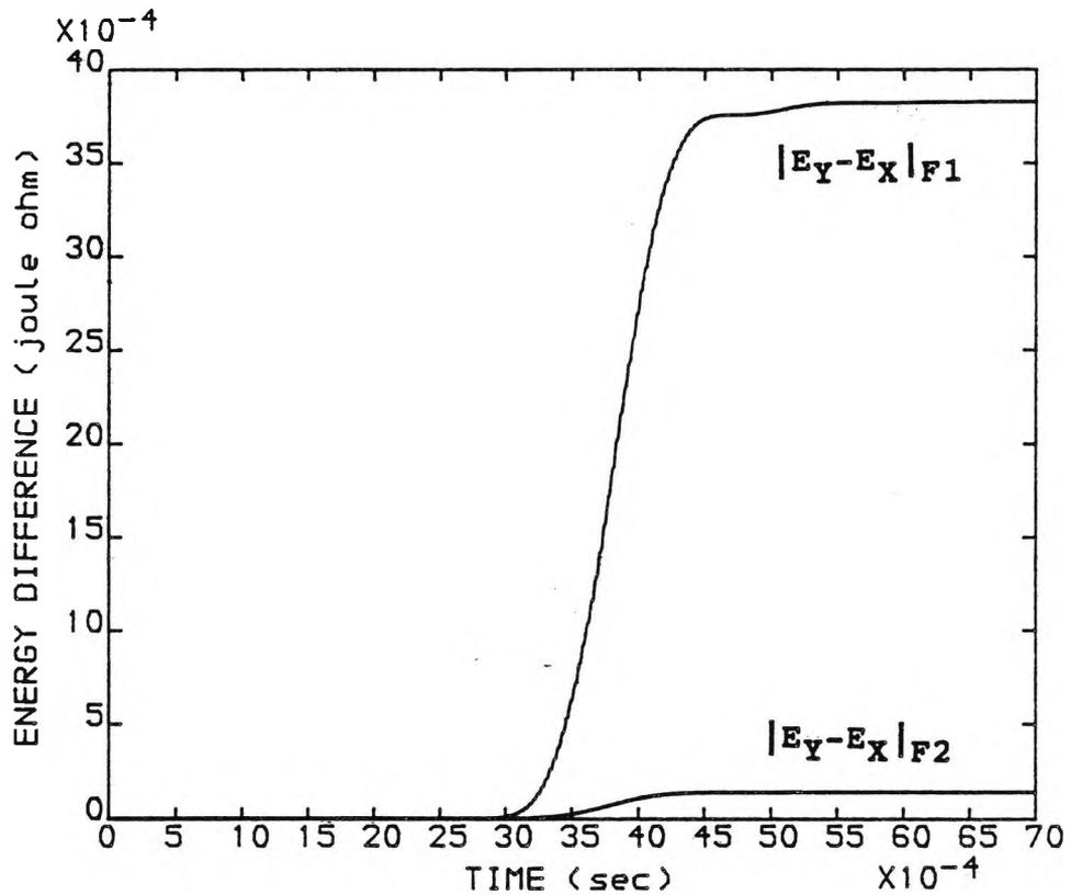
FIG (6.8). ENERGY DIFFERENCE COMPARISON BY (LOC) L1 BETWEEN IN-ZONE AND OUT-OF-ZONE FAULTS WITH  $f_c = 90.0$  (kHz)
