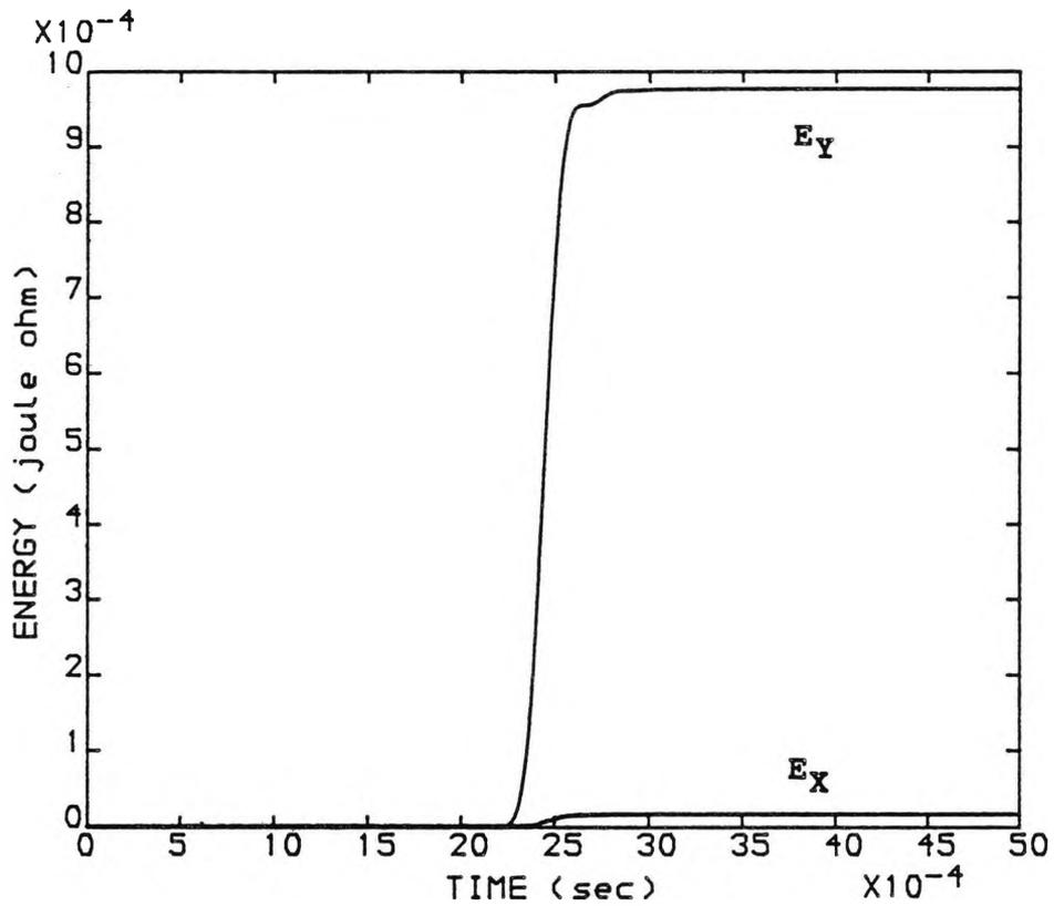
FIG (5.27). ENERGY COMPARISON BY (LOC) L1 DUE TO A FAULT AT POINT F1. WITH  $f_c = 270.0$  (kHz)
