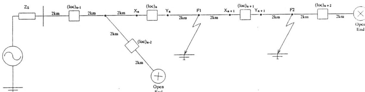
Figure 1 Schematic diagram of a simple overhead radial system
