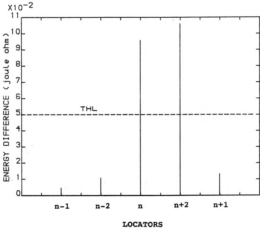
FIG (7.12). COMPARISON OF ENERGY DIFFERENCES OF LOCATORS WITH THL DUE TO A FAULT AT F1
