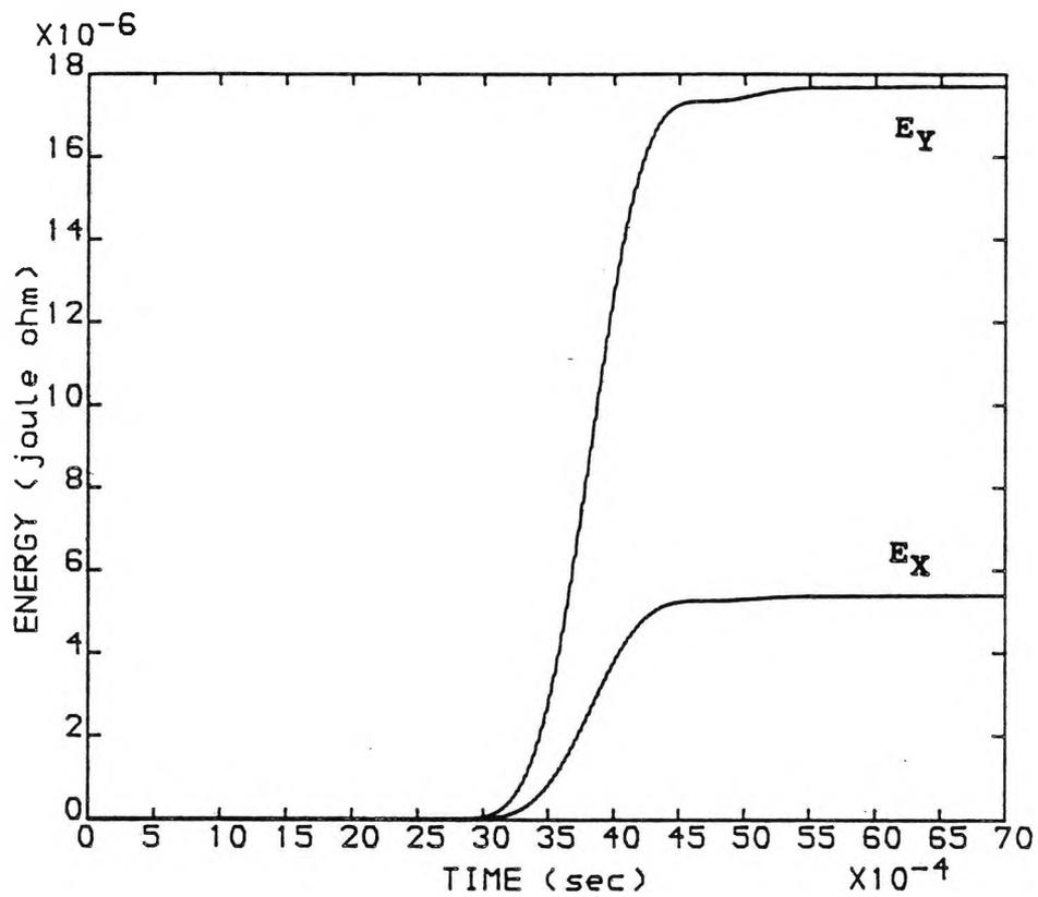
FIG (5.16). ENERGY COMPARISON BY (LOC) L1 DUE TO A FAULT AT POINT F1, WITH  $f_c = 90.0$  (kHz)
