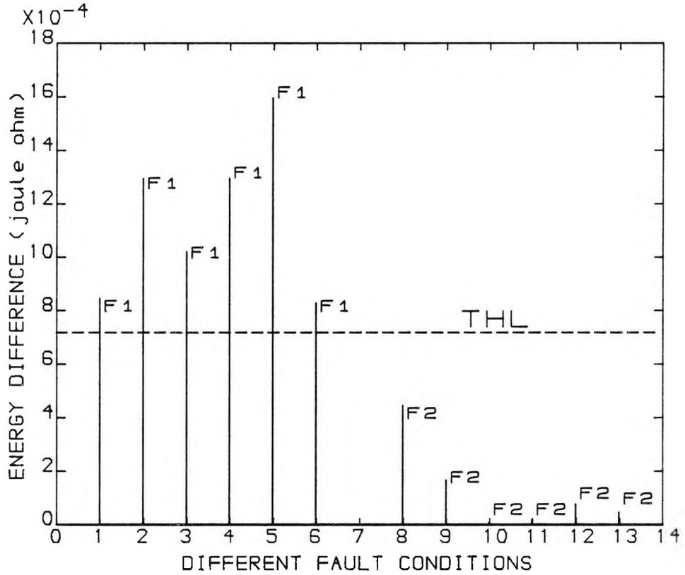
FIG (6.26), DISCRIMINATION BETWEEN IN-ZONE AND OUT-OF-ZONE FAULTS UNDER DIFFERENT FAULT CONDITIONS
