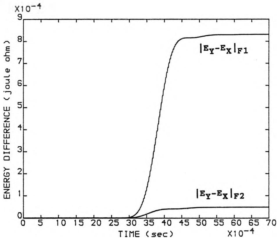
FIG (6.17). ENERGY DIFFERENCE COMPARISON BY (LOC)L1 BETWEEN IN-ZONE AND OUT-OF-ZONE FAULTS WITH  $f_c = 90.0$  (kHz)
