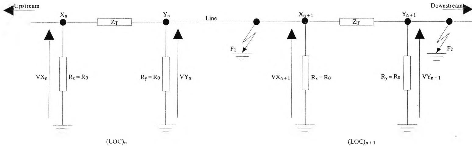
FIG(3.4), THE EQUIVALENT CIRCUITS OF  $(LOC)_n$  AND  $(LOC)_{n+1}$  PER PHASE AT CENTRE FREQUENCY  $f_c$ .
