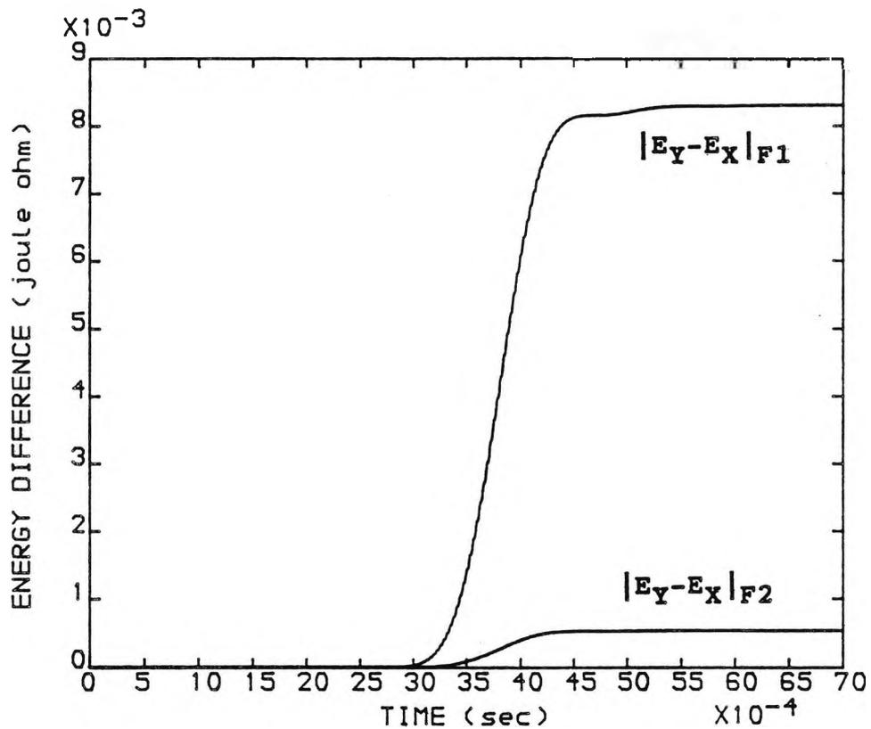
FIG (6.9). ENERGY DIFFERENCE COMPARISON BY (LOC) L1 BETWEEN IN-ZONE AND OUT-OF-ZONE FAULTS WITH  $f_c = 90.0$  (kHz)
