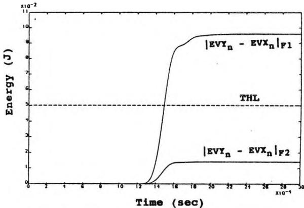
Figure 9 Comparison of energy level difference for in-zone and out-of-zone faults
