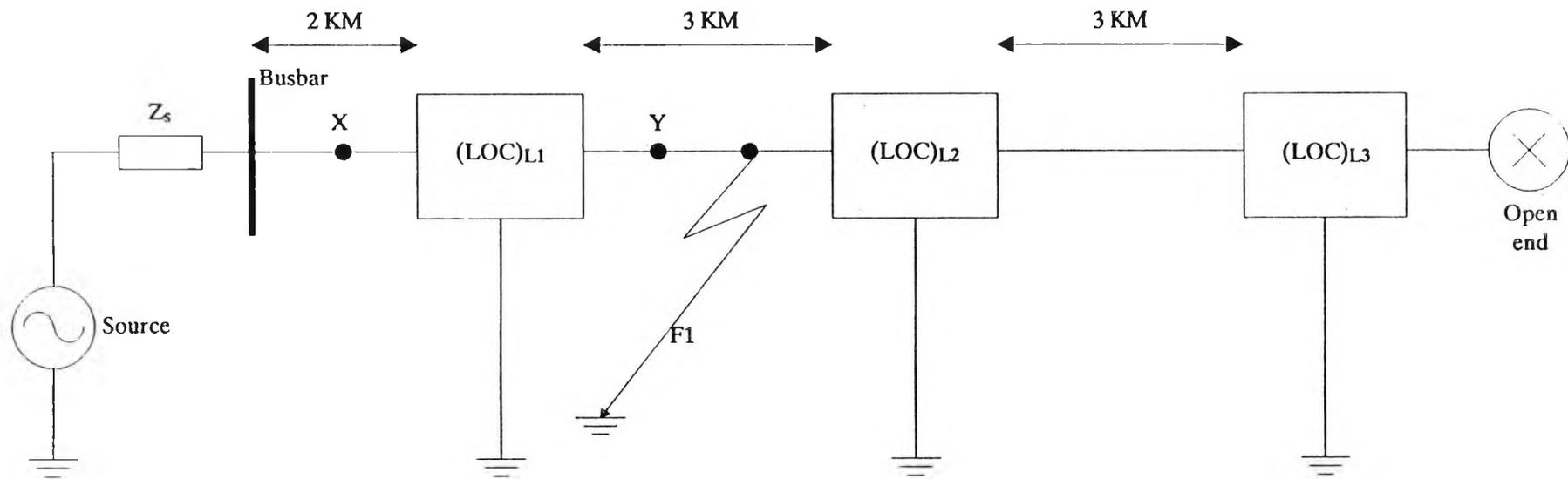
FIG (5.1), SCHEMATIC DIAGRAM OF THE SYSTEM SIMULATED PER PHASE WITH AN IN-ZONE FAULT, F1
