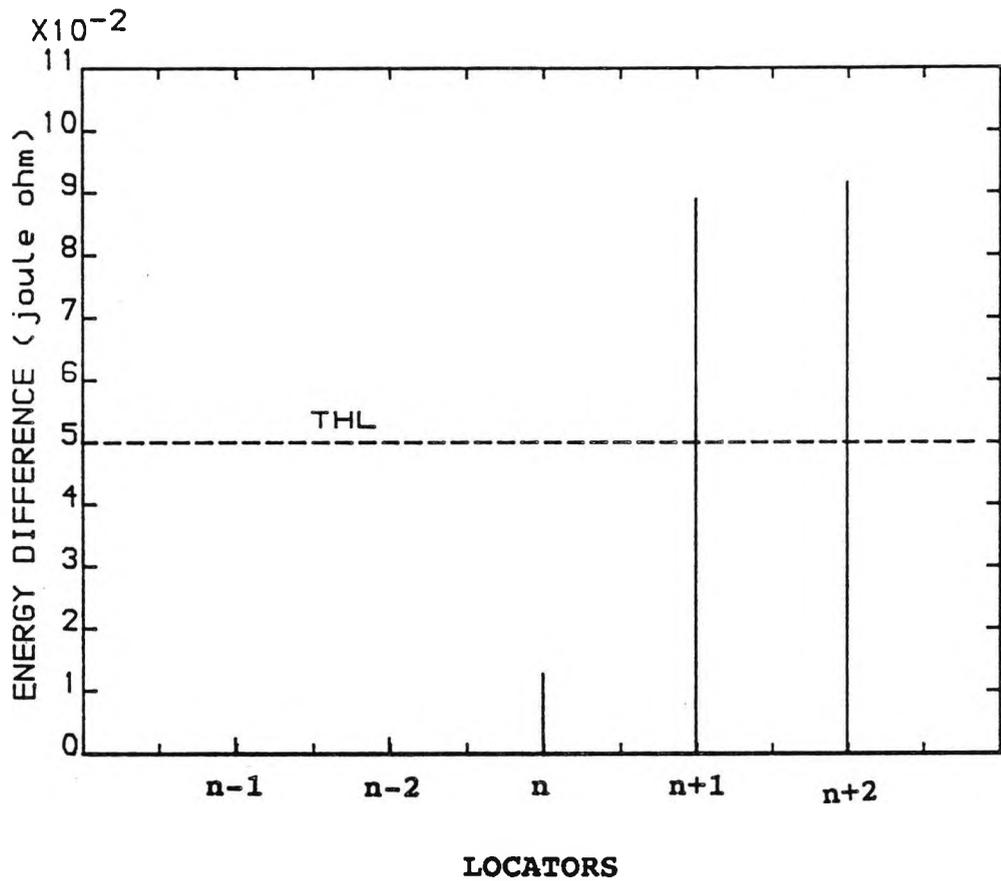
FIG (7.13). COMPARISON OF ENERGY DIFFERENCES OF LOCATORS WITH THL DUE TO A FAULT AT F2
