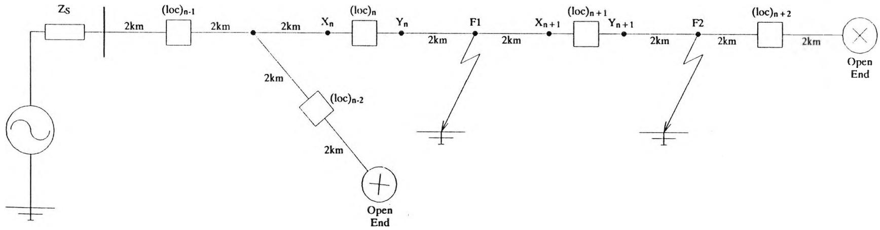
FIG (7.1), SCHEMATIC DIAGRAM OF A SIMPLE OVERHEAD RADIAL SYSTEM
