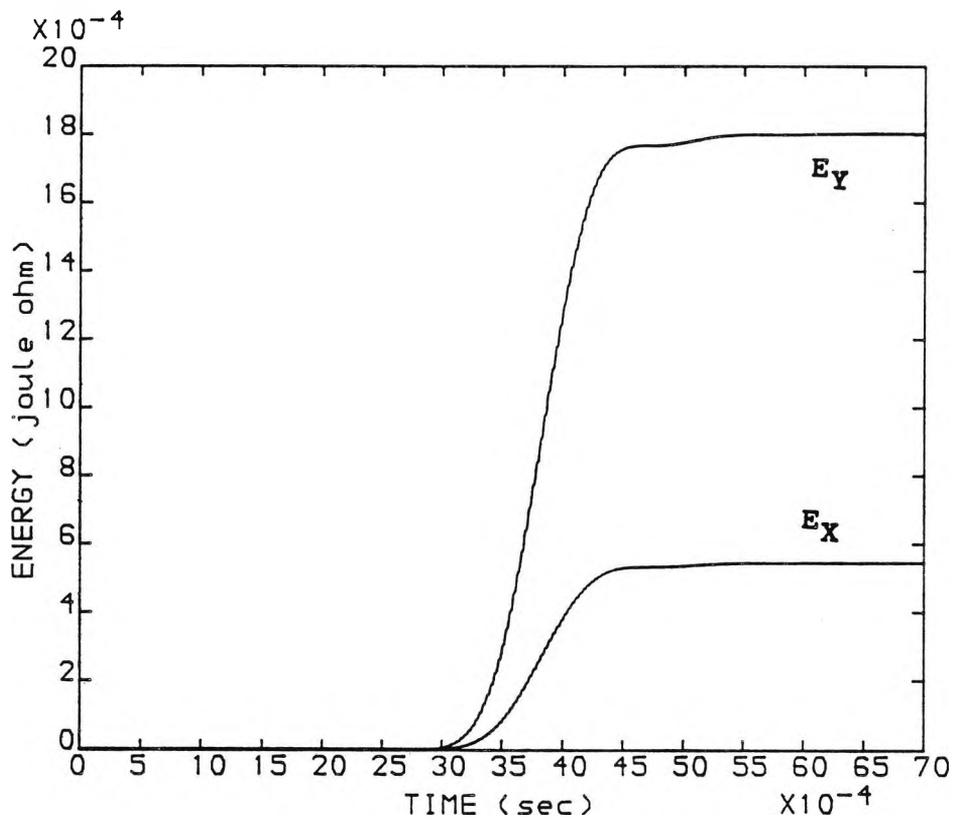
FIG (5.13). ENERGY COMPARISON BY (LOC) L1 DUE TO A FAULT AT POINT F1. WITH  $f_c = 90.0$  (kHz)
