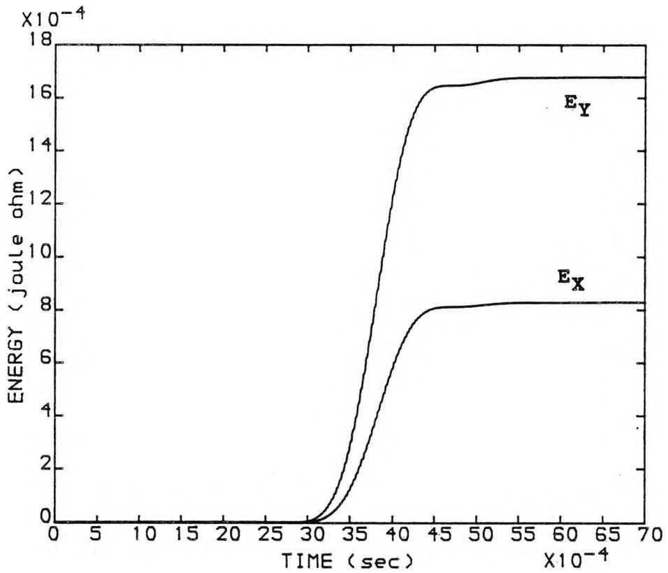
FIG (5.18). ENERGY COMPARISON BY (LOC) L1 DUE TO A FAULT AT POINT F1. WITH  $f_c = 90.0$  (kHz)
