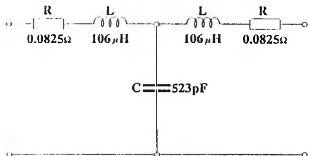
Fig (3) A T-section representing 100m length of a typical 11kV line
