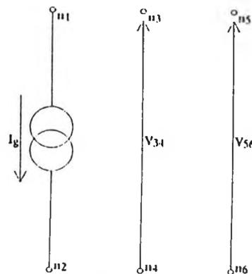
Fig (6) A 2-dimensional voltage controlled current source
