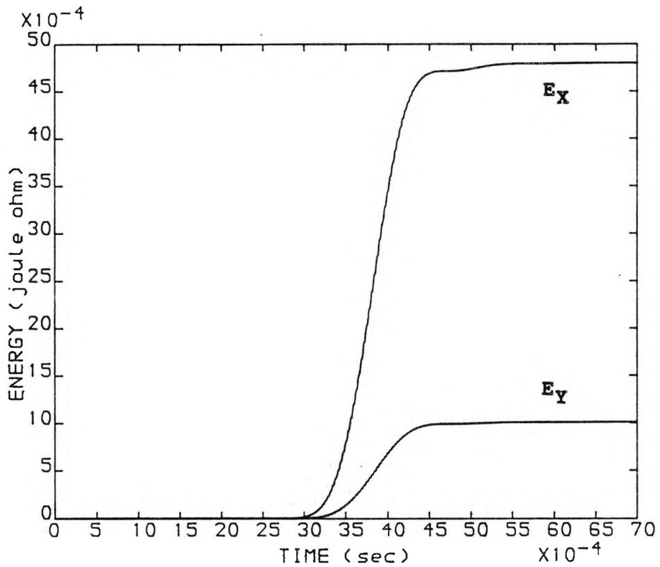
FIG 5.9 (b). ENERGY COMPARISON BY (LOC) L2 DUE TO A FAULT AT POINT F1, WITH  $f_c = 90.0$  (kHz)
