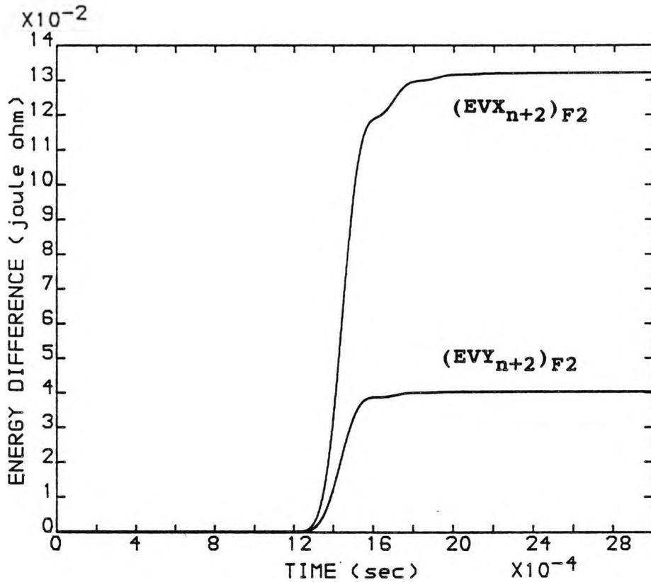
FIG (7.10). ENERGY COMPARISON BY (LOC)  $n+2$  DUE TO A FAULT AT POINT F2 WITH  $f_c = 90.0$  (kHz)
