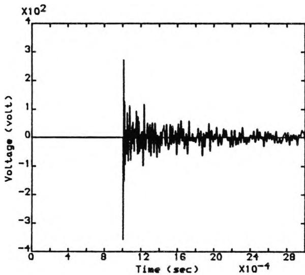
Figure 6 Voltage across resistor  $R_{p1}$  of locator  $(Loc)_n$
