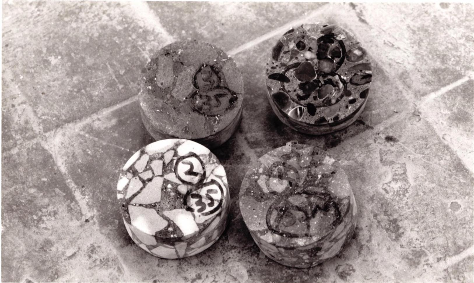
Figure 6.7. Cores used for VCD test.
