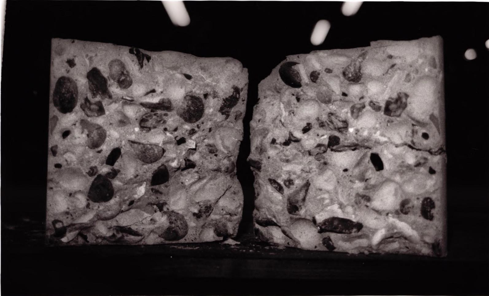
Figure 4.9. Splitting tensile failure of concrete with Thames Valley gravel.
