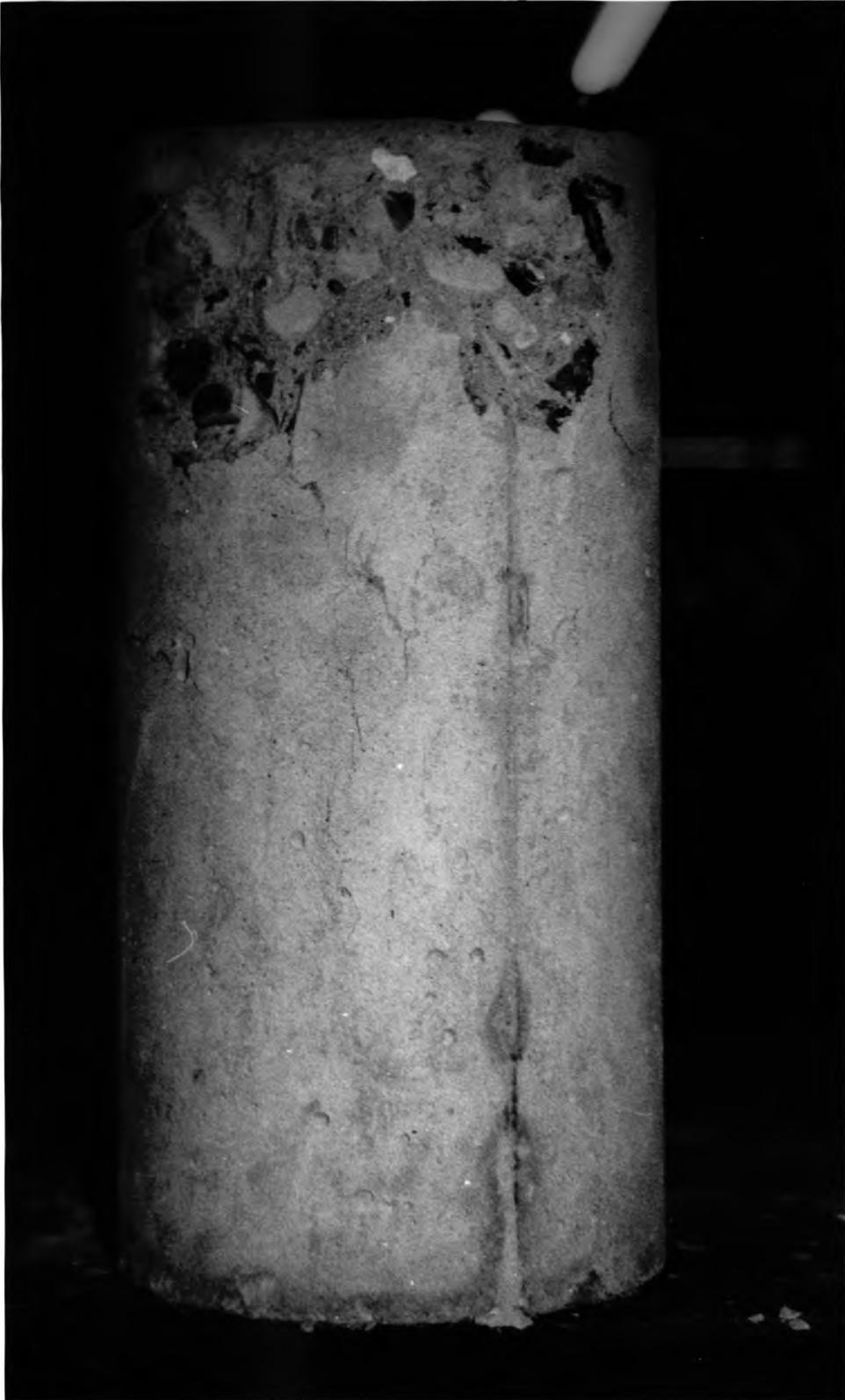
Figure 4.7. Cylinder made from concrete with Thames Valley gravel aggregate after failure in compression.
