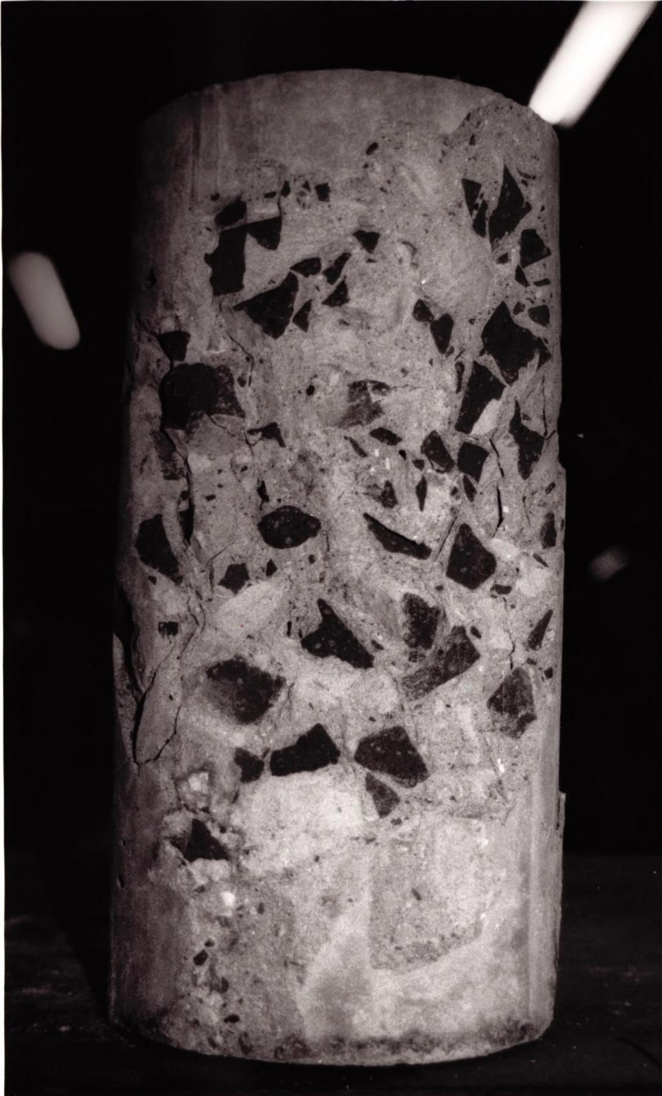
Figure 4.6. Cylinder made from concrete with engineering brick aggregate after failure in compression.
