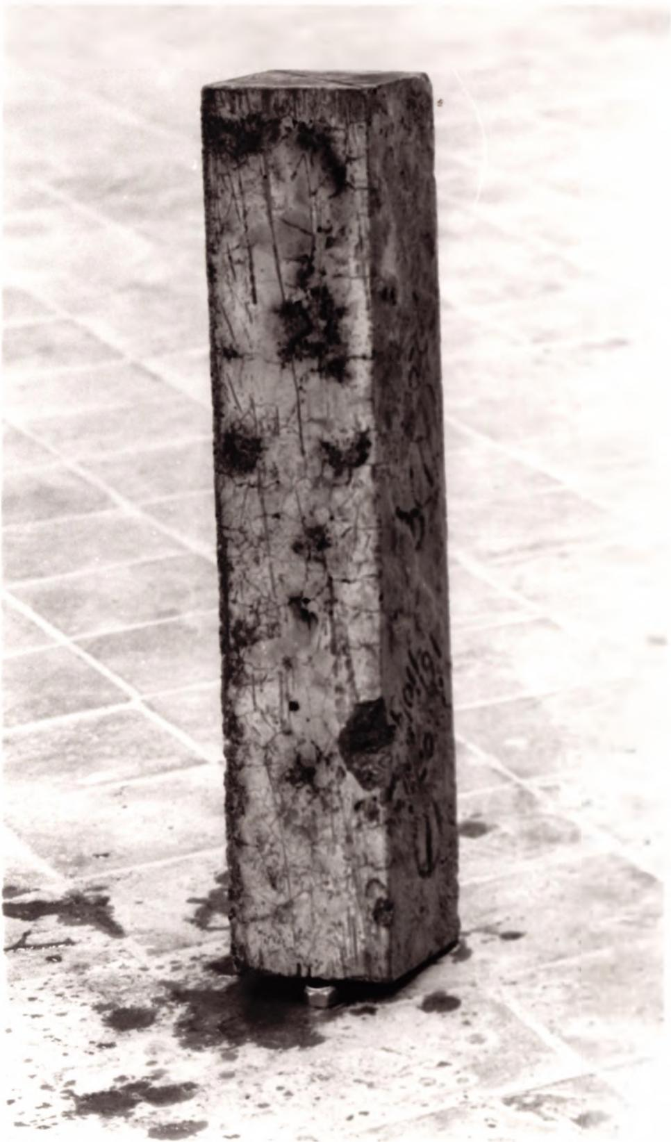
Figure 8.3. A specimen of concrete with normal construction brick aggregate after 50 cycles of sulphate resistance test.
