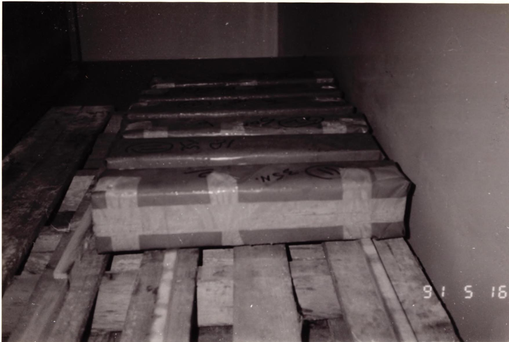
Figure 7.1. Specimens of frost resistance test in the refrigerating cabinet.
