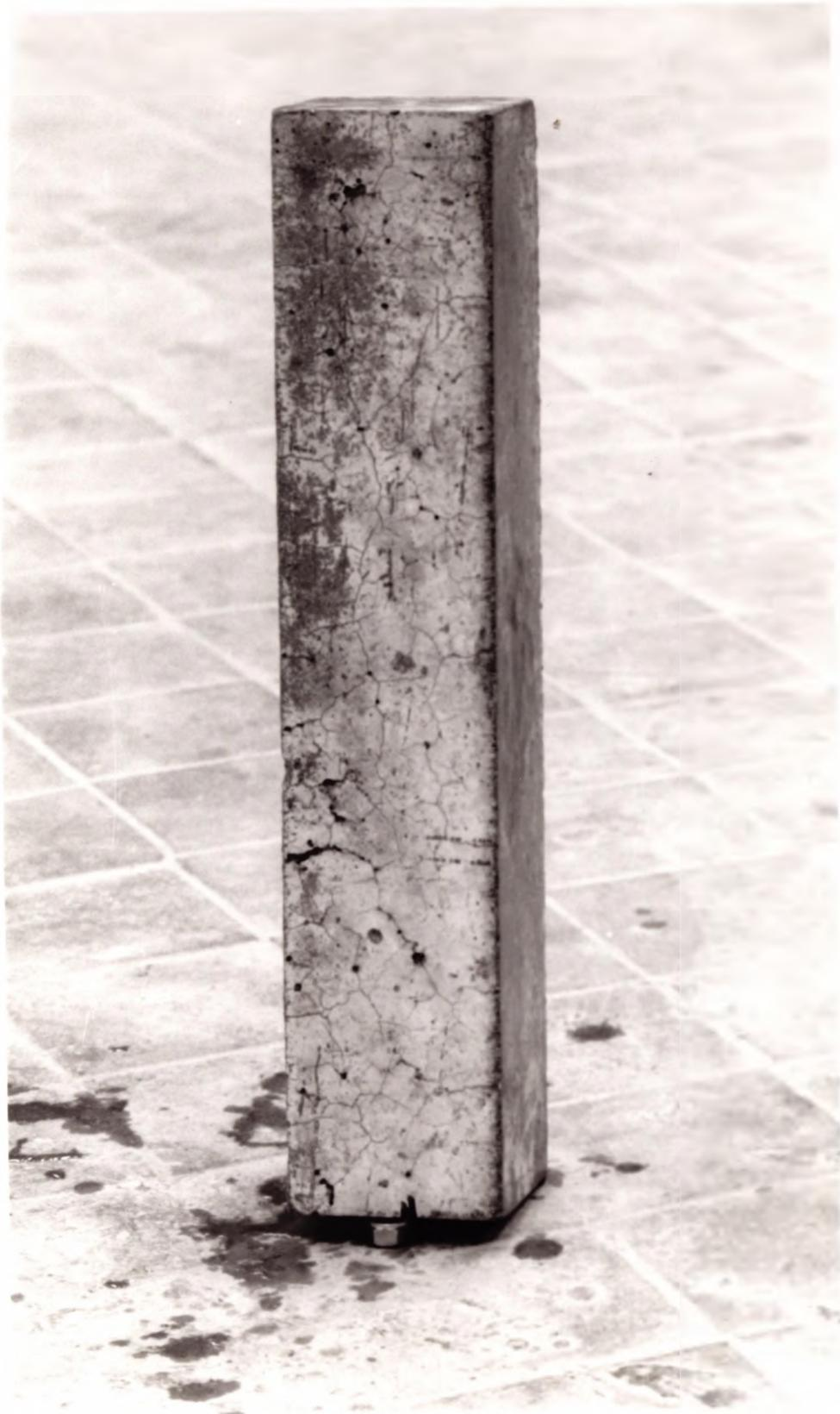
Figure 8.6. A specimen of gravel concrete after 50 cycles of sulphate resistance test.
