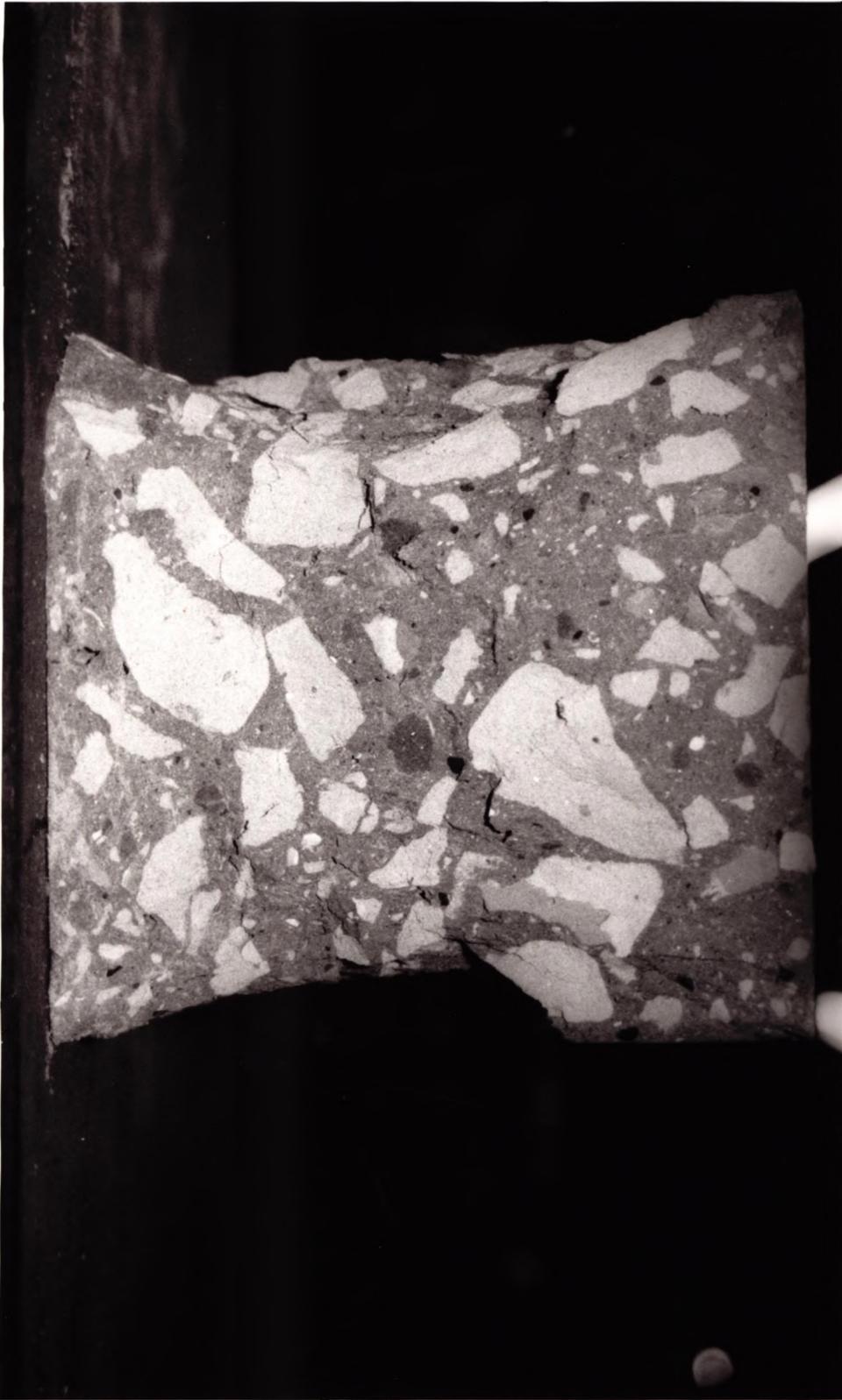
Figure 4.4. Typical failure of cubes of brick aggregate concrete
