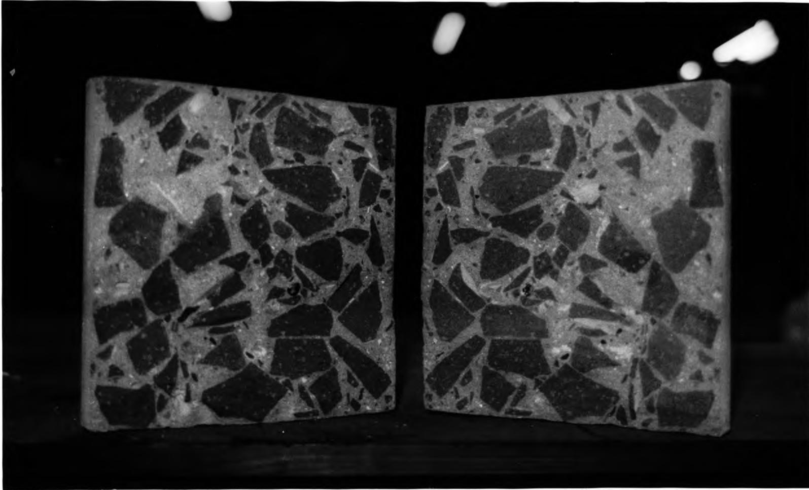
Figure 4.8. Splitting tensile failure of concrete with engineering brick aggregate.
