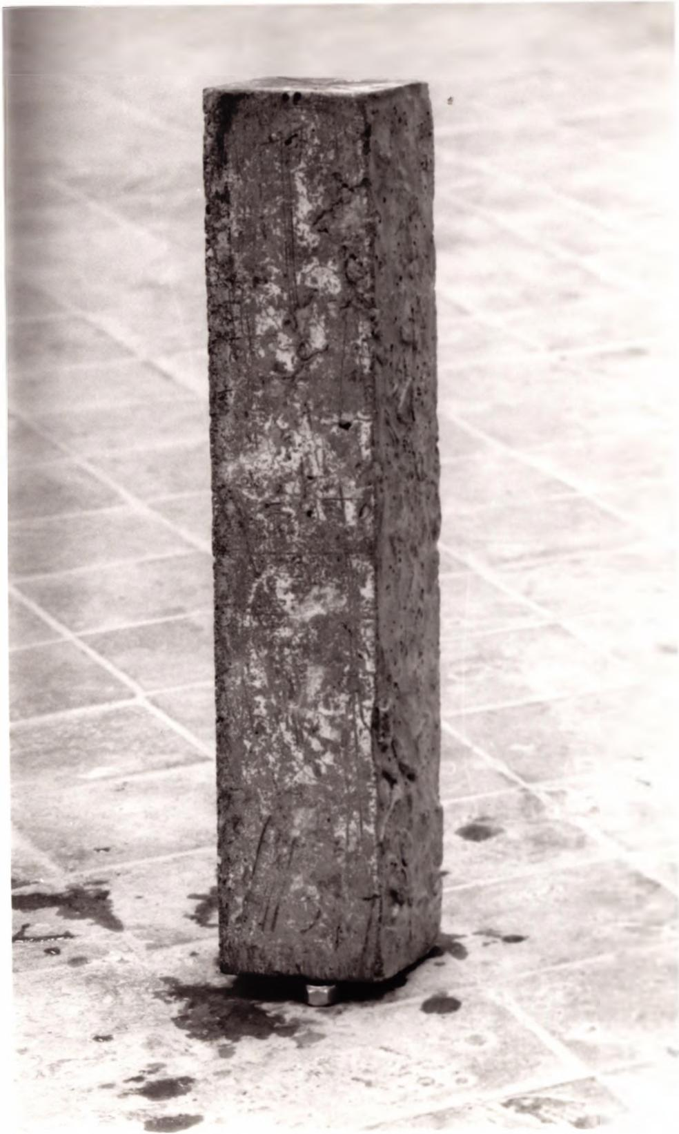
Figure 8.4. A specimen of concrete with sandlime brick aggregate after 50 cycles of sulphate resistance test.
