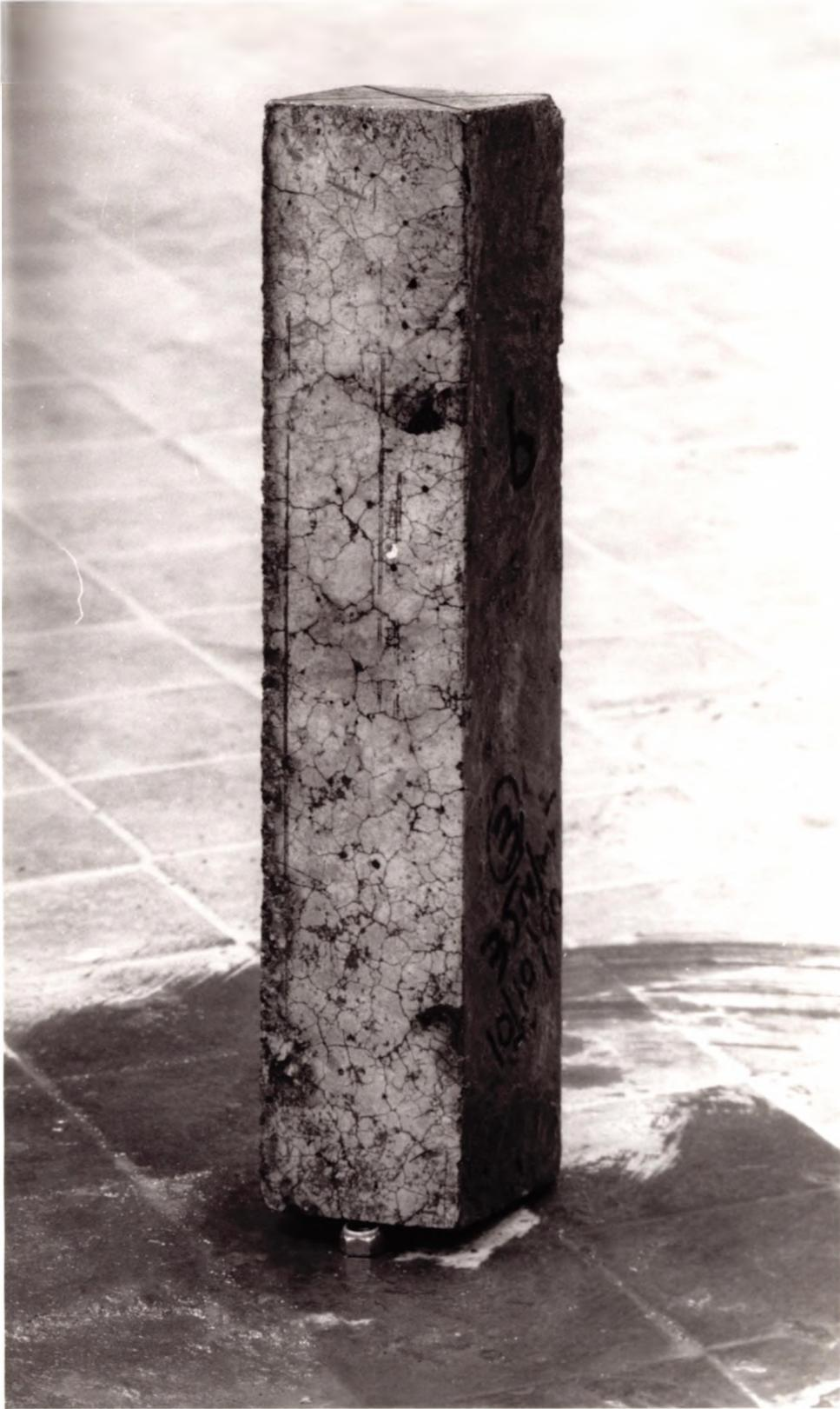
Figure 8.5. A specimen of concrete with engineering brick aggregate after 50 cycles of sulphate resistance test.
