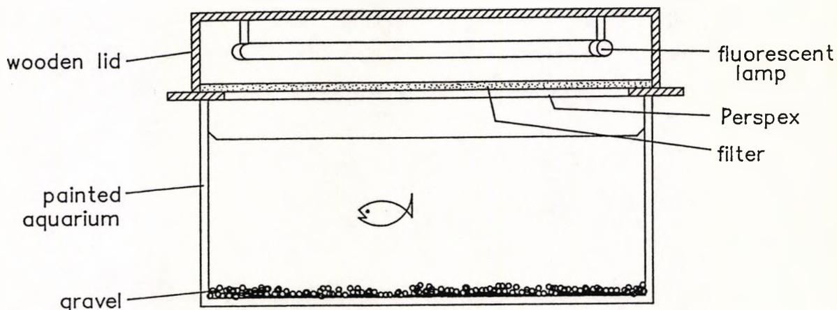
Figure 5-1. Diagram of the experimental tanks used in the lighting experiments. The lid of the high light tank contained two fluorescent lamps with no filter. The low light tank had just one fluorescent lamp and a total of 3.0 log unit neutral density filters. The UV tank lid had two UV tubes with no filter and 2mm thick glass in place of the Perspex.
