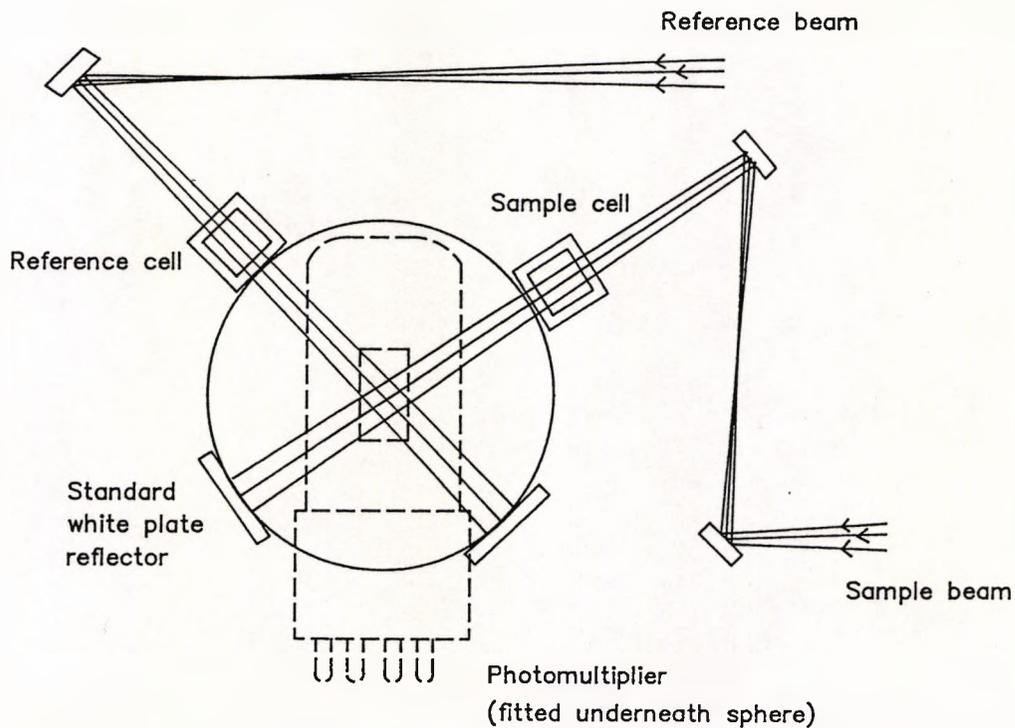
Figure 2-2. Optics of the Shimadzu UV240 integrating sphere.
