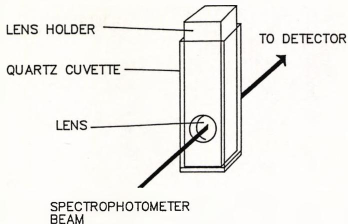
Figure 2-1. Diagram of lens positioned in metal holder within a quartz 1cm pathlength cuvette. The lens is held in position in the path of the spectrophotometer beam.
