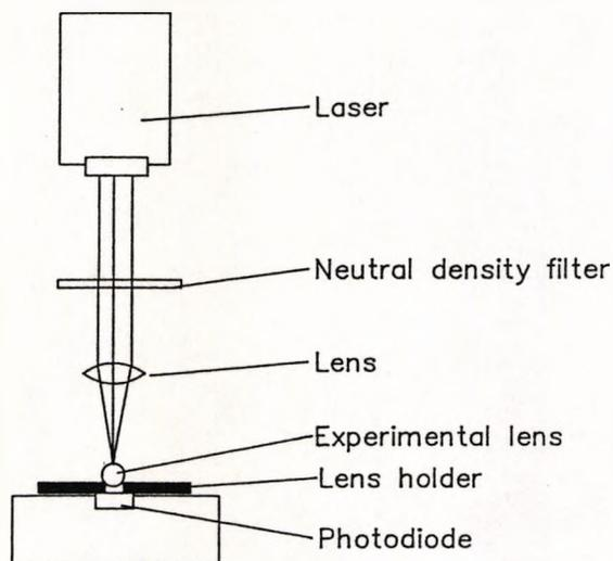
Figure 2-6. Diagram of the apparatus used to measure the absolute transmission of a lens at  $632.8\text{nm}$ . The laser beam was focused onto the experimental fish lens and light transmitted passed to a photodiode where it was converted into a voltage reading.
