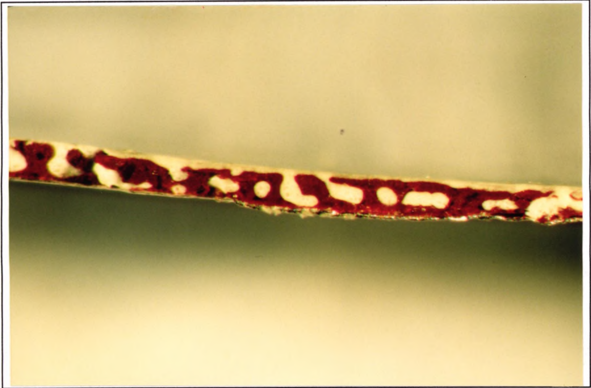
Figure 24 - Epikote 828 / Iron Oxide / Lumiflon LF200 / AMEO coated \text{TiO}_2
