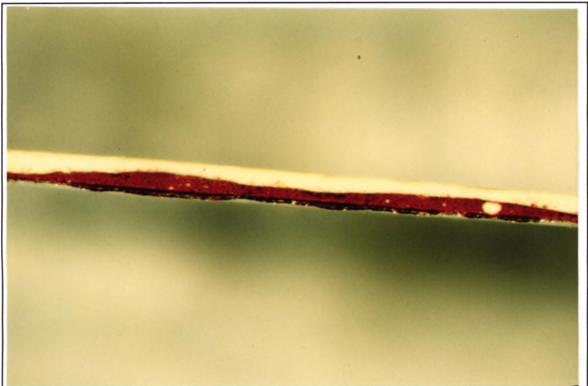
Figure 25 - Epikote 1001 / Iron Oxide / Lumiflon LF200 / AMEO coated \text{TiO}_2
